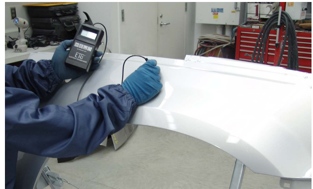
Inspect a recycled part for excessive film build by using a film thickness gauge on various spots.
