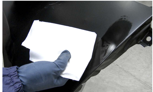
To test for E-coat, rub the surface with a solvent-soaked cloth and look for coating transfer to the cloth or softening of the coating.
