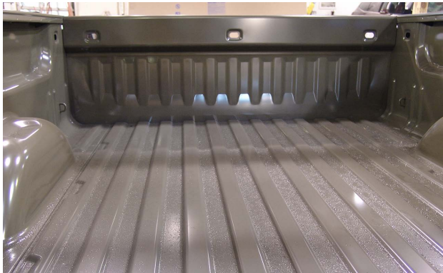
The olive-drab color on this GM pickup bed is electrodeposition coating, or E-coat.
