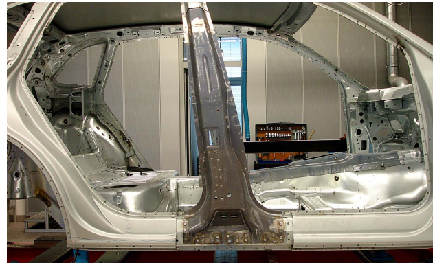
One of the variations of corrosion treatment is how boron-alloyed steel is protected. Audi uses an aluminum / silicon coating, such as on this Q5.
