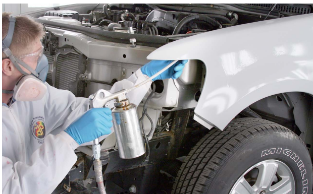
The interior of a replaced upper rail is one location for anti-corrosion compound.
