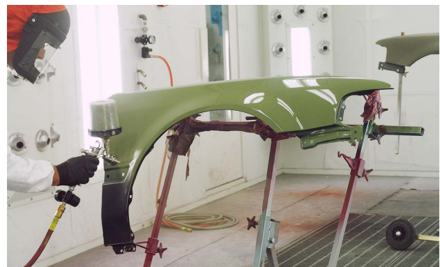
Epoxy primer is commonly applied with a spray gun on large surfaces such as this fender.
