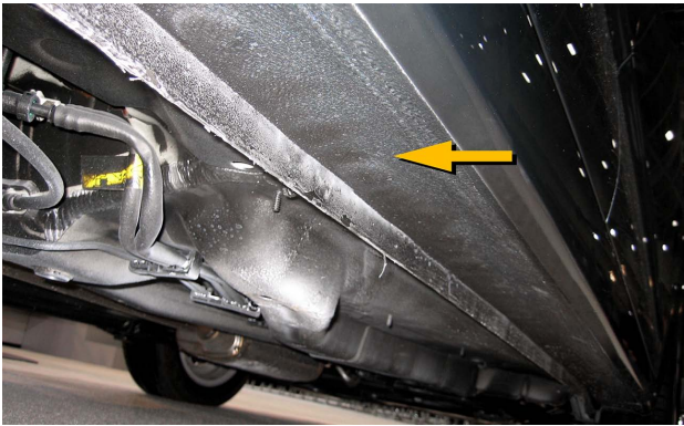
Textured chip-resistant coatings are most common on the lower part of the rocker panel.
