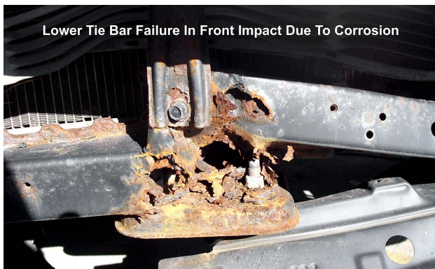
Not addressing corrosion protection during repairs can lead to failure of the structure, like on this lower tie bar.
