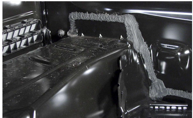
Seam sealers, like this sprayed bead on the inner rear body panel, are typically applied by robots.
