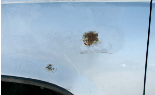
The exposed metal in this one spot is a classic example of a corrosion hot spot, where corrosion forms faster than other areas not exposed.
