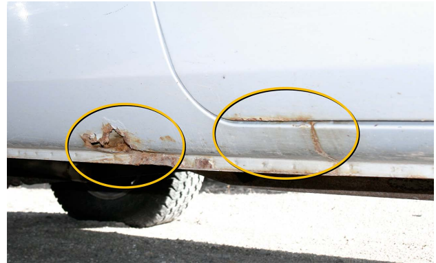
Lower hem flanges and pinchwelds are often traps for collecting water and will corrode from the inside if the backside surfaces are not treated during or after repairs.
