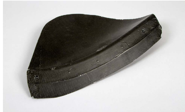
A composite caul plate must be strong enough to compress the repair plies.
