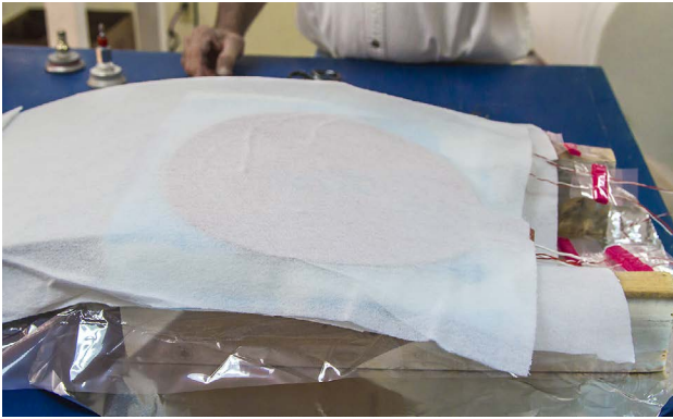
A breather cloth should cover nearly the entire vacuum bagging surface area.
