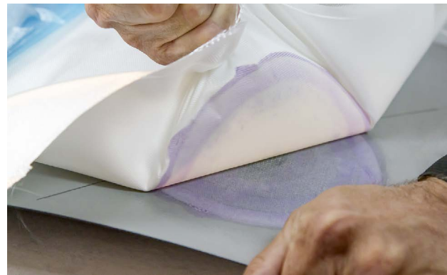
Peel ply and release film are materials that will not fuse with the repair resin.
