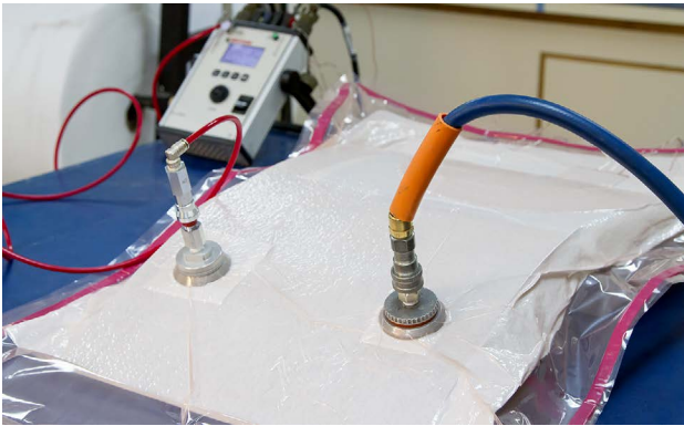
The vacuum port base plate must be placed under the bagging material before it is sealed.
