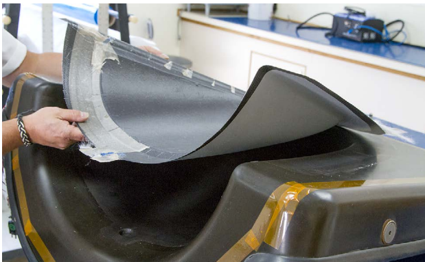
Molds can create a smooth exterior finish.
