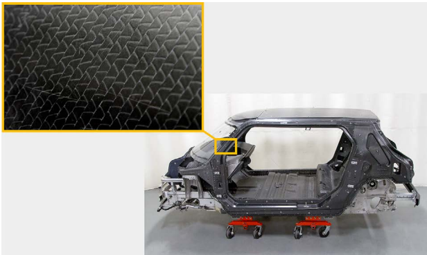
This BMW i3 has exterior panels and a passenger cell made from carbon fiber.
