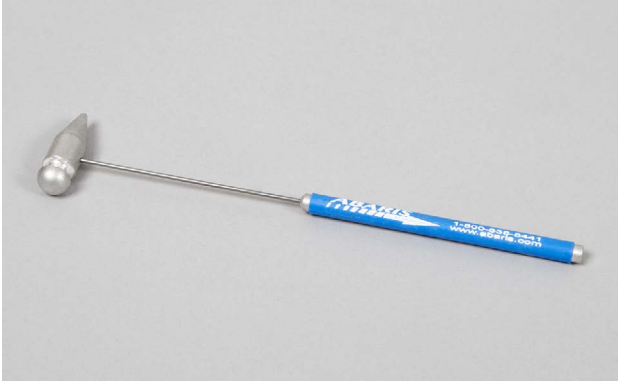
Tap testing allows the technician to hear where the damage is located.
