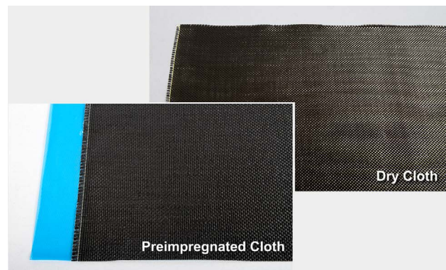
Dry cloth is used for both the wet-layup process and the resin infusion process.
