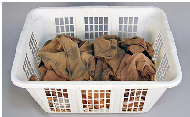
Do not store used shop towels with other materials.
