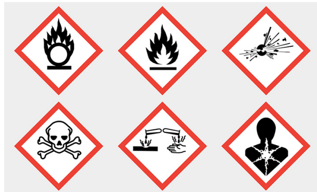
These symbols represent material waste that has ignitable, corrosive, reactive, and / or toxic hazardous material characteristics.
