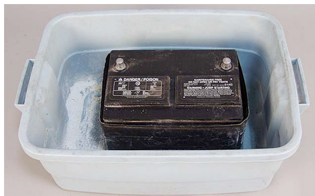
Store used lead-acid batteries separately from other wastes.
