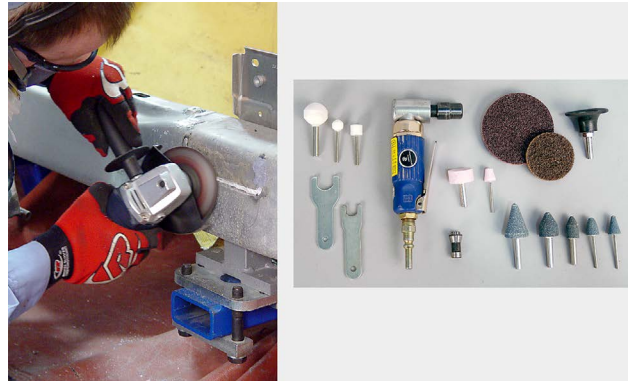
Electric grinders work well for grinding welds (left). Some grinders will have many different attachments (right).
