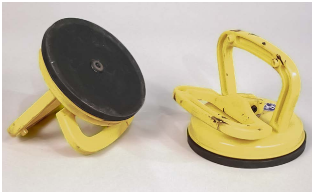
Suction cups are used to lift glass.
