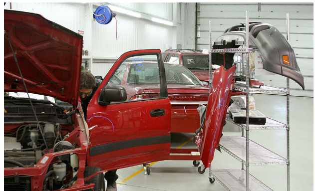
Before the vehicle starts the repair process in this facility, it is disassembled and undamaged parts are properly stored.
