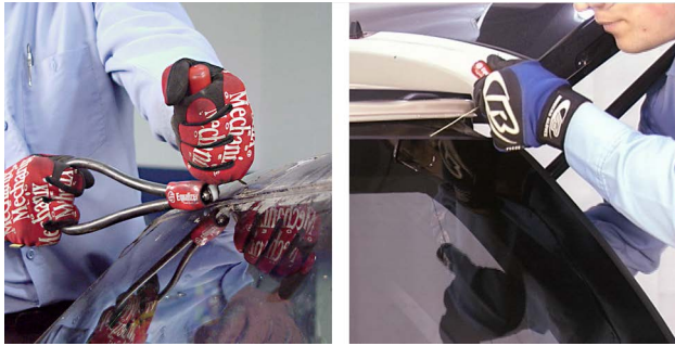
A cold knife is typically pulled through the adhesive (left). Some wire cutting tools are manually pulled through the adhesive (right).
