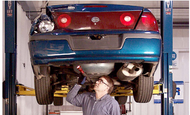
The damage appraiser has this vehicle raised on a lift to inspect the underbody for damage.
