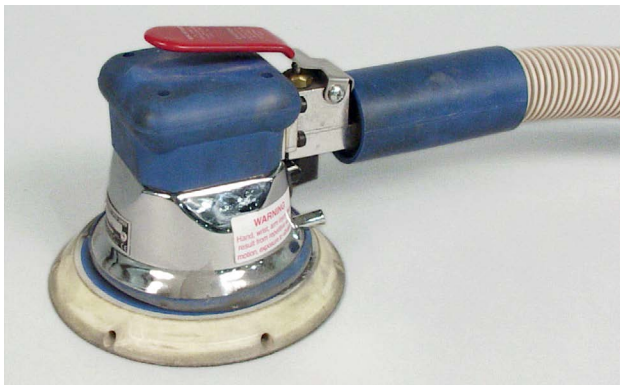
A dual-action sander can be used to remove painted pinstripes.
