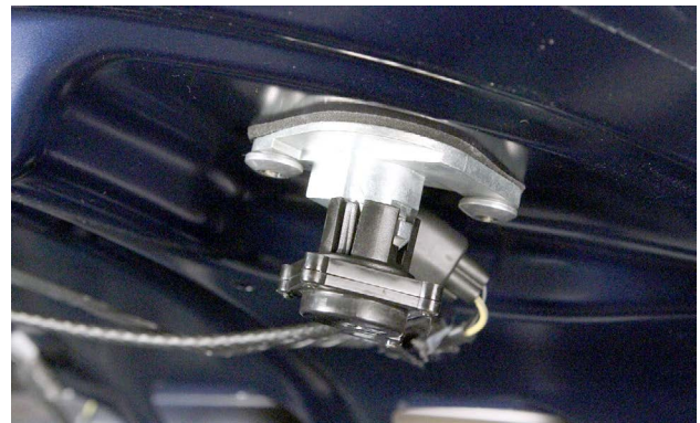
This door lock cylinder assembly is attached to the decklid with rivets.
