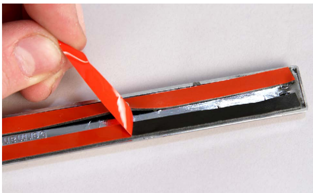
Two-sided tape is applied to the backside of this molding.
