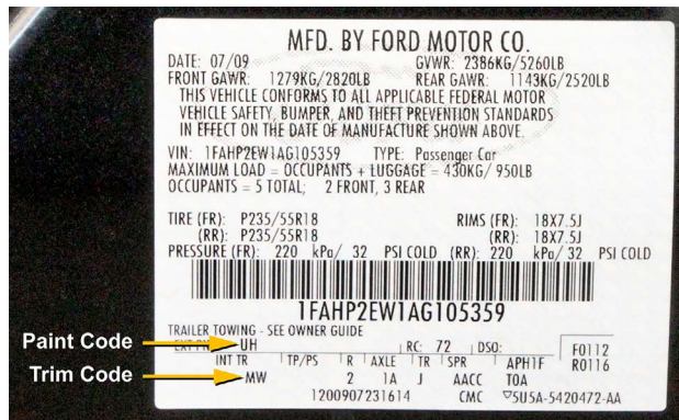
Paint and trim codes are included on this label.
