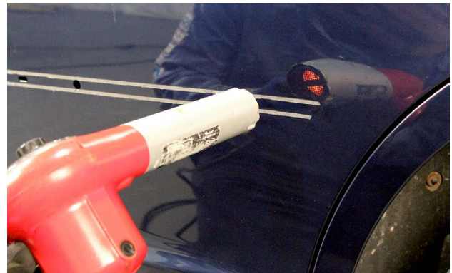
Heat is being applied to the adhesive residue on the panel surface.
