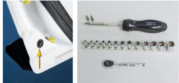
This screw attaches to the bodyside molding (left). Fasteners can be removed and replaced using basic hand tools (right).
