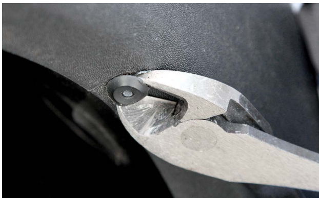
A side cutter is being used to remove this plastic rivet.
