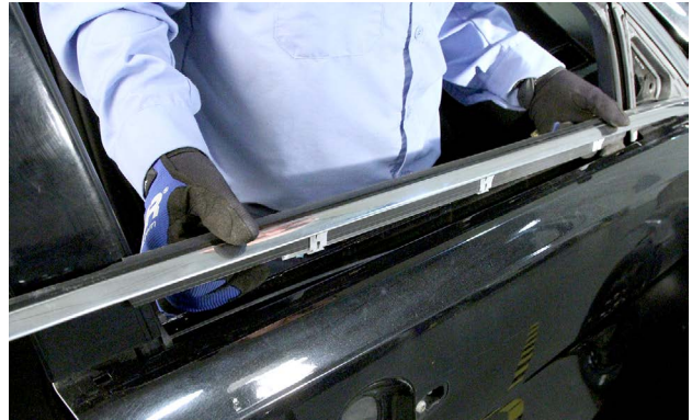
The belt-line molding runs from the front of the front door to the rear of the rear door.
