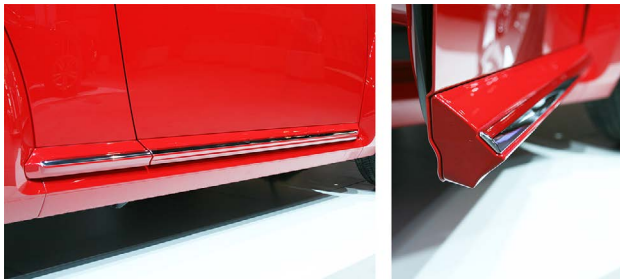
This bodyside molding has two pieces (left). The thickness of the molding can be seen on the edge of the part (right).
