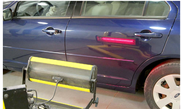
A heat lamp is being used to loosen the molding adhesive.
