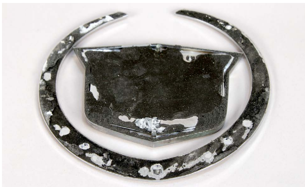
This emblem was attached with adhesive.
