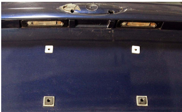
License plate screws fasten through the license plate and into these nylon retainers.
