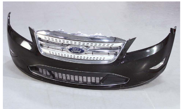
This grille assembly is attached to the bumper cover.
