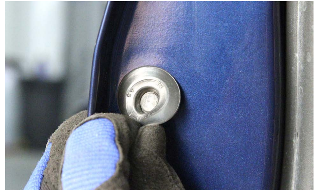
This grommet is being removed from the door shell to access a door handle fastener.
