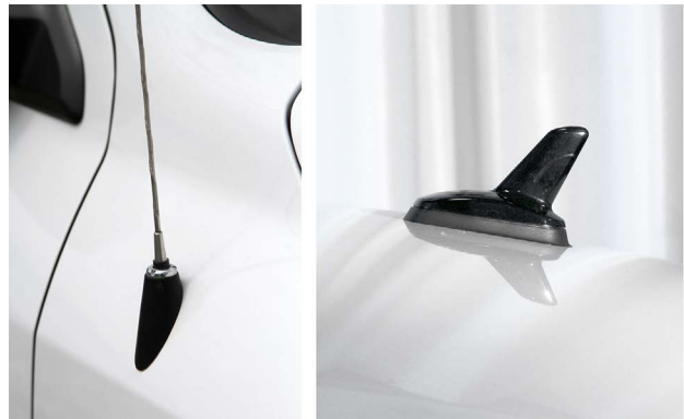
A radio antenna is mounted to the fender (left). This antenna is attached to the roof (right).
