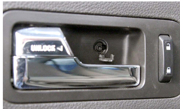
A screw for removing the door handle trim is shown.
