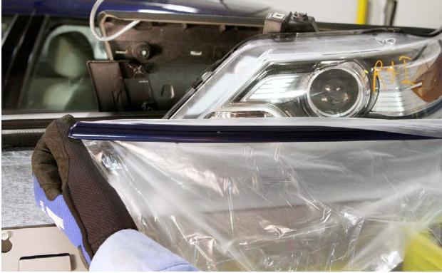
This molding is being wrapped in plastic to protect the backside from dust.
