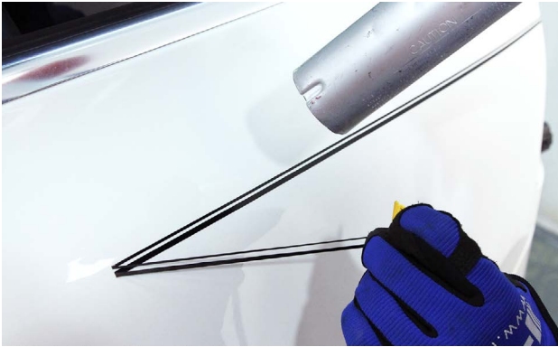
Heat is applied to the taped pinstripe as it is being removed.
