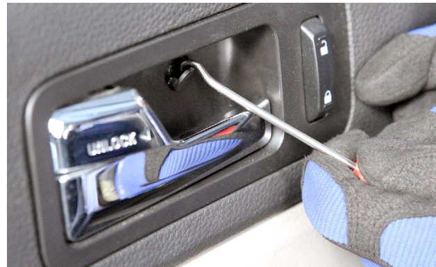
A plastic cover in the door handle trim is being removed.
