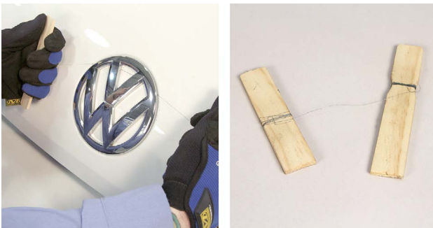
Fishing line can be used to cut the adhesive in recessed areas (left). Two pieces of a wooden paint stir stick are used as makeshift handles for the fishing line (right).
