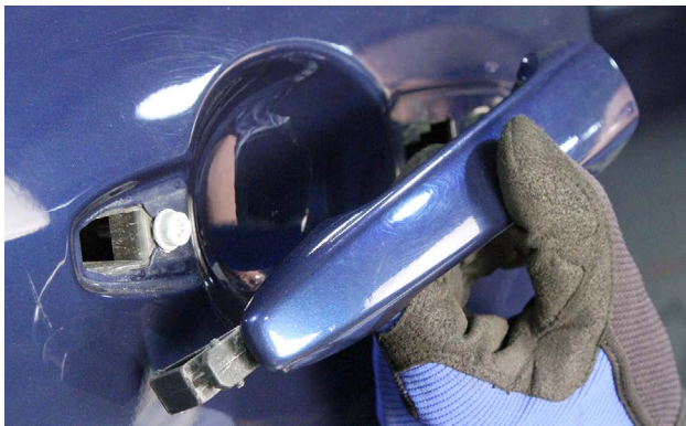
The door handle is being removed.
