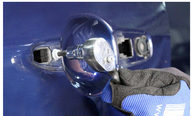
A door handle fastener is being removed.
