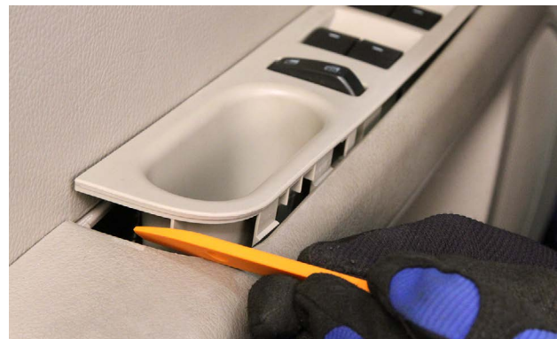
The power accessory switch panel is being removed.
