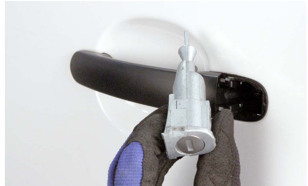
This door lock cylinder has been removed from the door handle assembly.
