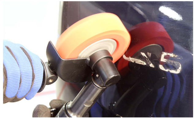
An eraser disc is being used to remove the remaining adhesive from the panel.
