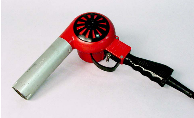
A heat gun may be used to soften the adhesive during removal.
