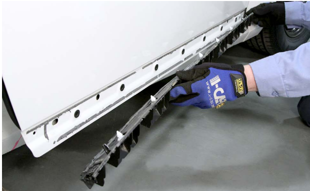
A part of this bodyside molding is attached with clips.
