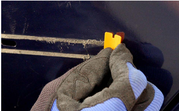
A plastic razor blade is being used to scrape the adhesive residue off the panel.
