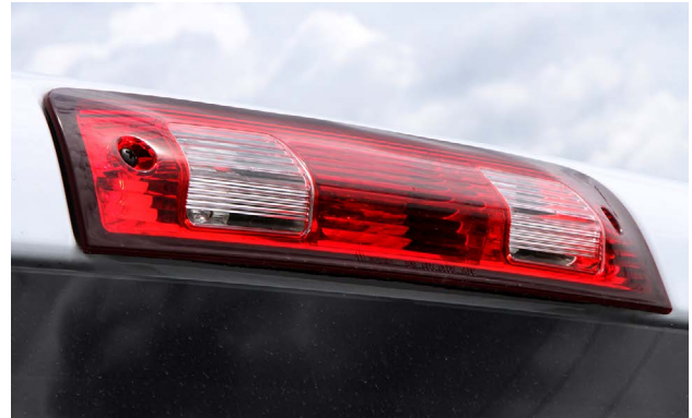
Screws and a moisture seal are used to attach this high-mount stop lamp to the roof panel.
