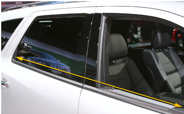
The belt-line molding runs from the front of the front door to the rear of the rear door.
