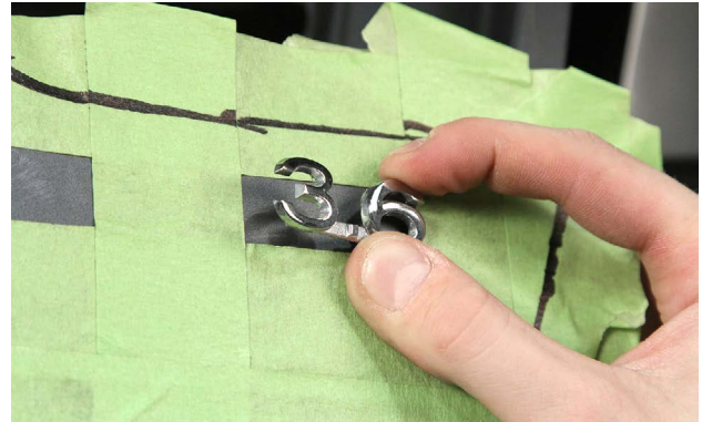
A pre-made template is being used to properly position the nameplate on the vehicle.
