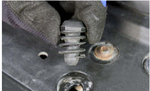
This stopper can be adjusted to align the hood to the fenders.
