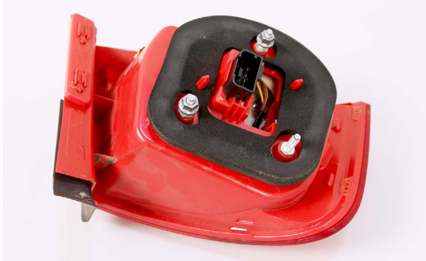
This tail lamp assembly is attached with hex nuts.
