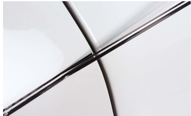
To help with alignment, the replacement pinstripe is temporarily applied to overlap the original pinstripe on an adjacent panel.
