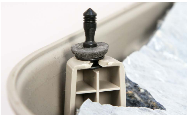
This fastener remains attached to the door trim panel.
