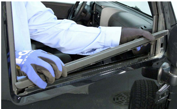
This belt-line molding is being removed.
