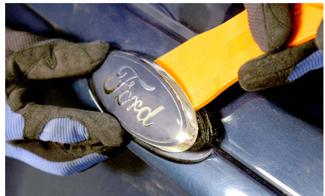
The emblem is being removed with a plastic trim removal tool.
