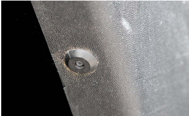
This plastic rivet attaches the wheelhouse flaring to the vehicle.
