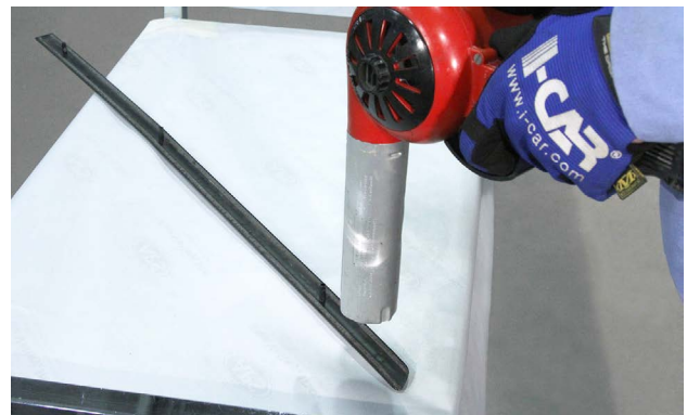
Heat is being applied to the backside of this molding to loosen the adhesive.
