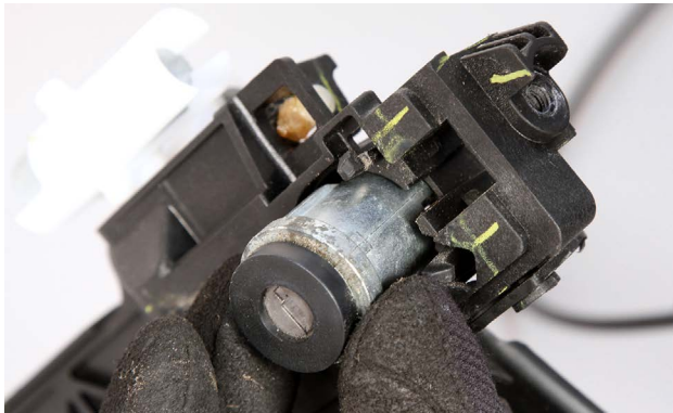
This door lock cylinder is being removed from the assembly.
