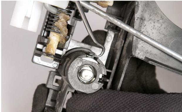
A retaining clip is being removed from this door lock cylinder.
