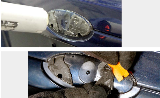
Heat is being applied to this panel to remove the adhesive (top). A plastic razor blade is being used to remove the heated adhesive from this panel (bottom).
