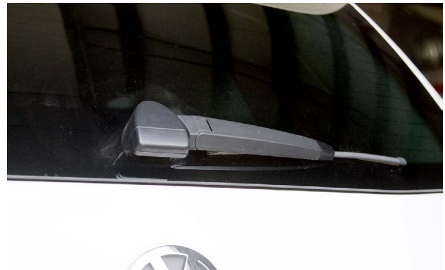
A rear windshield wiper is attached to this liftgate glass.
