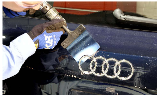
An air chisel attachment and lubricant are being used to cut the emblem adhesive.
