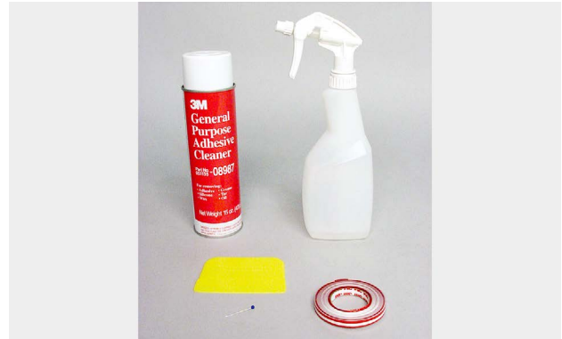
Tools and products needed to apply a taped pinstripe include water-based and oil-based cleaners, a squeegee, a pin, and the pinstriping tape.
