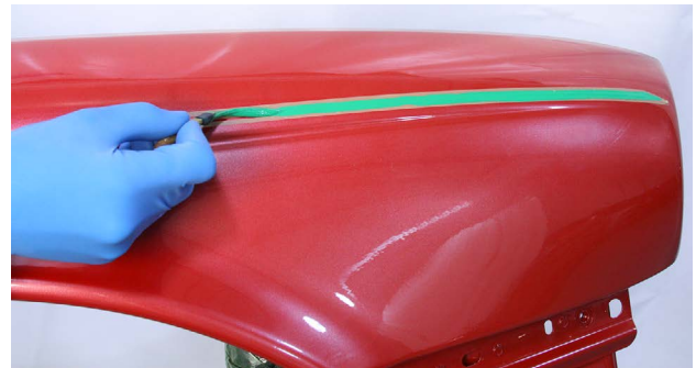
Pinstriping may be done using fine-line tape as a guide.
