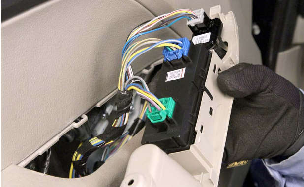
Various connectors for the power accessory switch panel will have to be removed.
