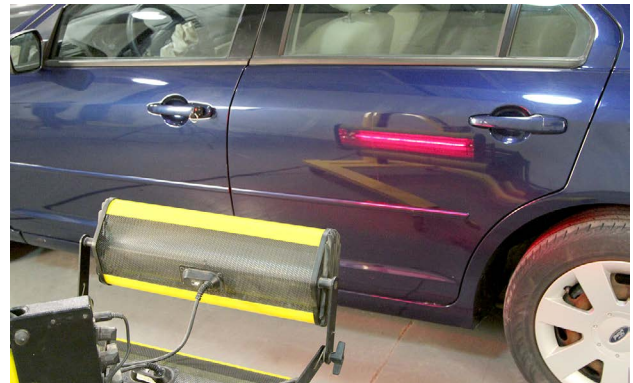
A heat lamp is being used to loosen the adhesive of this emblem.
