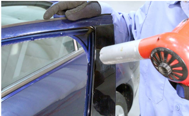
Heat is being applied to this adhered appliqué.
