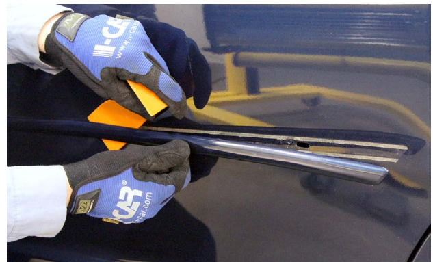
The molding is being carefully pried away from the panel.
