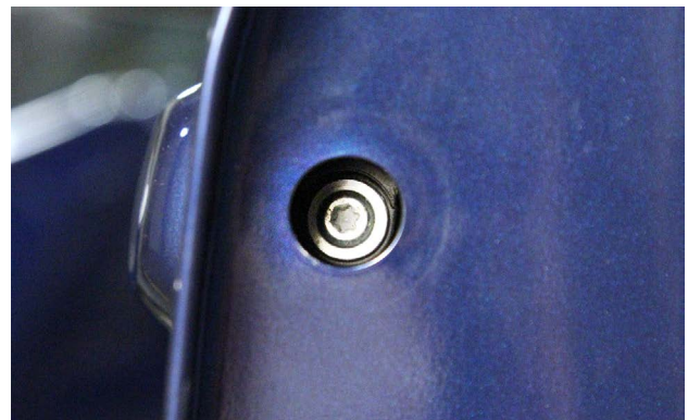
A fastener for the door handle is shown.
