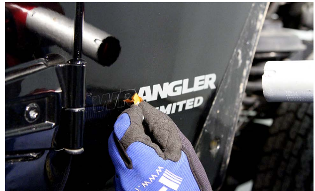
This decal is being removed with a heat gun and plastic razor blade.
