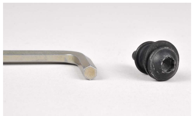
An allen wrench is used with fasteners that have an allen head.
