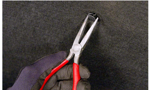
A needle nose pliers is being used to remove this nylon retainer.
