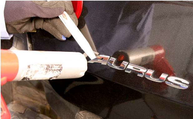
A heat gun and plastic tool is being used to remove the letters of this nameplate.
