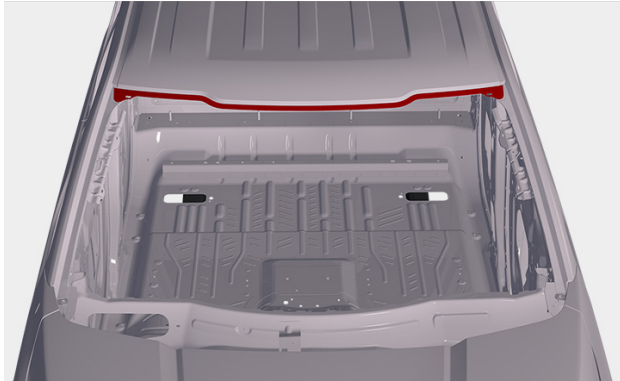
Rivet bonding is used along the front edge of the roof.
