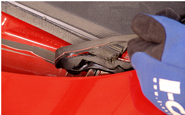
When trimming the existing adhesive bed, do not cut down to the bare metal.
