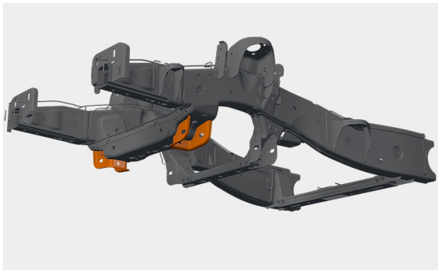
Front control arm brackets are a service part on the 2015 F-150.
