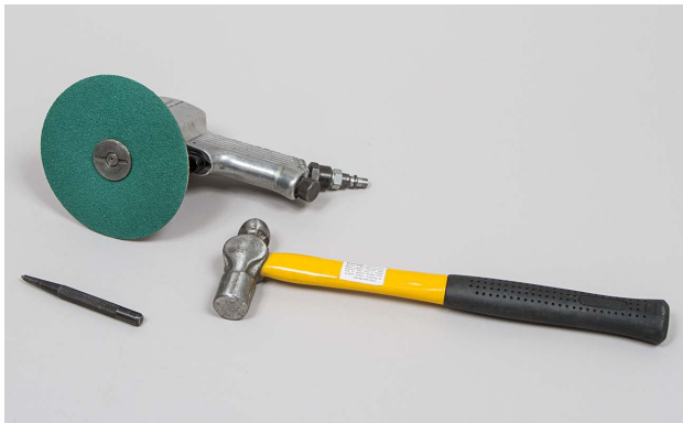
These are some tools that are used for removing rivets.
