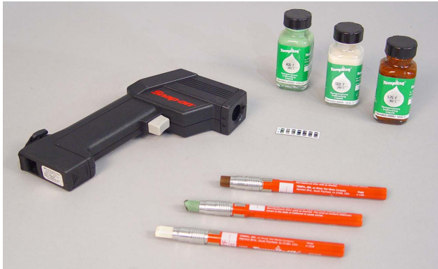
Thermal paint, thermal stickers, temperature crayons, and a noncontact thermometer are used to monitor heat.
