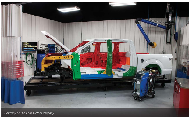
Courtesy of The Ford Motor Company Dedicated aluminum repair areas are designed to protect an aluminum vehicle during repairs.
