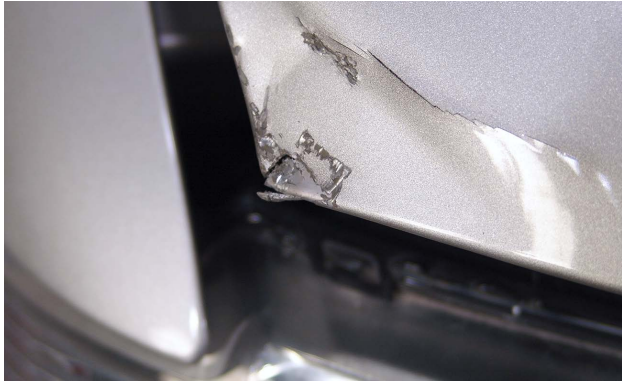
Creases or tears in a panel generally requires panel replacement.
