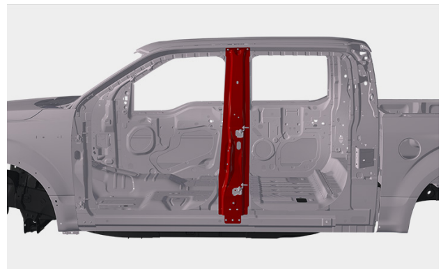
The replacement B-pillar reinforcement is attached with rivets and adhesive.
