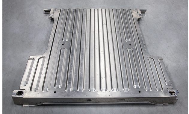
This bed floor is an aluminum stamped sheet.
