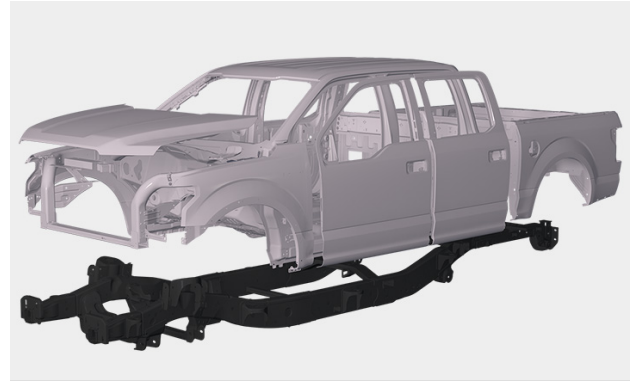
The aluminum outer body panels on the 2015 F-150 have different repair considerations than steel models.
