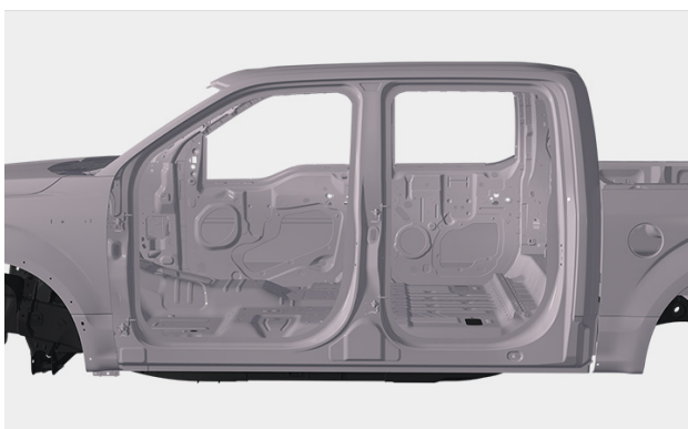
To gain access to the B-pillar reinforcement, at least a portion of the outer body side panel must be removed.
