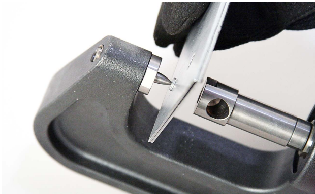
Some riveting tools have special dies for removing an SPR.
