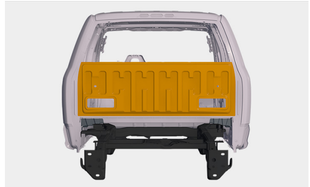
The rear cab panel is able to be replaced without damaging adjacent panels.
