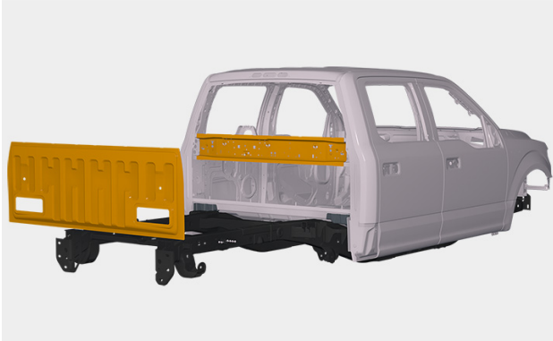
The rear cab panel is rivet bonded to the cab.
