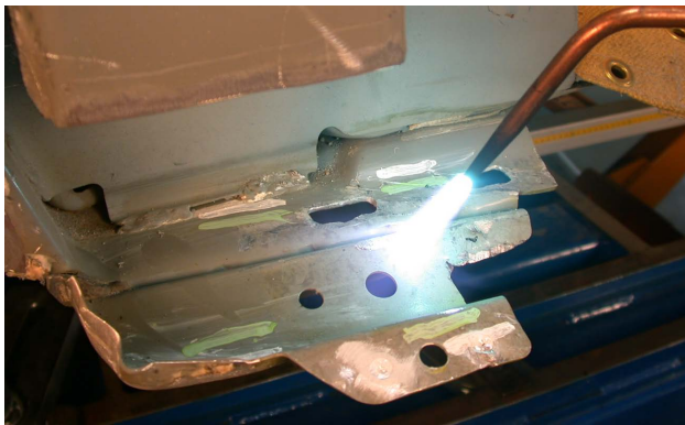
Heat-monitoring paint is used when heating aluminum.
