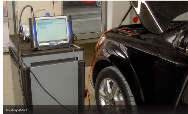
Vehicle maker-specific scan tools may be required to calibrate the system after repairs.
