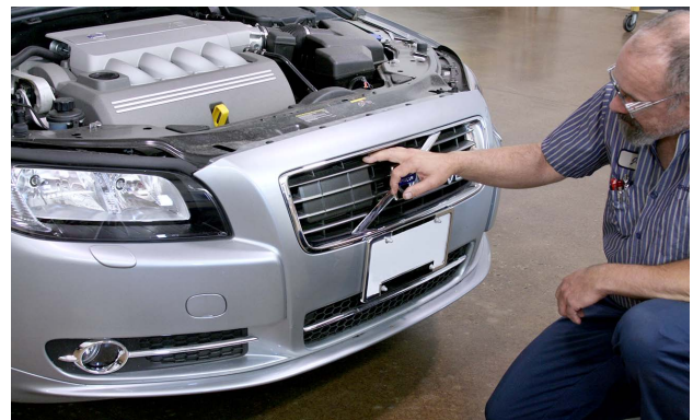
The pre-collision sensor on this vehicle is located behind the front grille, and is susceptible to light or moderate collision damage.
