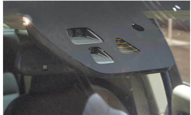
The City Safety system uses a laser sensor module that is mounted next to the rearview mirror.
