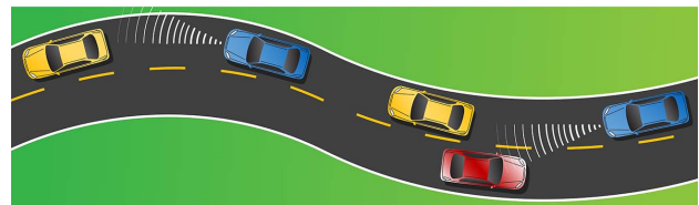
Dirty sensors or curvy roads can prevent proper operation of an ACC system.
