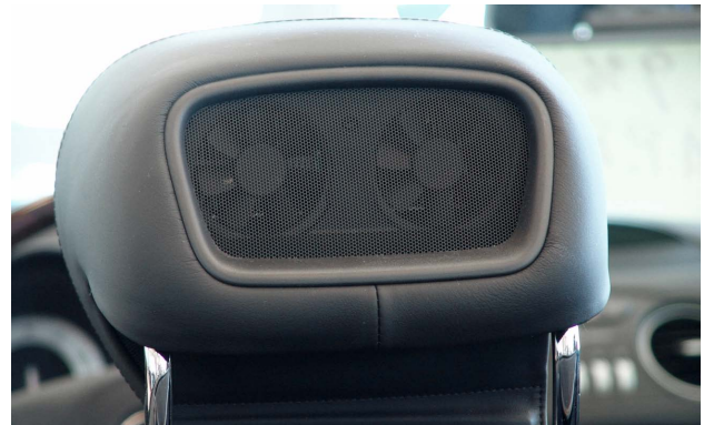
Blower vents for the Airscarf system can be seen from the backside of the head restraint.
