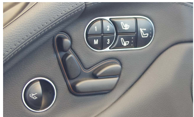
Switches for the climate-controlled seat and Airscarf system are located on the interior door trim panel.
