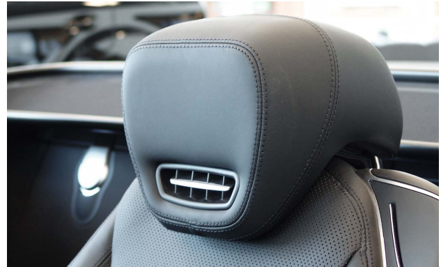
Mercedes-Benz has a seat comfort system called Airscarf that blows warm air through the head restraint.
