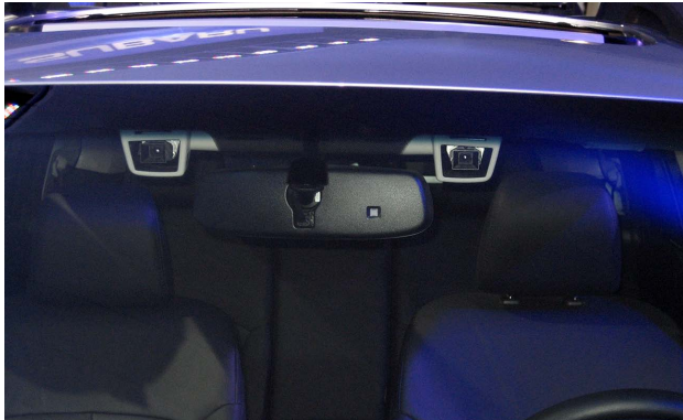
Two cameras straddling the rearview mirror keep an eye to the front with Subaru's Eyesight Driver Assistance system.
