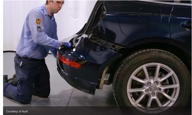
Part removal may be required to determine if a sensor has collision damage.
