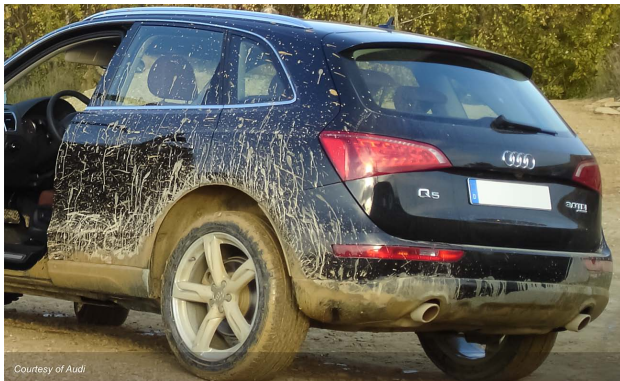
Mud buildup on the rear bumper cover can interfere with a blind spot detection system.
