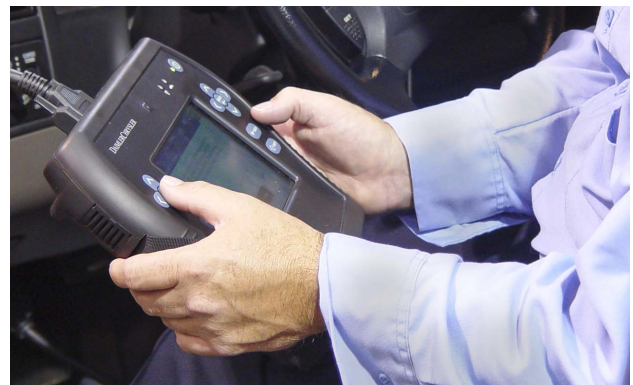
Scan tools are generally required for performing diagnostics on advanced vehicle systems.
