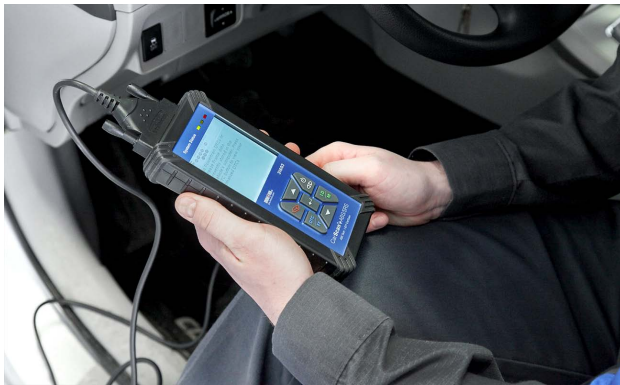
A scan tool is used to diagnose the parking assist system.
