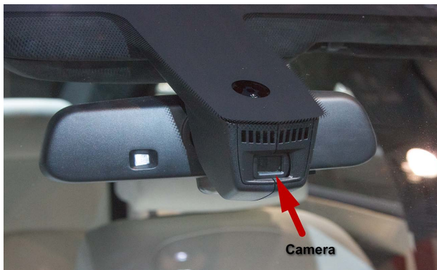
The camera for the high beam assist system on this vehicle is mounted by the interior rearview mirror.
