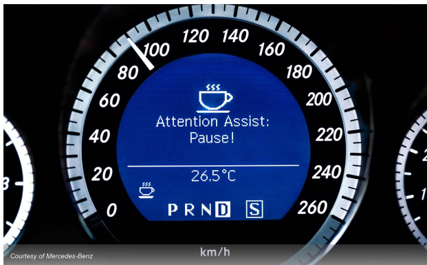
The message displayed in the driver information center is recommending that it is time for the driver to take a break.
