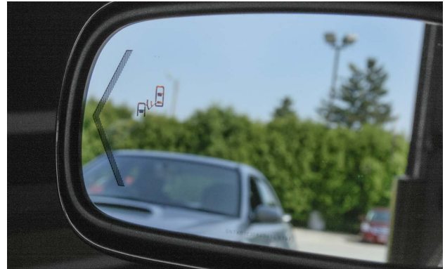
This type of icon on the door mirrors is an indication that the vehicle is equipped with a blind spot detection system.
