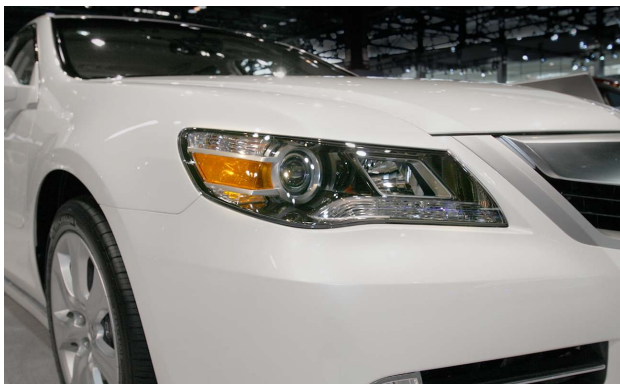
The rotation of the headlamp is controlled by the steering wheel angle sensor.
