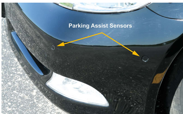
The parking assist sensors are used by the system to judge the distance to other vehicles.
