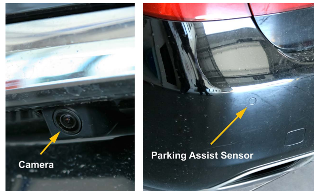
The camera and sensors are integral parts of the hands-free parallel parking assist system.
