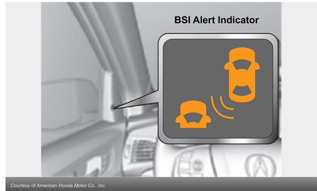
The indicator lamp turns on or flashes when a vehicle is in the blind spot area.
