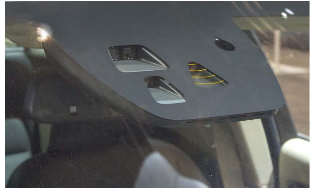
The attention assist system uses the same camera as the lane departure warning system.
