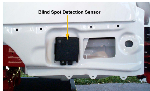
The blind spot detection system on this Ford Fusion has a sensor located behind the rear bumper cover.
