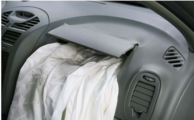
Some passenger airbags use the windshield for proper deployment.
