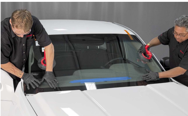
When installing the glass, push down on the bonding areas to help make the seal.
