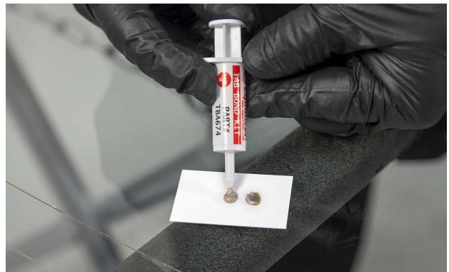
The special kit adhesive, an epoxy, is dispensed in the two parts and mixed.
