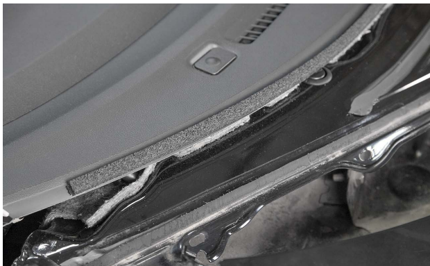
The foam strip on the inside of this pinchweld is from the OEM, and must be kept intact or be replaced during glass replacement.
