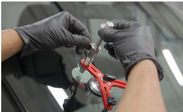
The bullseye is centered under the guide so resin can be inserted.
