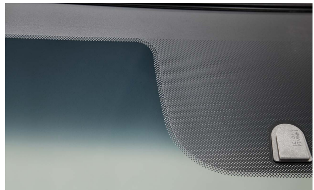
Shading across the top of some windshields is designed to help keep the sun out of the driver's eyes.
