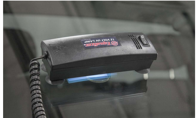
A UV lamp is used to cure the resin.
