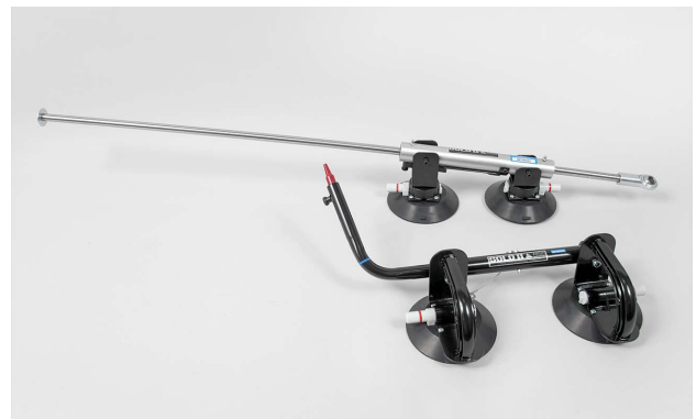
This is another version of a tool allowing a technician to do a solo install of a windshield.
