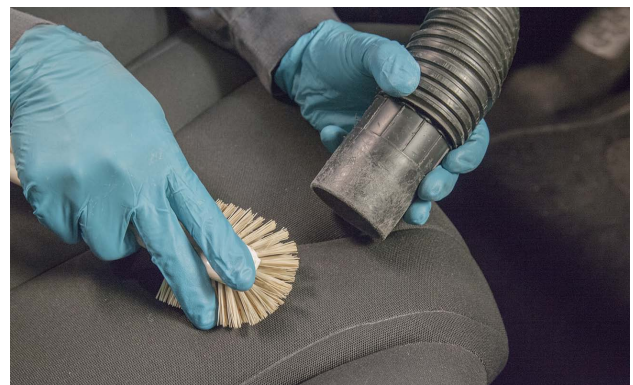
When cleaning the interior, vacuum the seats and use a brush to help pick up slivers from broken laminated glass.
