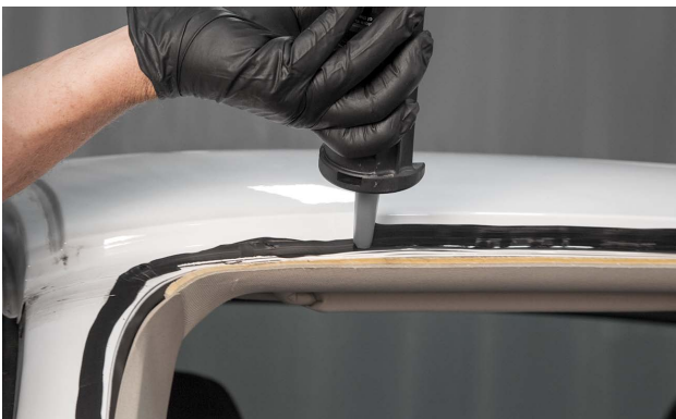
The applicator gun is held straight out so the top of the triangular bead sticks straight up.
