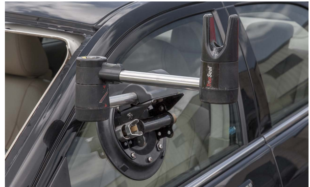
This "Lil Buddy" tool allows one technician to safely remove and install a windshield.
