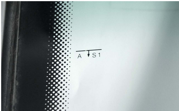
The AS1 code indicates a laminated glass windshield, with the proper light transmittance below the arrow.
