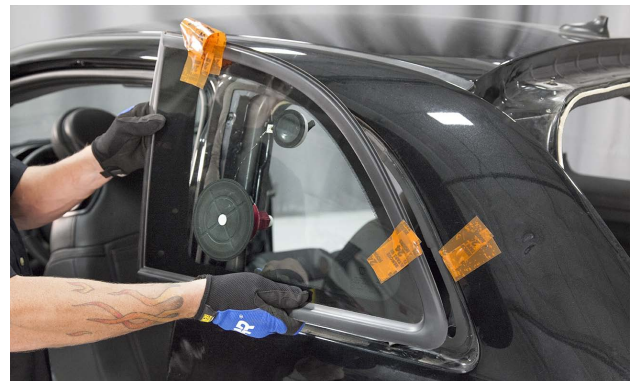
The side glass has just been cut out with the wire tool and is being removed from the opening.
