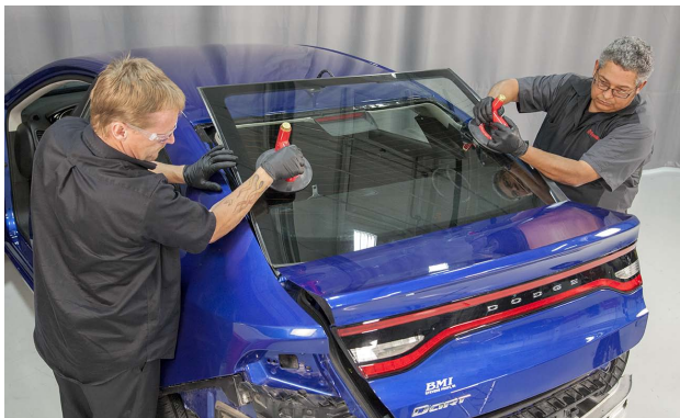
The backglass is being carefully installed in the glass opening.
