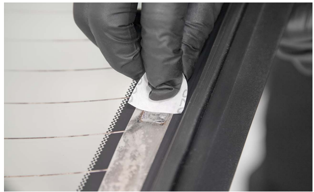
Sand the mounting area and the base for the terminal tab.
