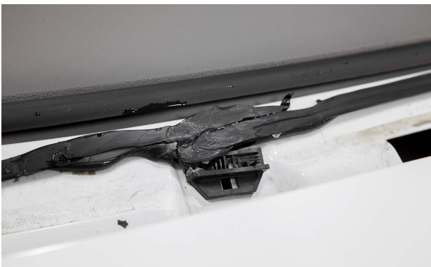
Setting blocks are handy for setting the windshield on when installing.
