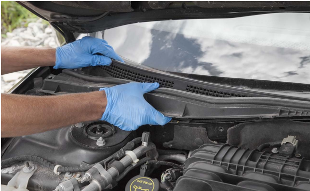
The cowl trim panel typically must be removed when replacing a windshield.
