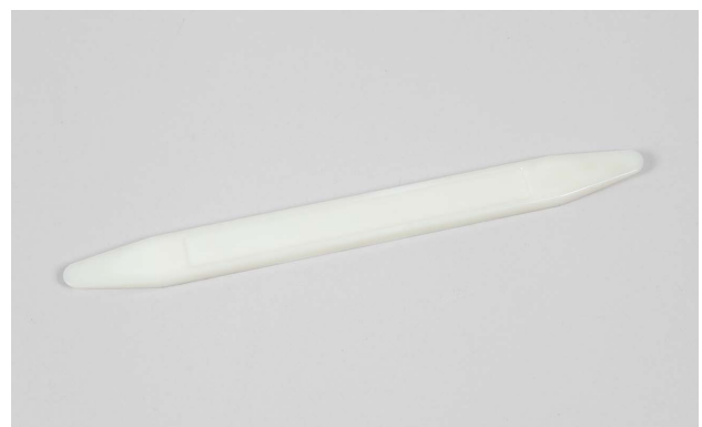
This plastic stick is for paddling the urethane after it is applied.
