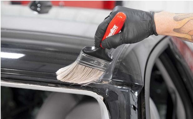
Brush off contaminants from the pinchweld before trimming the urethane down.
