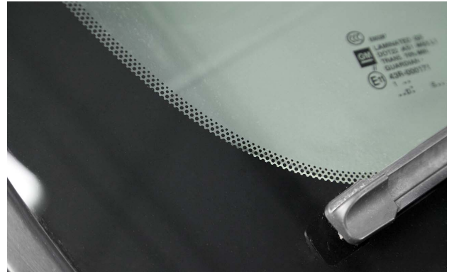
The frit is designed primarily to protect the urethane adhesive from deteriorating due to UV ray exposure.
