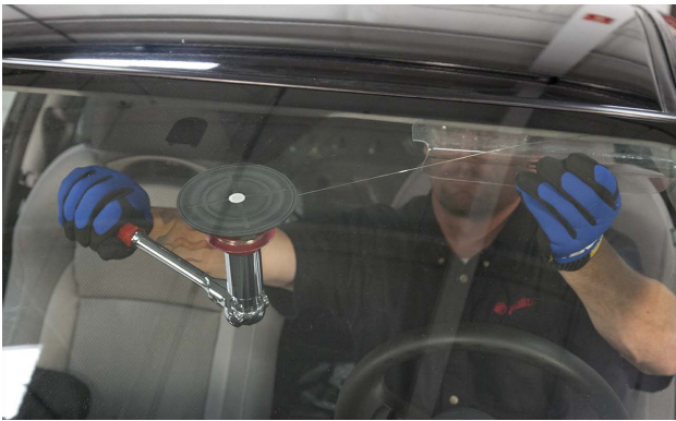
The pulley is ratcheted around to pull in the wire, drawing the wire around the perimeter of the glass while cutting through the urethane.
