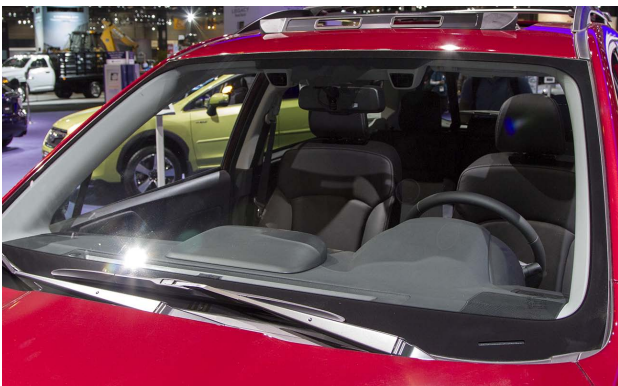
This windshield, bonded with urethane adhesive, contributes to the structural strength of the vehicle.
