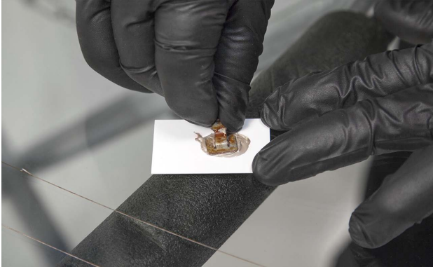
The base of the terminal is coated with the adhesive.
