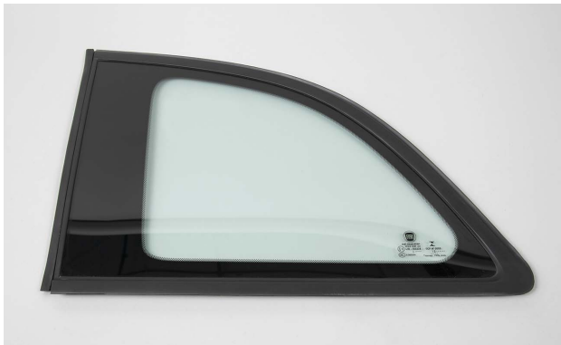
The molding on the edge of this quarter glass is a permanent part of the glass, formed onto the glass when the glass was made.
