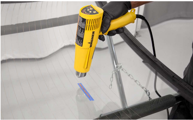
A heat gun is used to cure the conductive paint.
