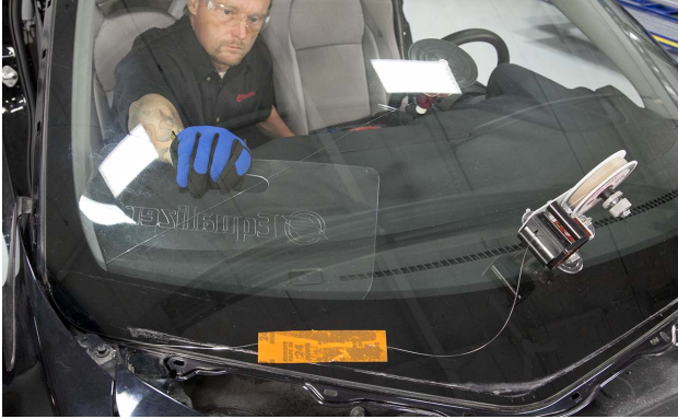
A plastic shield is part of the tool kit for protecting the dash and other parts from damage.
