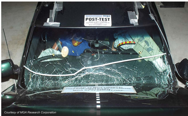
The strong plastic inner layer in a windshield holds the glass together when broken and helps to retain occupants during a collision.
