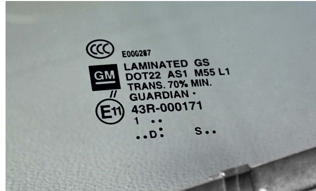
Some of the information for ordering glass can be found in the label on the glass itself.
