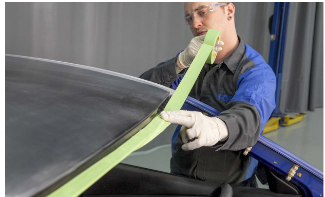
This new pinchweld is being masked before the application of basecoat / clearcoat in order to prevent a possible weak link.
