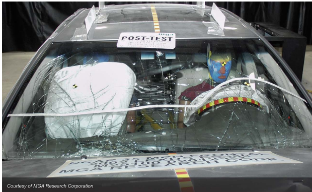
Airbags must properly deploy to meet the FMVSS 208 standard.
