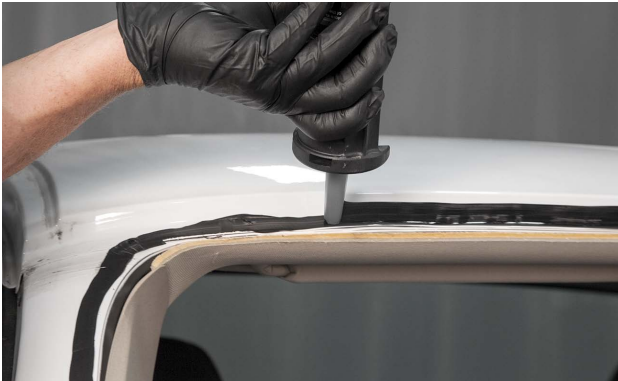
The technician is applying urethane adhesive to the trimmed-off existing bead.
