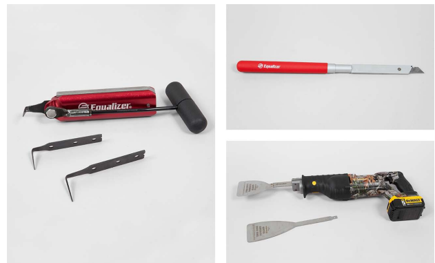
Other removal tools include (clockwise from left) a cold knife, long knife, and power cutters.
