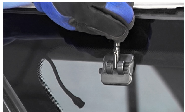
This mount for a telecommunications antenna comes already attached to the glass.
