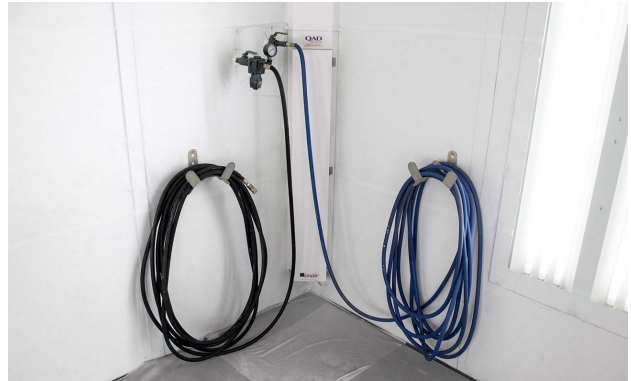
Connect air hose inlets to regulators and shutoff valves inside the spraybooth.
