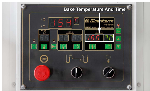
The spraybooth temperature and time left is displayed during the bake cycle.
