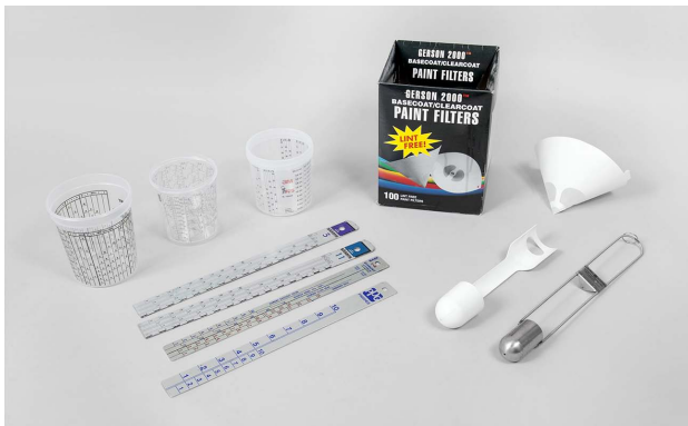
Mixing cups, viscosity cups, paint filters, and mixing sticks are all important tools needed to help create a quality refinish.
