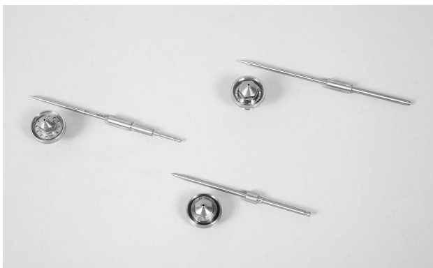
Fluid needles and nozzles come matched.
