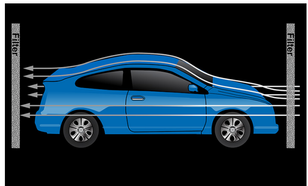
Air flows this direction in a crossdraft spraybooth.
