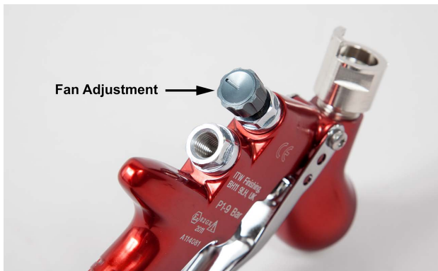
The fan adjustment can be located in different areas depending on the spray gun maker.
