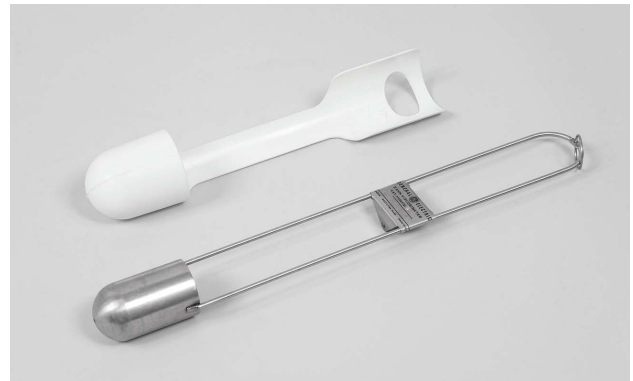
Viscosity cups are used to measure the thickness of the refinish material.
