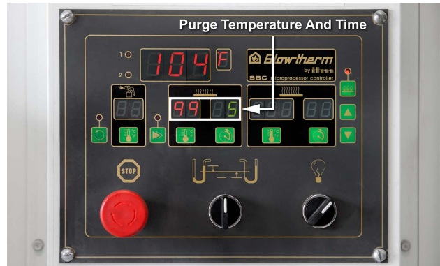
The spraybooth temperature and time left is displayed during the purge cycle.
