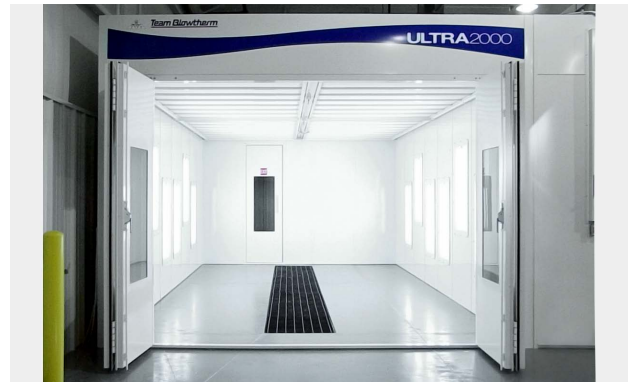
A spraybooth should be clean, bright, and airtight.
