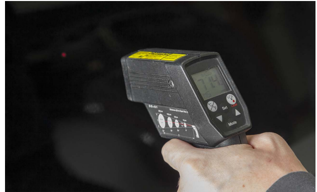
Surface temperature can be measured using a noncontact surface thermometer.
