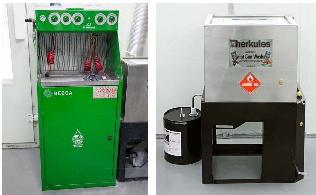
Spray gun washers are used to evacuate solvent fumes and contain cleaning solvent.
