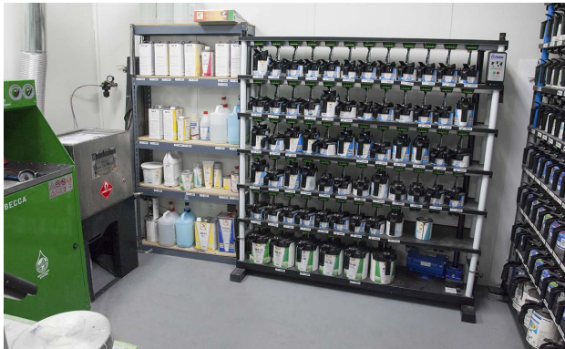
Mixing rooms contain the materials and equipment for preparing refinish materials.
