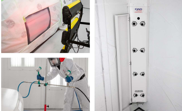
Shown is a portable infrared lamp (top left), hand held multipliers (bottom left), and venturi blowers (right).
