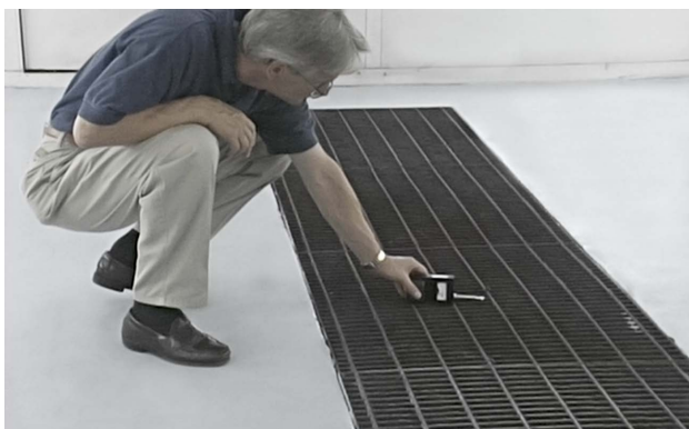
A velometer measures the exchange of air through a spraybooth.
