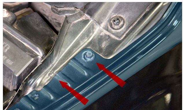
This fender is being adjusted inward, indicated by the finish from under the bolt head.
