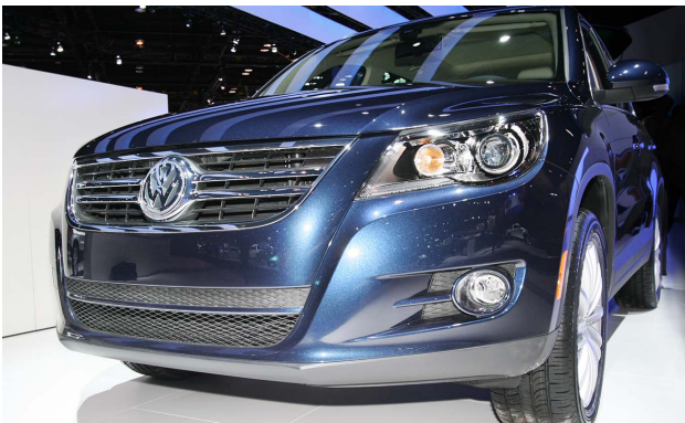
Attachments to a front bumper cover may include an air dam, and lamps.
