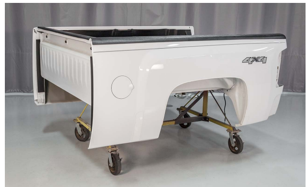
Use a cart or dolly to aid in moving the truck box.
