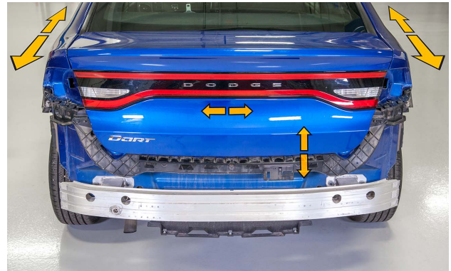
Adjustments on this deck lid include forward and rearward, up and down, and from side-to-side.
