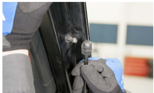
This piston-type prop is installed on the ball stud.
