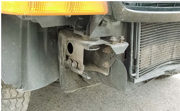
On this body-over-frame vehicle, adjustments are in the form of slotted holes.
