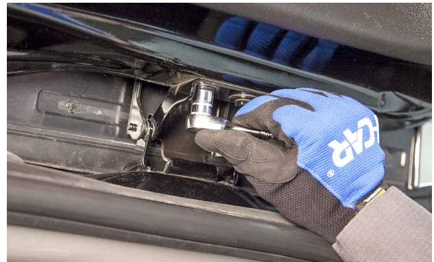
These hinge-to-liftgate fasteners are removed with a socket and ratchet.
