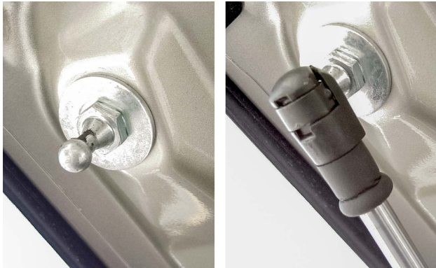
Piston-type prop rods may use a ball stud and a socket with a retainer clip to attach them to the hood.
