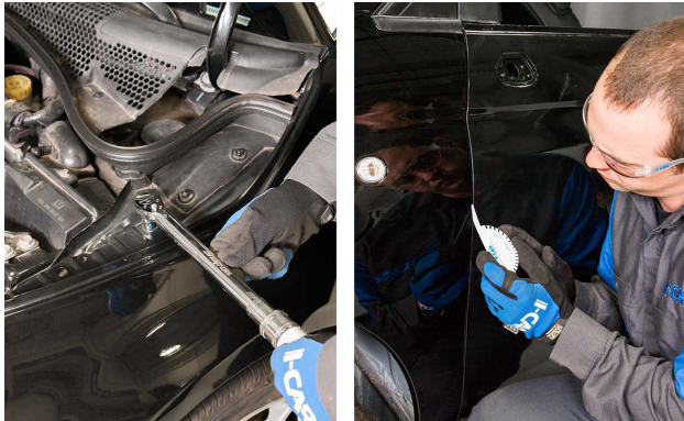
This fender bolt is being tightened to the recommended torque specification (left). The panel gaps are being verified (right).
