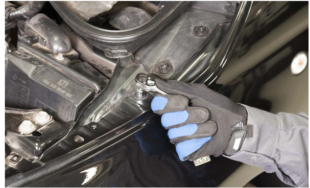
This damaged fender is being removed from this vehicle.
