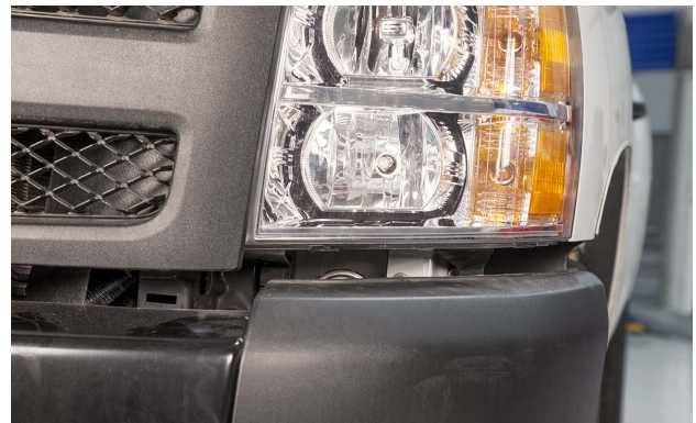
This bumper will have to be adjusted so that the gaps between the lamps and the bumper are consistent from side-to-side.
