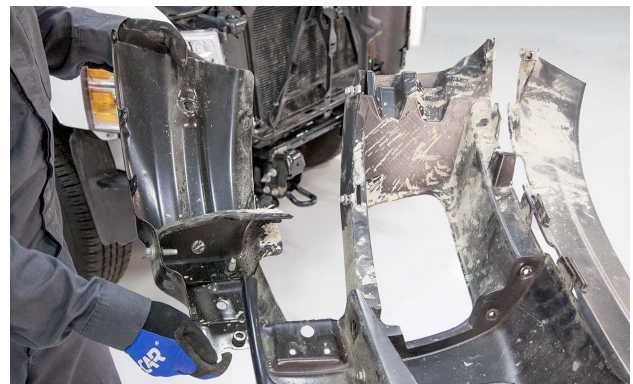
This bracket is being inspected for damage.
