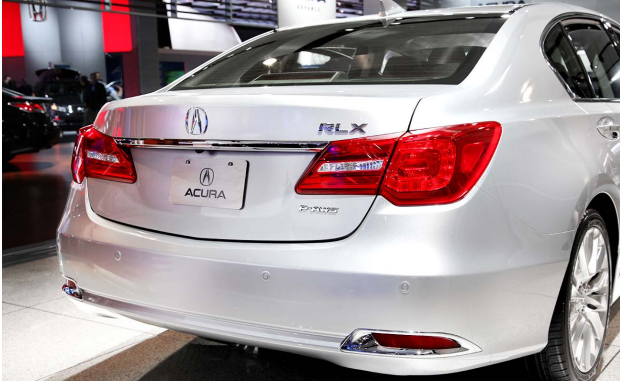
A rear bumper cover may have attachments such as lamps.
