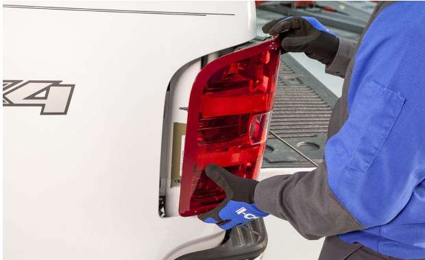
This tail lamp is being transferred to the reinstalled truck box.
