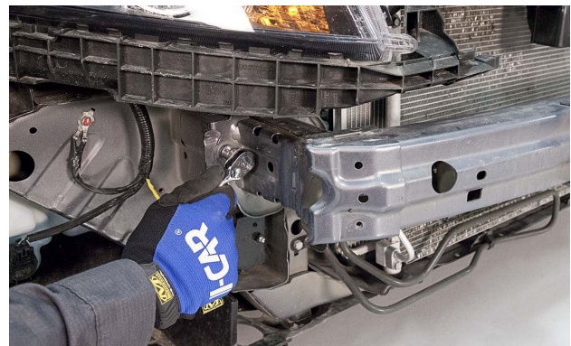
The bumper reinforcement on this vehicle is being replaced.
