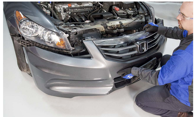
After removing this bumper cover, any hidden damage to the foam energy absorber will be revealed.
