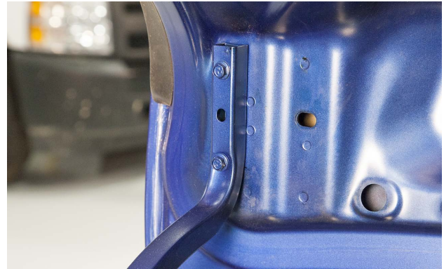
Deck lid hinges are designed to hold a deck lid in the open position.
