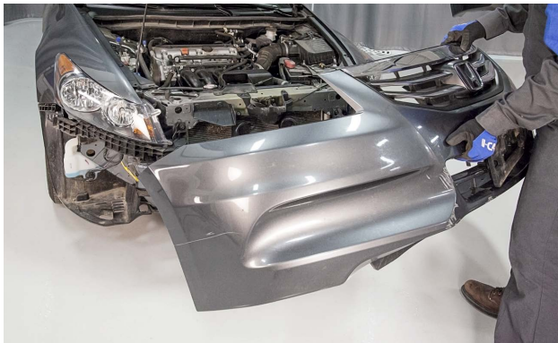
Due to the extent of damage, this bumper cover will be replaced.
