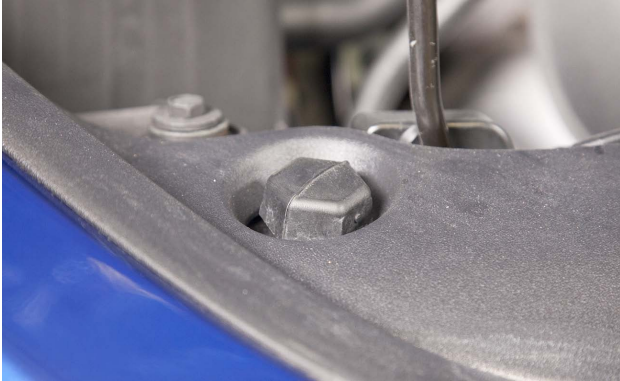
This hood stop is adjusted fully down.
