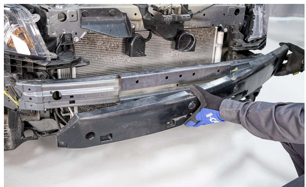
After removing this energy absorber, damage to the reinforcement is revealed.
