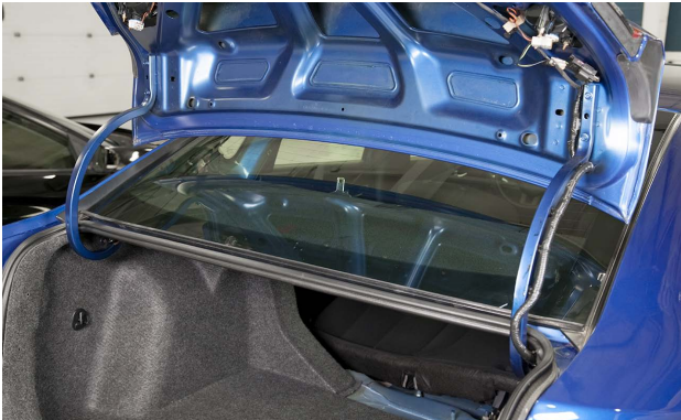
This deck lid has hinges mounted in the package tray area.
