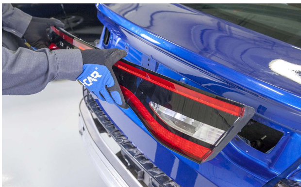
The deck lid attachments are being reinstalled.
