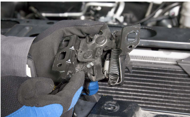
This cable is used to pull the release lever on this latch.
