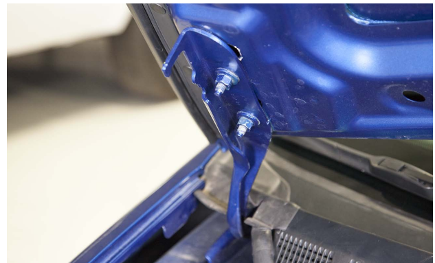
Hoods can be adjusted on the hinges or the hood stops.
