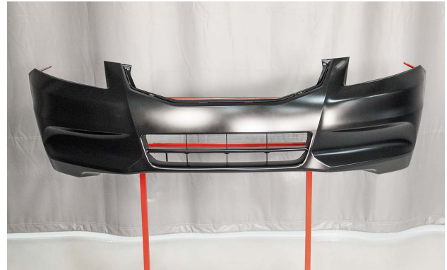
Replacement plastic bumper covers will require refinishing before installation.
