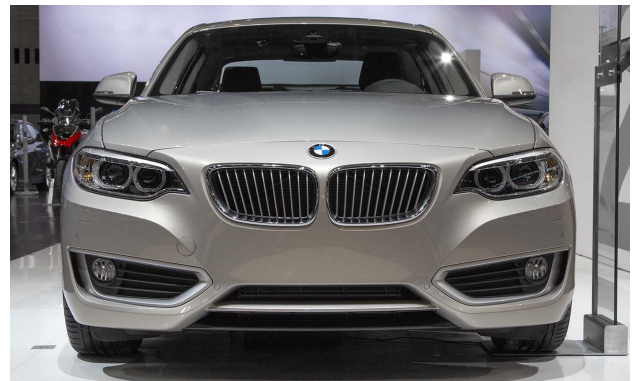
Grilles allow airflow into the engine compartment.
