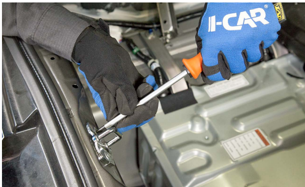
After the liftgate has the correct gaps, the striker is installed.
