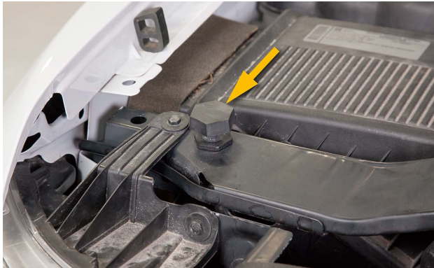
Adjusting the stops will change the flushness at the front of the hood.
