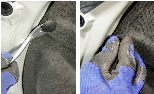
This hood insulation blanket is fastened to the hood with plastic retainers.
