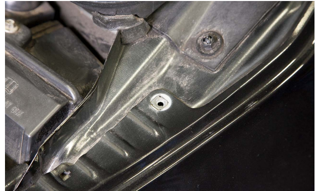
The U-clip in the slotted hole of an upper rail allows some adjustment in the fender.
