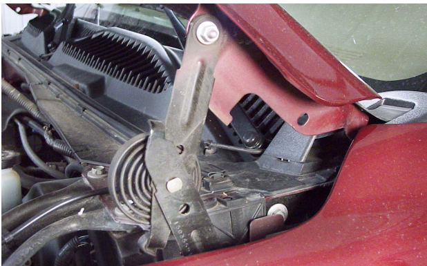
This hinge uses a coil spring to keep the hood open.
