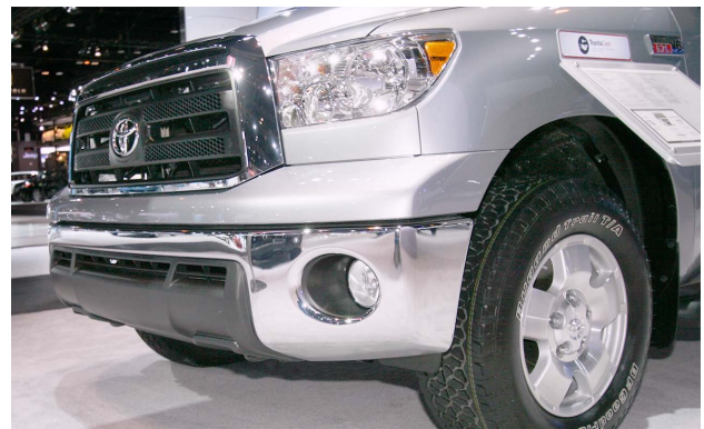
The bumper assembly on this vehicle is a combination of steel and plastic.
