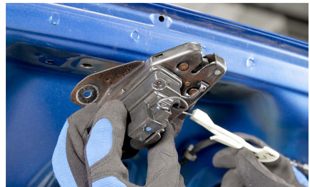
This deck lid latch is being reinstalled.
