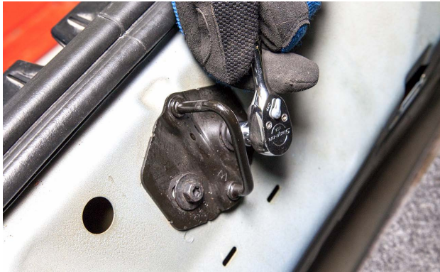
This deck lid latch striker is being adjusted.
