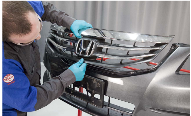
The grille may need to be re-attached on some bumper covers.
