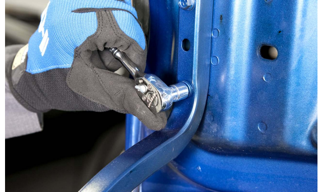
This hinge has elongated holes for adjustments.
