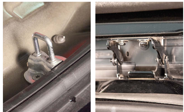
Shown are the liftgate striker (left) and hinge (right).
