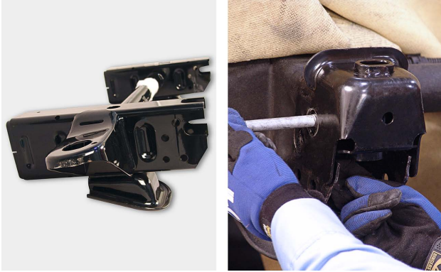
This bracket attaches the steel bumper to the frame (left). Brackets may be bolted to the frame assembly (right).
