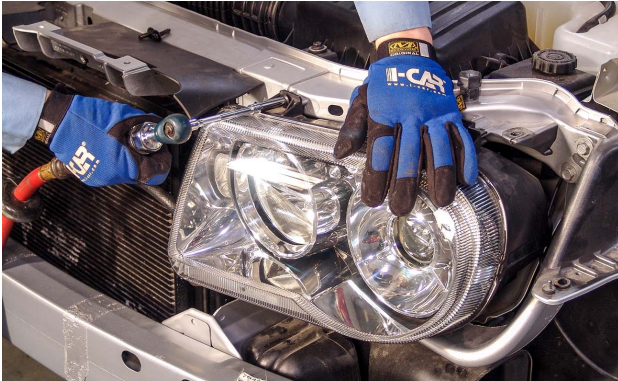
This headlamp mounting panel is attached to the radiator core support.
