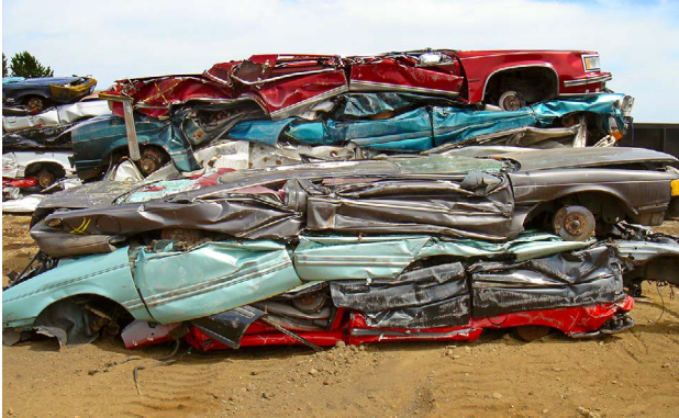
Vehicles are crushed for scrap metal after the usable parts and hazardous fluids have been removed.
