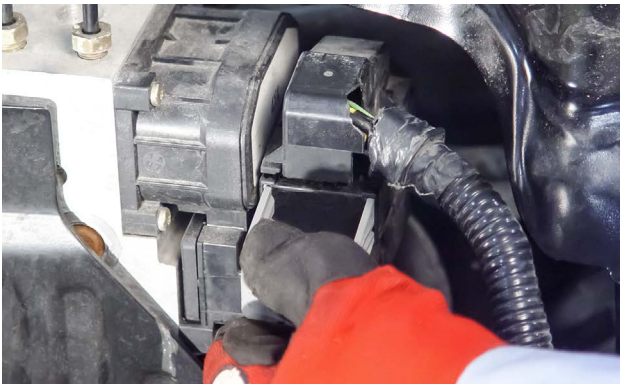
This ABS control module should be inspected for proper operation after installation.
