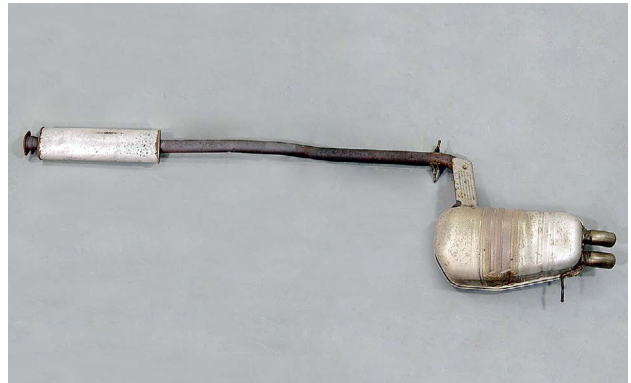
Recycled exhaust systems must be inspected for any visual defects.
