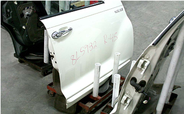
Recycled door shells do not typically include door mirrors.
