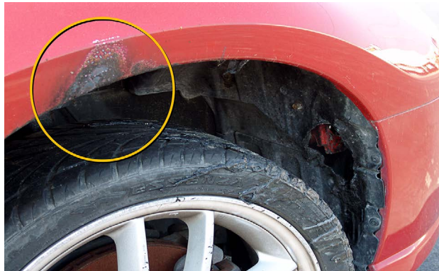
Fire-damaged parts should not be reused.
