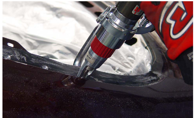
Drilling spot welds is required for separating quarter panels from the inner structure.
