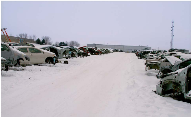
Vehicles that are acquired by the recycling facility are stored outside with most sheet metal intact.
