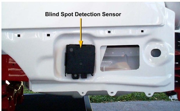
This is a blind spot sensor for the 2010 Ford Taurus, which is located near the bottom of the quarter panel.
