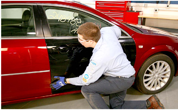
A visual inspection of the installed recycled part helps verify that the part matches the vehicle.
