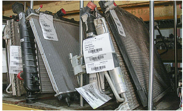
Recyclers may test the radiators before checking them into inventory.
