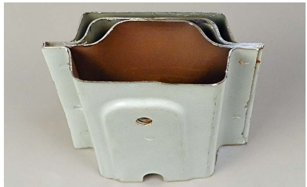
Multi-layered assemblies may make complete part replacement impractical.
