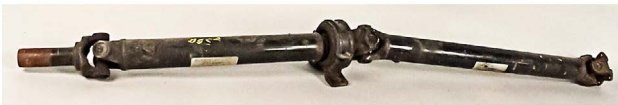
Recycled halfshafts and driveshafts should be inspected for evidence of previous repair.
