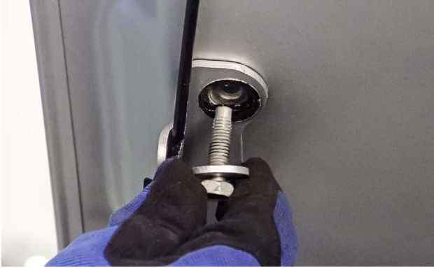
Aluminum parts, such as this hood, may require specific fasteners to avoid galvanic corrosion.
