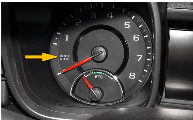
The "Auto Stop" on the instrument panel shows this vehicle is equipped with stop / start technology.
