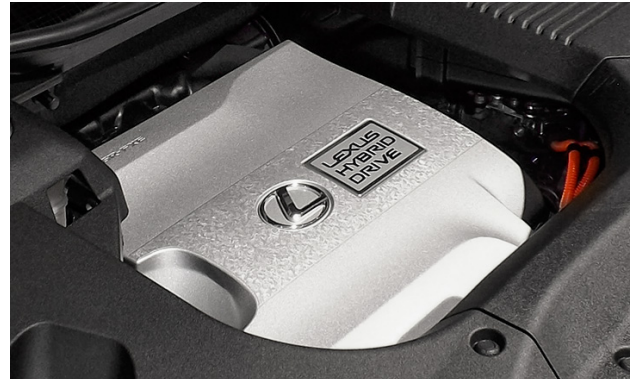
The word "hybrid" on the underhood cover panel is a common indicator.
