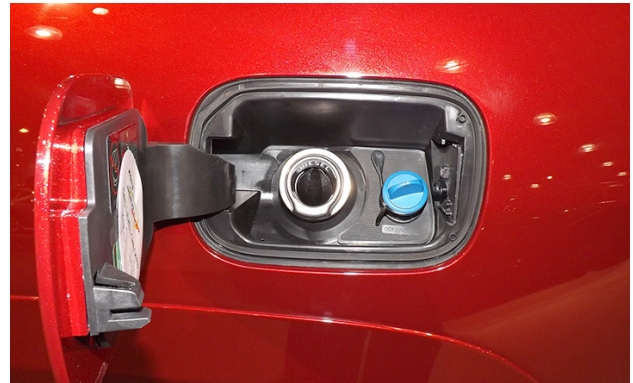
Modern diesel vehicles sold in North America have a separate tank and filler port for the diesel exhaust fluid.
