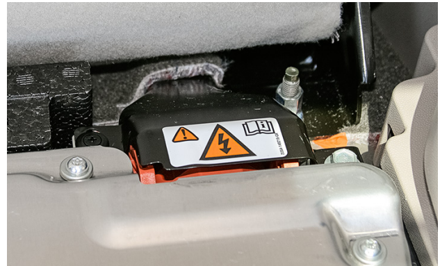
This label in the trunk on a Ford Escape Hybrid indicates the presence of the HV battery and to consult the service manual.
