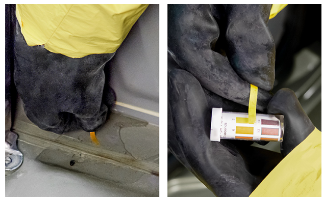
An electrolyte spill kit should include litmus strips to determine if the spill is acidic or alkaline.
