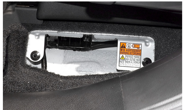
This "high voltage" label on the inside of the trunk on a Lexus RX450h also shows a drawing of the service disconnect.
