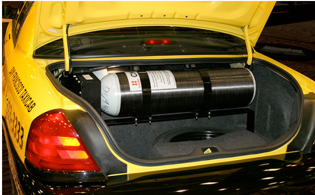
CNG requires a tank pressurized to 3,600 psi.
