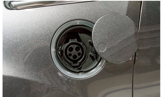
This is a standard configuration charge port on the Ford C-Max Energi plug-in electric vehicle.
