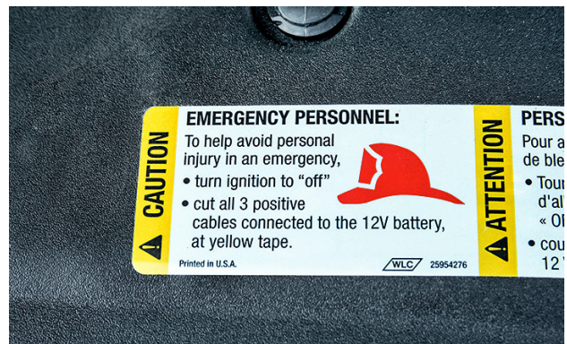
Emergency personnel are told the quickest way to cut the power to avoid personal injury.
