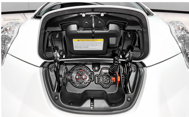
This is a closeup view of the charge port on the pure-electric Nissan Leaf, with the standard port on the right and fast-charge port on the left.
