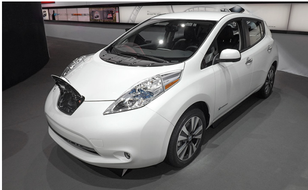
The charge port on the pure-electric Nissan Leaf is behind a flip-up door in the front.
