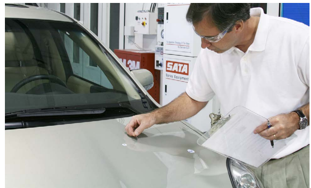
Tools may be used to help gauge the size of dents when writing estimates.
