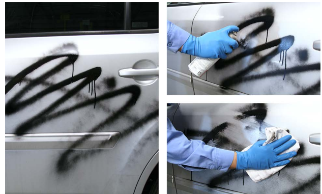
Spray paint removal products are available to remove graffiti from a finish.
