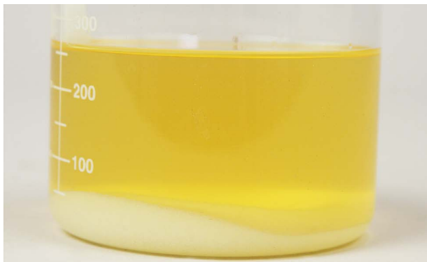
Sugar does not dissolve in gasoline and will sink to the bottom of the fuel tank.
