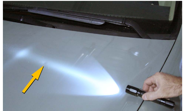
A flashlight held parallel and close to the panel can help identify hail dent locations.
