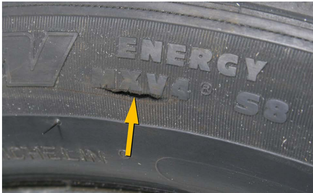
Tires that are punctured on the sidewall are not repairable.
