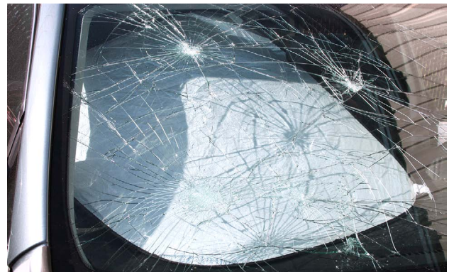
Glass that is damaged from very large hail may be replaced before body repair to prevent interior damage from moisture.
