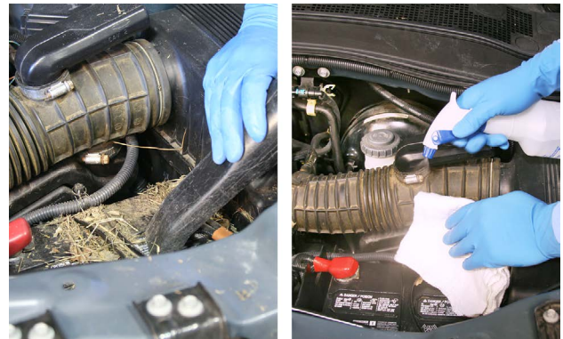
Cleaning up underhood infestation generally requires removing the nest and using an all-purpose cleaning solution to disinfect the area.
