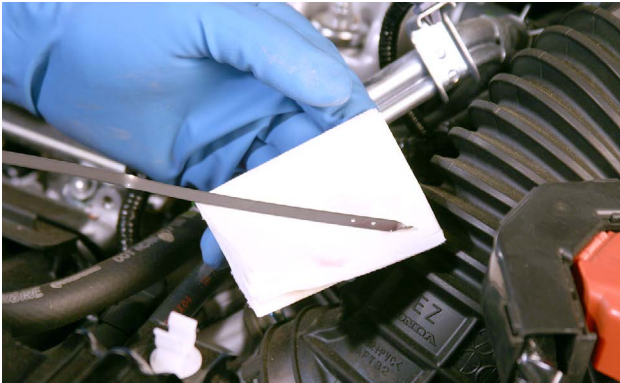
Fluid levels should be checked during damage analysis to ensure proper levels or that the fluid color looks normal.
