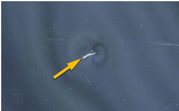
The scratching in the center of this dent makes it not a good candidate for PDR.
