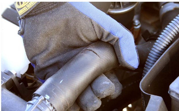
A cut radiator hose requires replacement.
