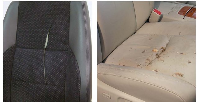
Slashed seat fabric may require replacement of the seat cover if not the entire seat, while mud stains on seats require proper cleaning.
