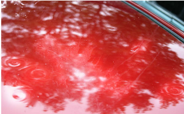
Raw eggs can etch the clearcoat if left to dry.
