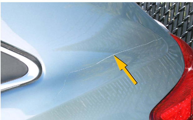
Deep key scratches require refinishing a panel.
