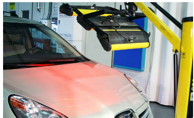
Heat may be used to soften aluminum panels before PDR is performed.
