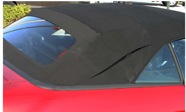
A slashed convertible top may require replacement of the fabric if the slash is not along a seam.
