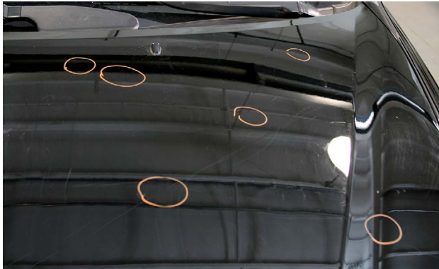
A water-soluble marker may be used to help identify the quantity and location of hail dents.
