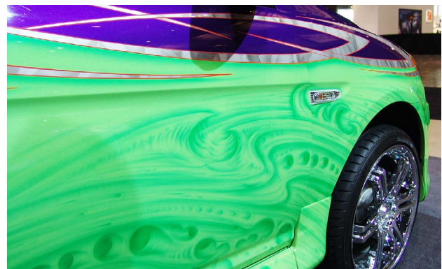
Damage to a custom finish, such as this, requires access to paint records on how the finish was created. This helps determine if the finish is repairable.
