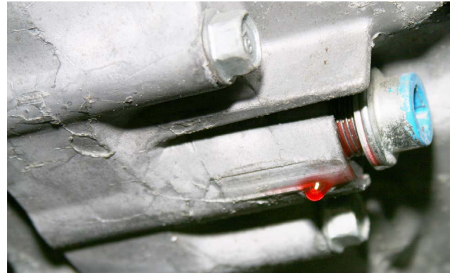
A loosened transmission fluid plug will slowly drain the fluid and lock up the transmission.
