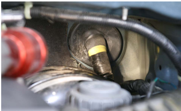
Check hole plugs to ensure rodents have not created entryways into the passenger compartment.
