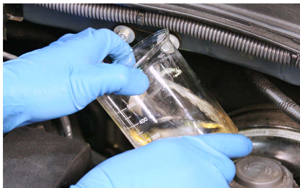
On this 2007 Honda Pilot, the fuel sample is collected from the engine compartment area.
