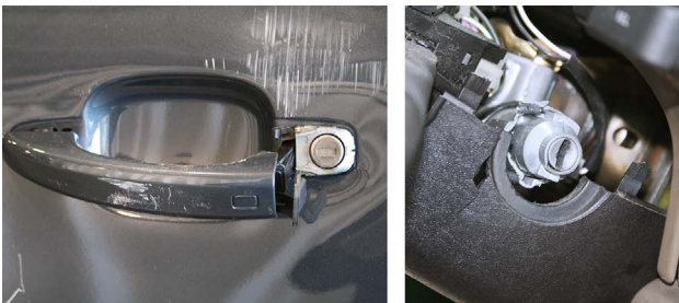
Damaged door handles or ignition cylinders are indications that the vehicle was forcefully accessed and driven.
