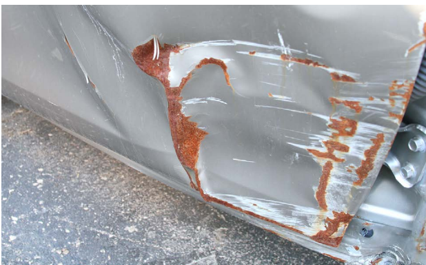
Rust always provides the best indication of previous damage.
