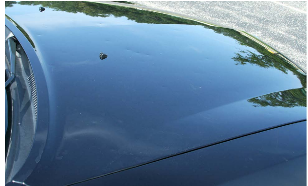
Hail often damages horizontal panels the most.
