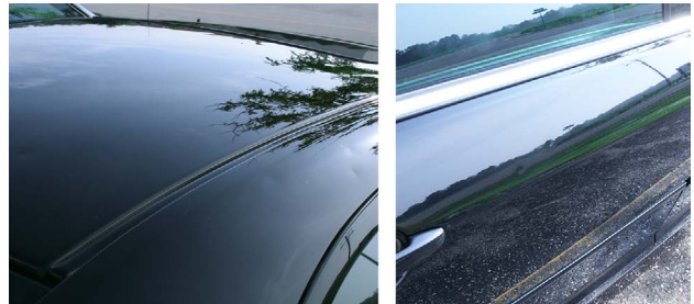
Look for inconsistency with hail damage. Generally, there is not a pattern to hail damage.
