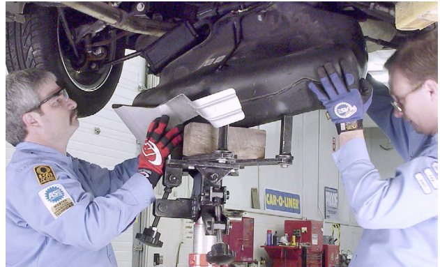
Dropping and cleaning the fuel tank is required for removing contaminants from the fuel system.
