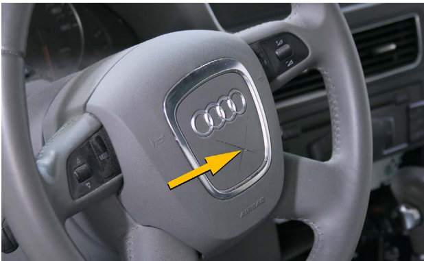
Slashed airbags require replacement. Repairs should never be made to airbag covers.
