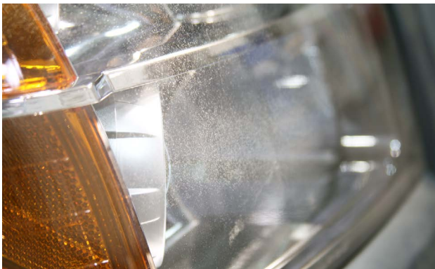
Wind-blown sand has scarred the headlamp lens on this vehicle.
