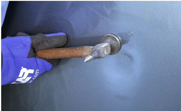
A hammer and dolly are common tools used to make conventional repairs to damaged metal.
