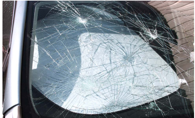
Glass that is damaged from hail is not repairable. The damage pulverizes the glass at the point of impact, making repair impossible.
