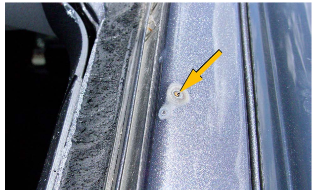
A direct lightning strike can blow a hole into the outer sheet metal of a vehicle.
