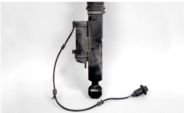
This shock absorber has an external damping valve to control the firmness of its damping force.
