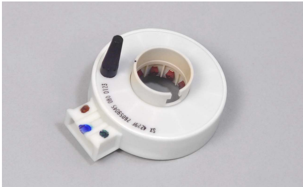
This is an example of a steering wheel position sensor from an electronically controlled steering system.
