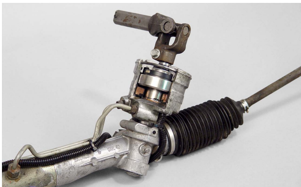
Electromagnetic fields control and vary the hydraulic fluid flow in this type of electronically controlled power steering system.
