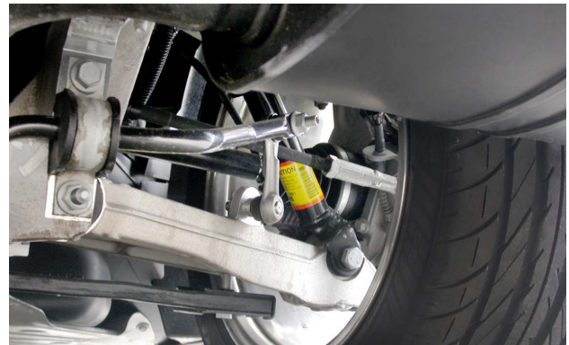
This magnetically controlled shock absorber looks like a typical conventional shock absorber from this angle.
