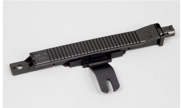
This is the receiving antenna located in the wheelhouse area of a BMW 745i with a direct tire pressure monitoring system.
