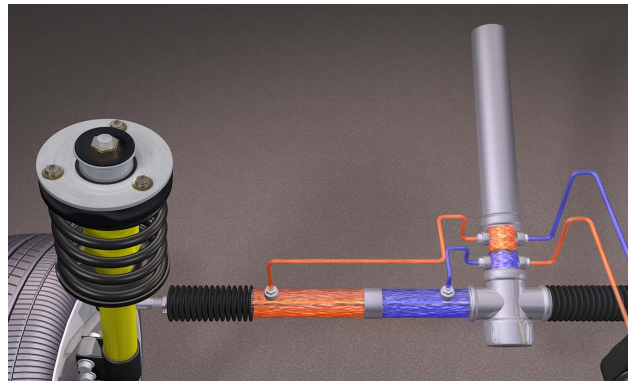
This illustration shows the high pressure hydraulic fluid assisting in pushing the rack in the direction of the turn while hydraulic fluid from the opposite side is returned to the fluid reservoir.
