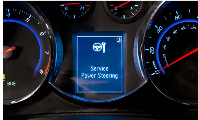
Some vehicles use an information message center instead of a MIL to warn of system problems.
