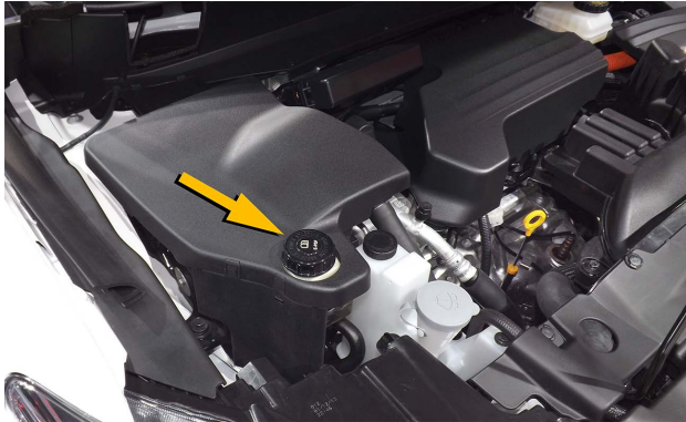
The reservoir tank is part of the electro-hydraulic power steering system on this vehicle.
