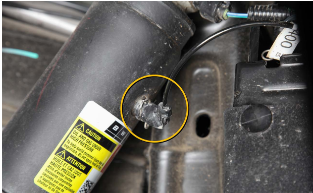
Shown here is the air line and connector on rear air shock absorber.
