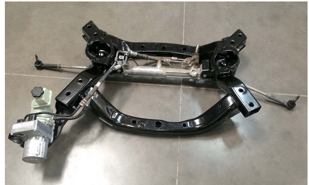
The electric assist motor and control module should be inspected for collision damage.
