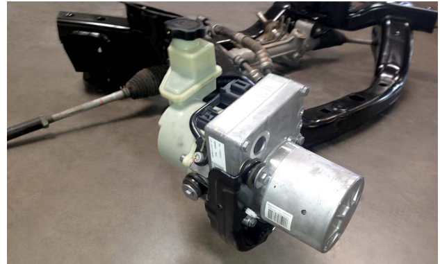
This is a power steering pump and motor assembly from a Chrysler 300.
