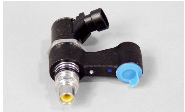
This solenoid valve is used to control fluid pressure at the fluid outlet of the power steering pump in an electronically controlled power steering system.
