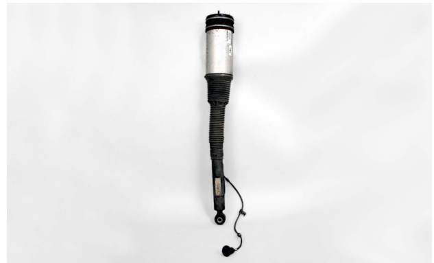
This variable damper air strut has been bent in a collision and requires replacement.
