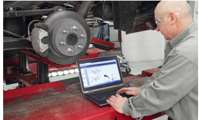
This estimator is looking up a repair procedure in the vehicle service information.
