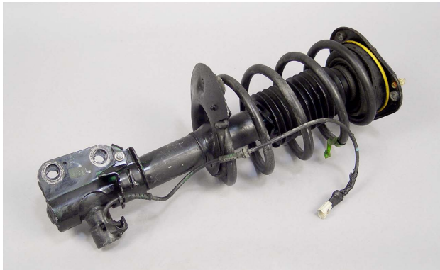
The computer controlled damper on this strut assembly has the fluid control valve located externally at the bottom of the strut.
