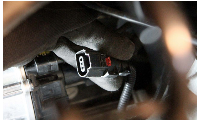
Inspecting for collision damage includes checking connectors for cracks or breakage.
