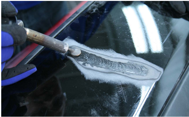
When using an airless welder, the filler rod is blended into the base material.
