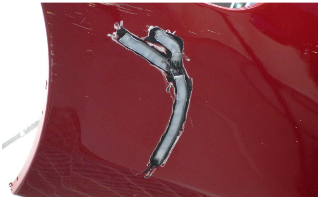
This repair was made with hot air welding equipment.
