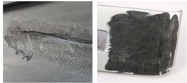
This sanding test shows that the part is a polyolefin.
