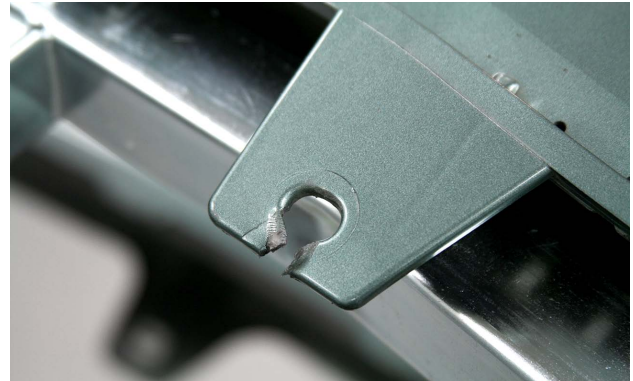
This partially-torn tab is repairable.
