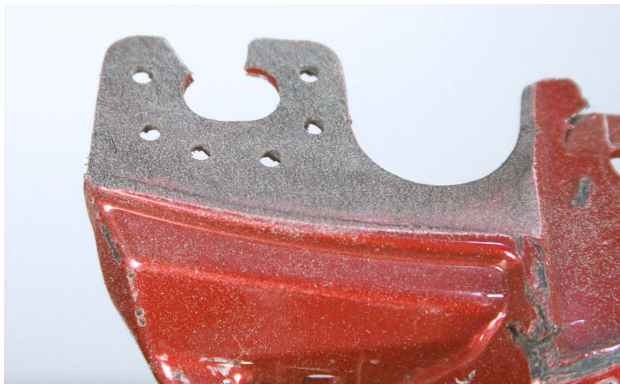
This tab has 1/8" pinning holes that will provide strength for the repair.
