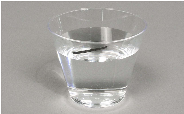
This float test shows that the piece of plastic is likely to be a polyolefin.
