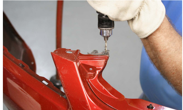
1/8" pinning holes are being made to help anchor a replacement tab.
