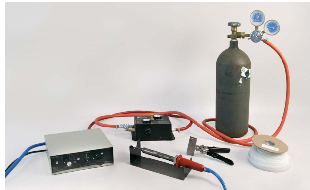
A nitrogen hot air welder can only be used on thermoplastic parts.
