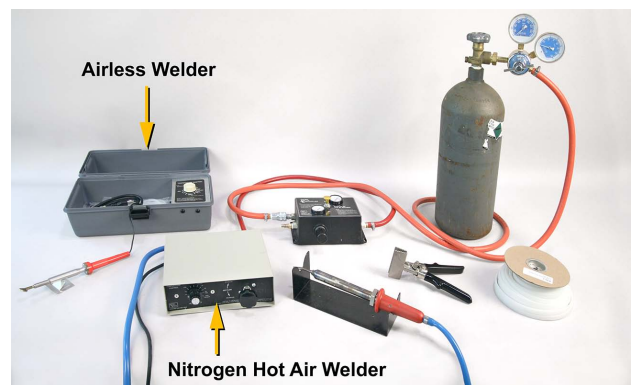
The two types of plastic welders are airless and nitrogen / hot air welders.
