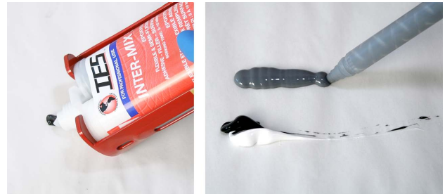
Running out a bead of repair product will ensure the product is properly mixed before use.
