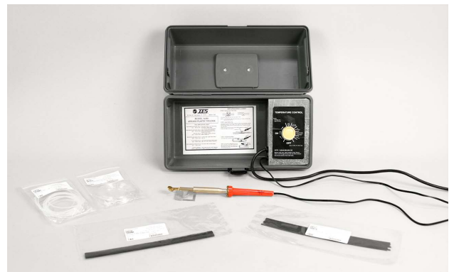
This airless welding kit includes 110-volt power supply, a flat-bottomed welding shoe, and filler rods.
