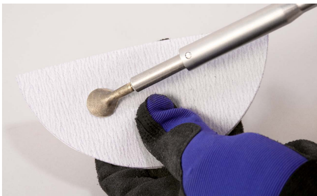
The welding shoe can be cleaned with P220 grit sandpaper while the tip is hot.
