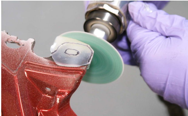
A grinder is used to shape the new mounting tab.
