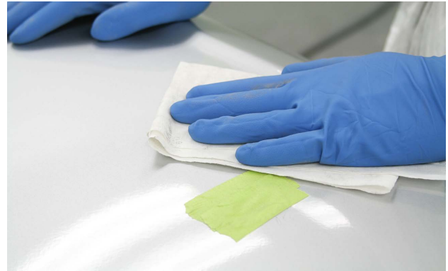
Damaged SMC parts should be cleaned before making any repairs.
