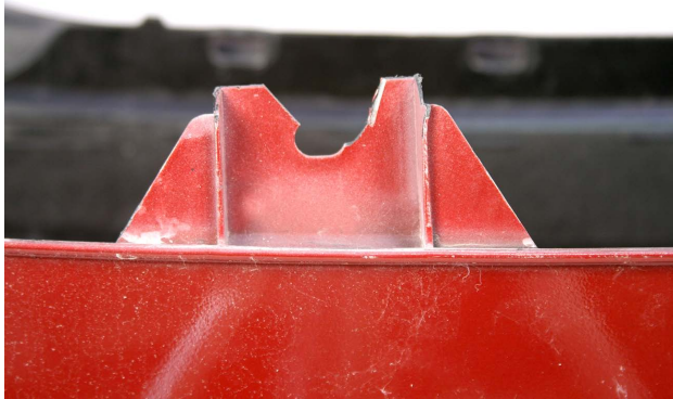
Broken-mounting tabs can be recreated if a portion is missing.
