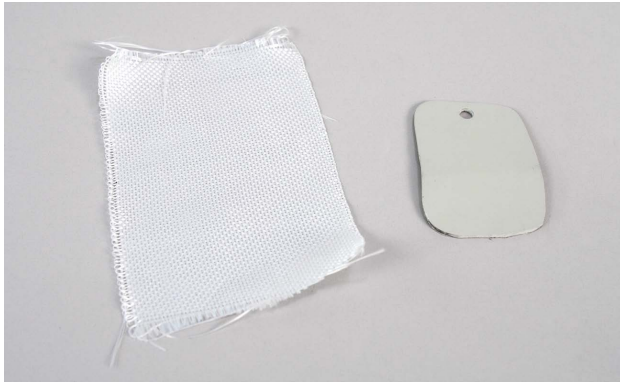
The backing material can be a fiberglass cloth (left) or a scrap piece of the same material (right).
