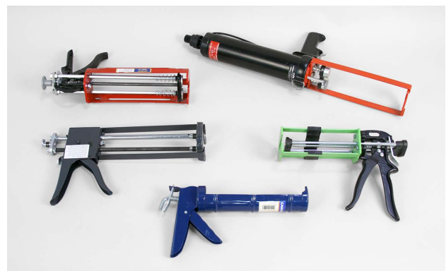
There are a variety of applicator guns used to dispense repair adhesive.
