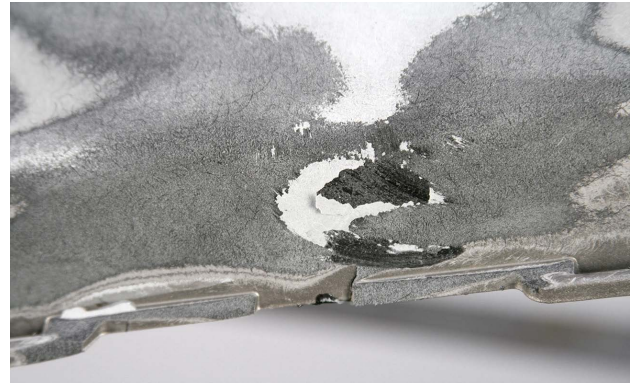
If the plastic becomes overheated from sanding, the plastic repair adhesive may lift.
