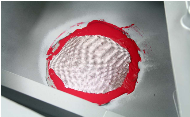
The backing should be pressed into the composite repair adhesive.
