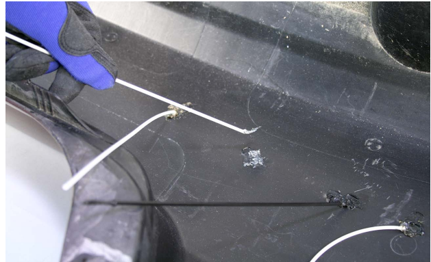
A rod adhesion test may be used if the ISO code is not available.
