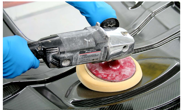
Minor scratches in an exposed-weave carbon fiber body panel may be removed by buffing the area.
