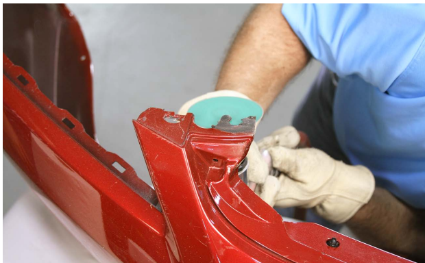
The finish is being removed from the repair taper area.
