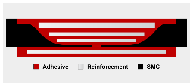
Alternating the composite repair adhesive and backing material make the pyramid patch.
