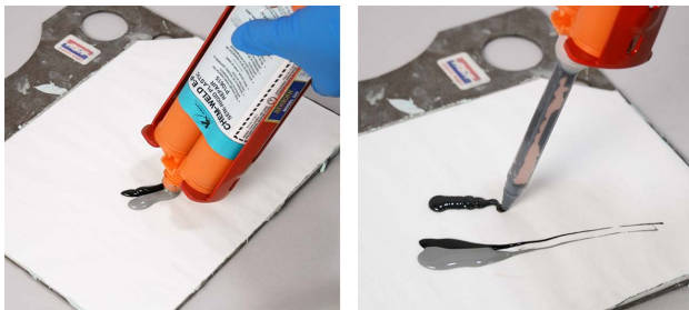
Dual cartridge tubes must always be leveled before use.
