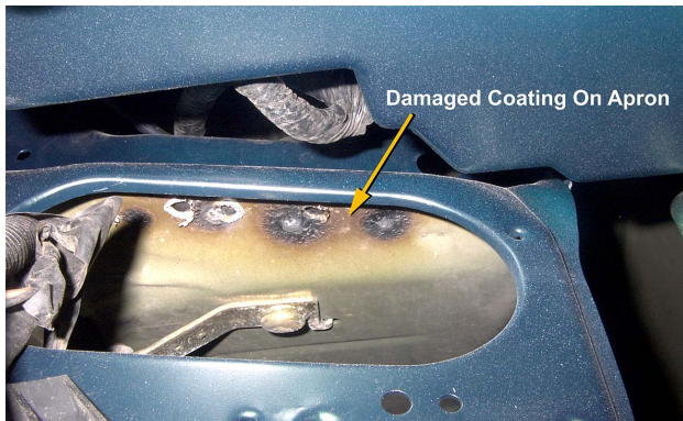
The coatings on the backside of this apron are damaged and must be replaced.
