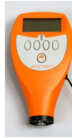
A film thickness gauge may help determine if chip-resistant coatings were replaced properly. The OEM service information may specify locations and thicknesses for replacement chip-resistant coatings.
