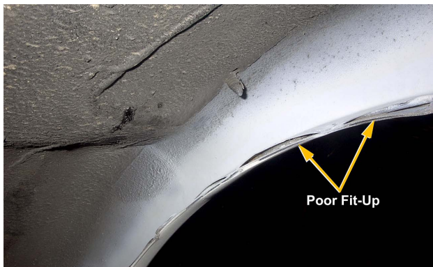
The distorted mating flanges of this quarter panel and wheelhouse may lead to corrosion.
