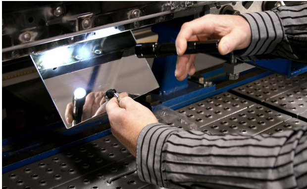
Shining the flashlight into a mirror will reflect the light onto the repair area.
