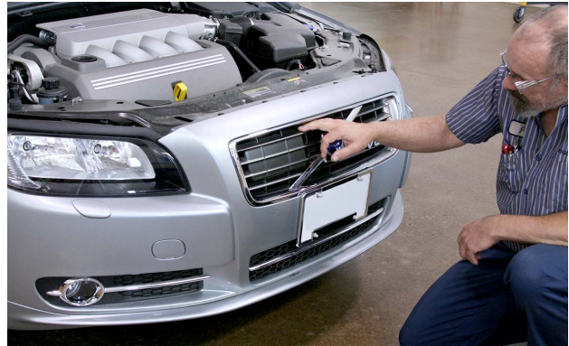
A radar sensor for a collision warning system is being inspected for proper installation.
