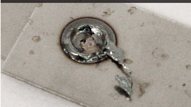
Excessive Metal Throwout
