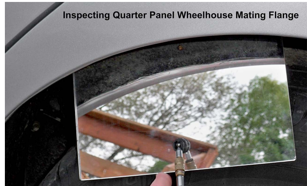
A mirror is being used to inspect the mating flange of this quarter panel and wheelhouse.
