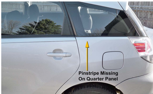
The pinstriping is missing on this replaced quarter panel.
