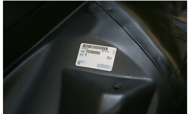
The service part label should be removed from this replacement apron.
