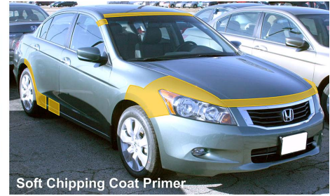
A film thickness gauge may help determine if chip-resistant coatings were replaced properly. The OEM service information may specify locations and thicknesses for replacement chip-resistant coatings.
