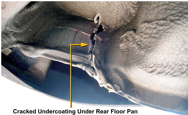
Cracked Undercoating Under Rear Floor Pan
