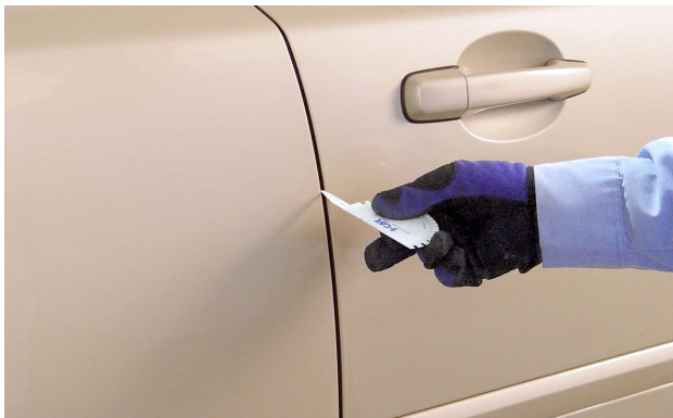
A gap gauge is being used to verify this door gap is consistent.
