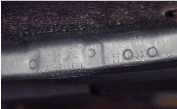
Clamp marks from vehicle straightening equipment can be seen on this pinchweld flange.
