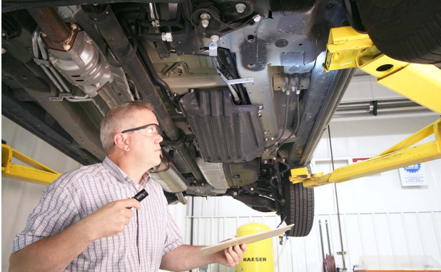
A vehicle lift provides the best access for inspecting underbody repairs.
