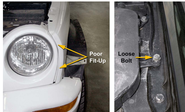
Fenders should be inspected for proper fit-up and that all the bolts are properly tightened.
