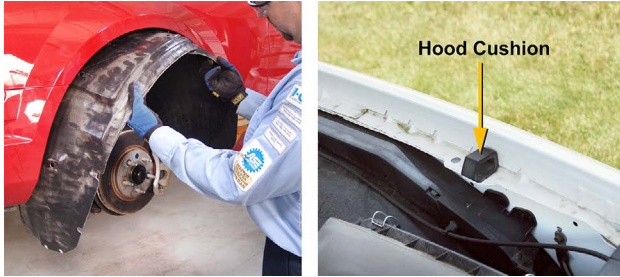
This fender liner is being removed (left). This is an example of a hood cushion attached to the fender (right).
