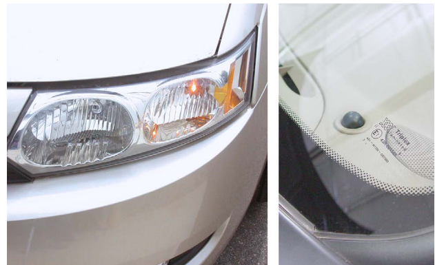
This vehicle has an amber-colored daytime running lamp (left). This is an example of an ambient light sensor (right).
