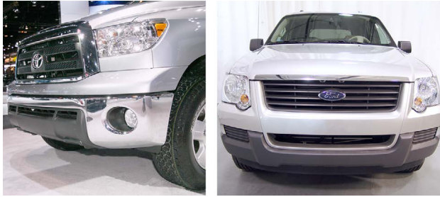
This pickup truck has a chrome-plated steel facebar (left). The front bumper cover on this pickup truck is made of plastic (right).
