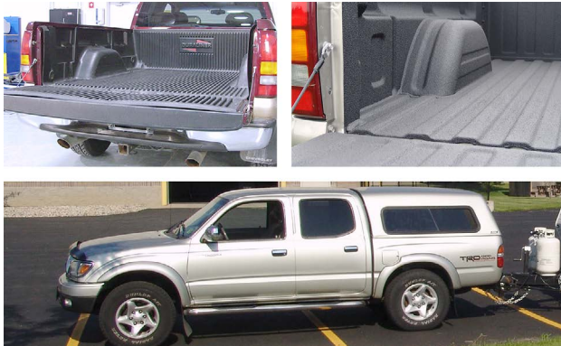
This is an example of a drop-in bedliner (top left). This is an example of a spray-on bedliner (top right). This pickup truck has a cover attached to the box assembly (bottom).
