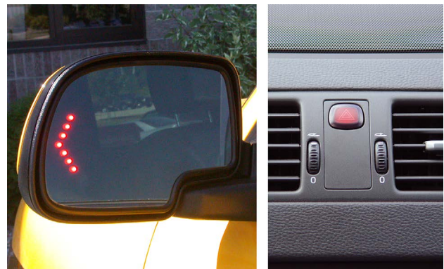
Some vehicles have a turn signal lamp as part of the mirror glass or as a separate lamp on the bottom of the mirror housing (left). The hazard switch will often flash with the exterior lamps (right).
