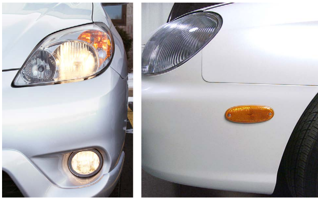
This vehicle uses the same bulb for the parking and marker lamps (left). Some vehicles will have a reflector instead of a side marker lamp (right).
