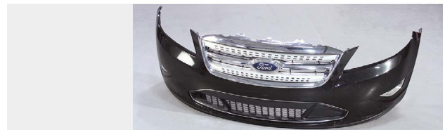
This grille is attached to the hood (left). This grille is attached to the bumper cover (left).
