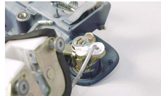
This shows a door lock cylinder (top left). A linkage rod is connected to the door lock cylinder (bottom left). The door is being locked with the remote control key fob (right).
