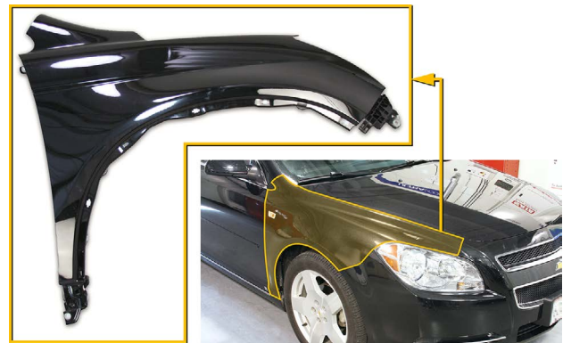
The fender that has been removed from a vehicle (left). The highlighted area shows a fender attached to a vehicle (right).
