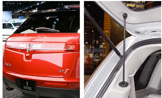
This photo shows the liftgate on a 2010 Lincoln MKT (left). This photo shows one of two strut rods used to hold the liftgate open (right).
