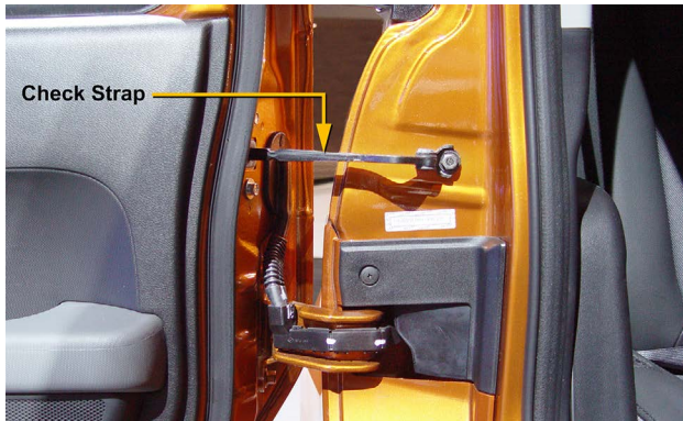
This check strap is bolted to the vehicle structure.
