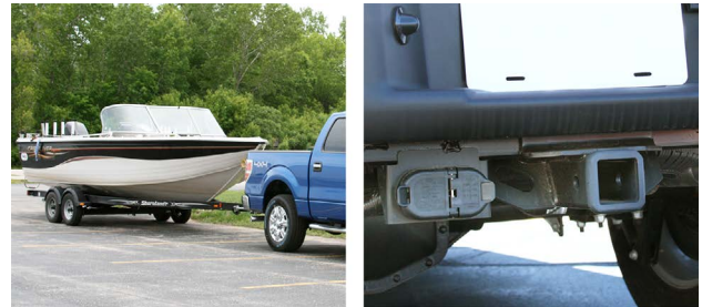
Trailers may come equipped with its own set of marker lamps (left). A special connector is required for proper trailer lamp operation (right).
