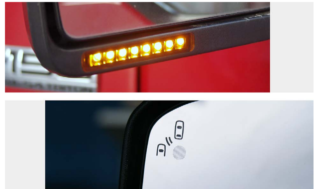
This turn signal is a series of LEDs (top). An indicator lamp for the blind spot detection system is on this mirror (bottom).
