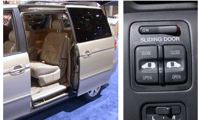
The sliding door is open on this minivan (left). These are the controls for an automatic sliding door (right).
