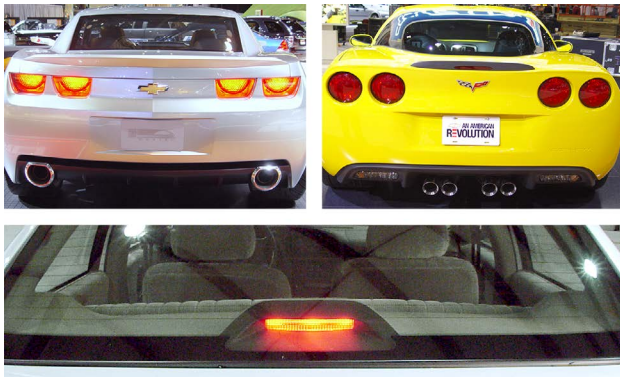
There may be multiple brake lamp lenses (top left). The reverse lights on this vehicle are at the bottom of the bumper cover (top right). High-mount brake lights may also be called a third brake light (bottom).
