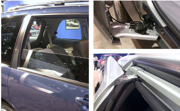
This van is equipped with a power window in the sliding door (left). The bottom track for the sliding door (top right). The top track for the sliding door (bottom right).
