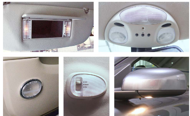
These lamps will light only when the mirror is visible to the occupant (top left). The lamps in an overhead console are often called reading or map lights (top right). Lamps in door trim may be red, white, or amber (bottom left). Dome lamps often have an ON/OFF switch that will only control the dome light (bottom middle). This lamp is used to illuminate the ground by the driver's door (bottom right) .
