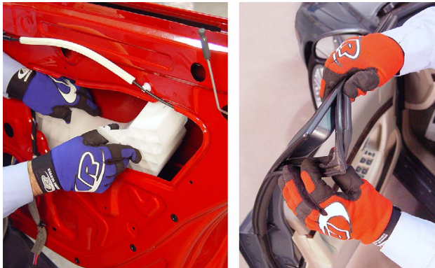
Energy absorbing foam is located in the door shell on this vehicle (left). The weatherstripping is being removed from this door (right).
