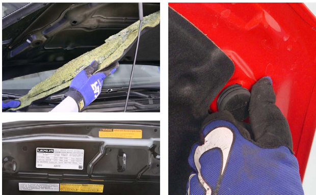
The hood insulator is being removed (top left). Various labels are attached to the bottom side of this hood (bottom left). The hood stop is being adjusted to align the hood to the proper height (right).
