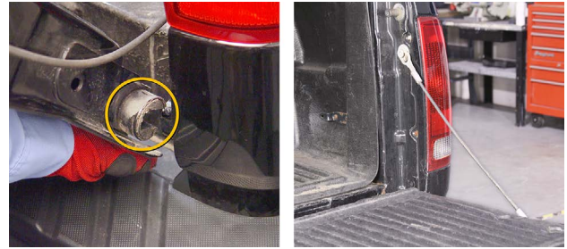
The cup that forms a pivot point is circled in this photo (left). A cable is attached to the box assembly and tailgate to prevent it from opening too far (right).
