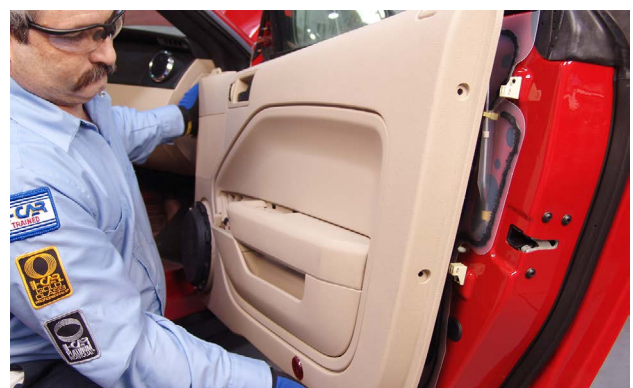
The interior door trim panel is being removed from the door.
