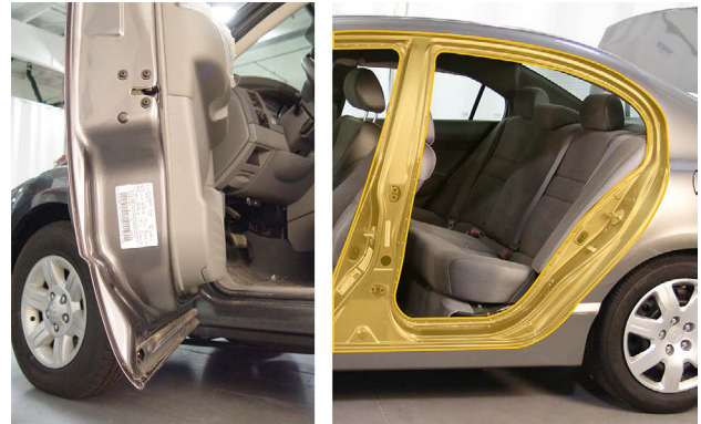
An information label is located on the doorjamb area of this door (left). The doorjamb areas on the vehicle are highlighted (right).
