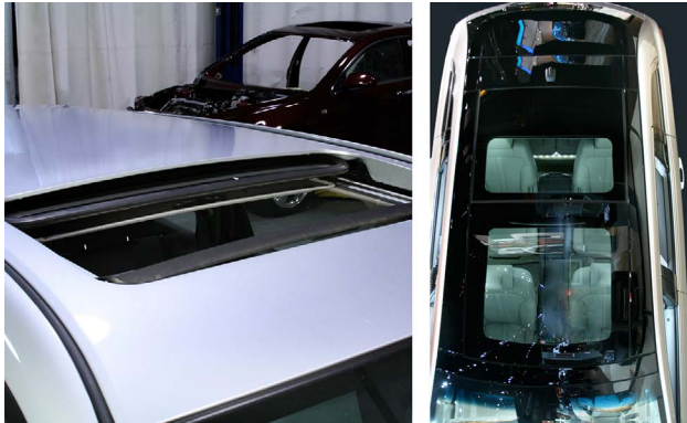
This is an example of a power sunroof (left). This is an example of a panoramic roof (right).
