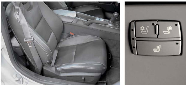
A seat is primarily for comfortably sitting in a vehicle, but there are several safety options in a seat (left). These are controls for climate-controlled seats (right).
