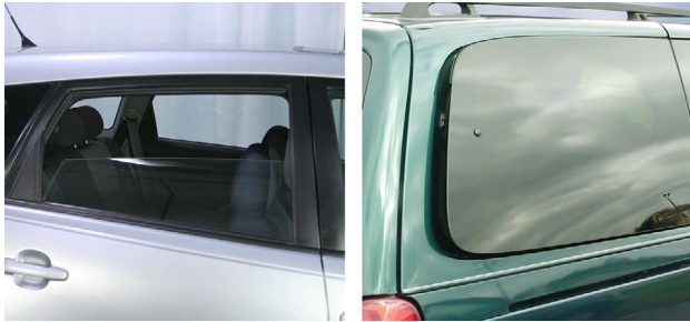
This sliding door glass is in the down position (left). This hinged vent glass allows air to flow into the passenger compartment (right).
