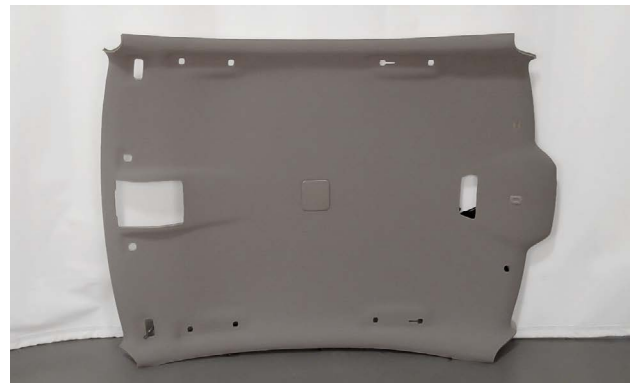
This is a stiff headliner that keeps its form outside the vehicle.
