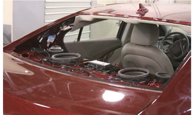
This package tray, without the trim cover, shows some of the parts that are located on this back shelf.
