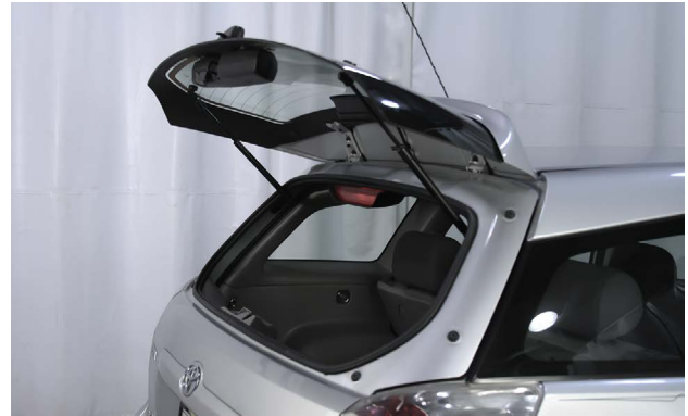
The glass on this liftgate has hydraulic struts that hold the glass open.
