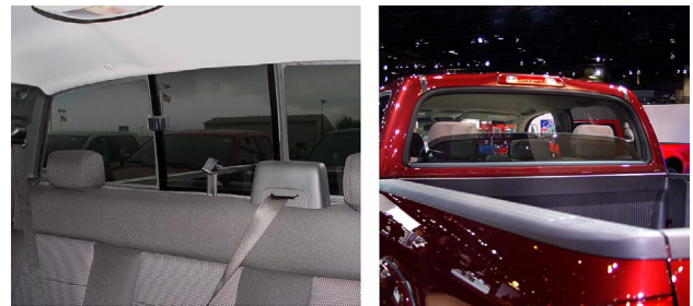
The backglass on this pickup truck can be manually opened by sliding the middle glass (left). This is an example of a power-operated pickup truck backglass on a Toyota Tundra (right).
