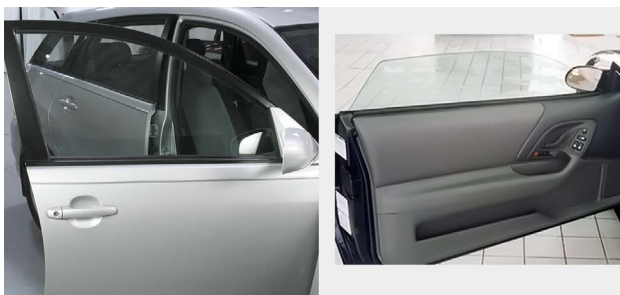
This is an example of framed door glass (left). This is an example of frameless door glass (right).
