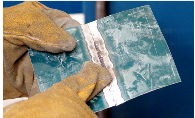
Just like the other joint types, test open butt joint welds should be visually inspected.
