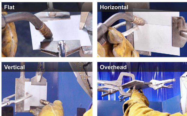
Welding may be required in any one of four positions when doing collision repairs.
