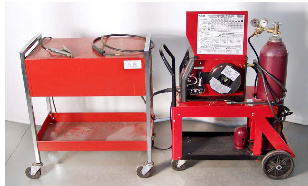
GMA (MIG) welders all have the same basic parts regardless of their type or size.
