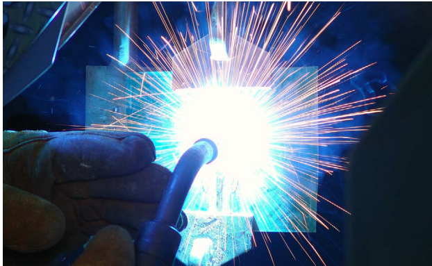
The travel speed, or how fast the welding gun is moved along the joint, has an effect on the weld being made.
