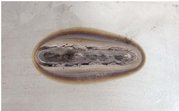
The ripple on the backside of this weld is an indication of good weld penetration.
