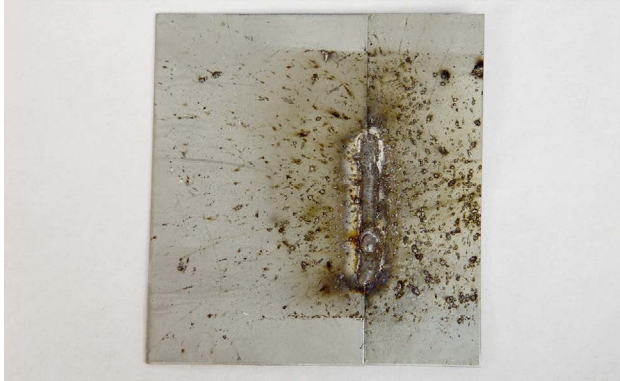
Excessive spatter may be caused by welding on dirty or contaminated metal.
