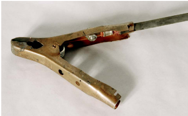
This work clamp completes the electrical circuit for the output of the welding machine, but is not the electrical ground for the input side.
