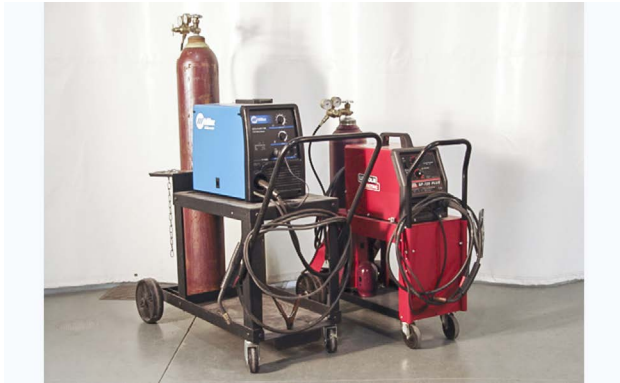
These are examples of 115 volt GMA (MIG) welding machines that are commonly used for collision repairs.
