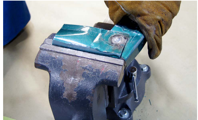
This test plug weld has passed the visual inspection and is being destructively tested with a twist test.
