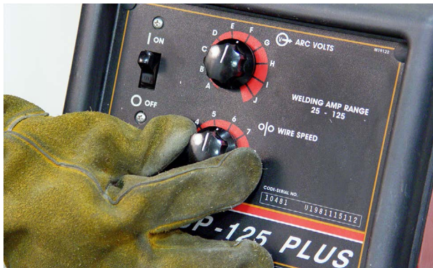
The amperage output of this welding machine is being changed by adjusting the wire speed.
