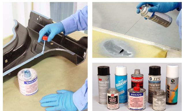
Weld-through primers may be brush-on (left) or aerosol (upper right). Shown are some examples of weld-through primers (lower right).
