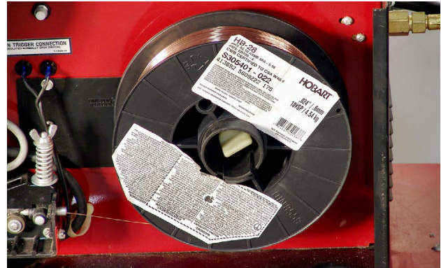
The label on this spool of electrode wire has a wealth of information, including the size of the wire and the AWS code for the wire type.
