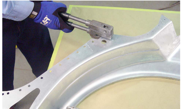
A hand punch is a good method of making plug weld holes in parts.
