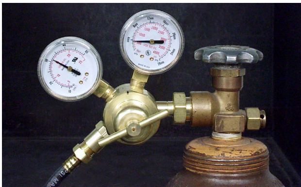
This regulator is designed for use on a 75% argon / 25% CO 2 shielding gas cylinder.
