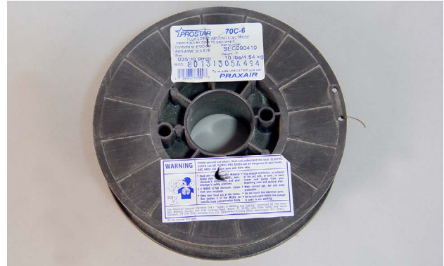
This is an example of a spool of flux-cored electrode wire that may be recommended for specific applications by some vehicle makers.
