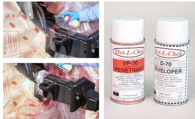
Dye penetrant is being applied to the welds for this full frame sectioning joint to check for cracks and other flaws (upper / lower left). One example of a dye penetrant is shown here (right).
