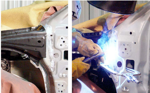
A fillet weld on lap joint is used where this upper frame rail attaches to the A pillar (left). This fillet weld on lap joint is being made in an area where it will not require dressing (right).
