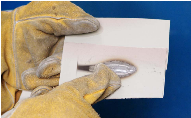
The backside of the practice weld must be inspected for evidence of penetration.
