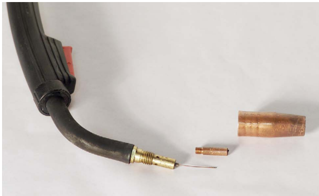
The contact tip and gas nozzle are removed from this welding gun assembly.
