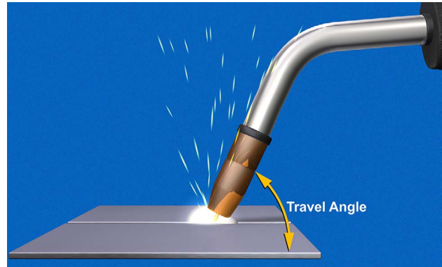
Travel angle is the angle between the gas nozzle and the workpiece in relation to the direction of gun travel.
