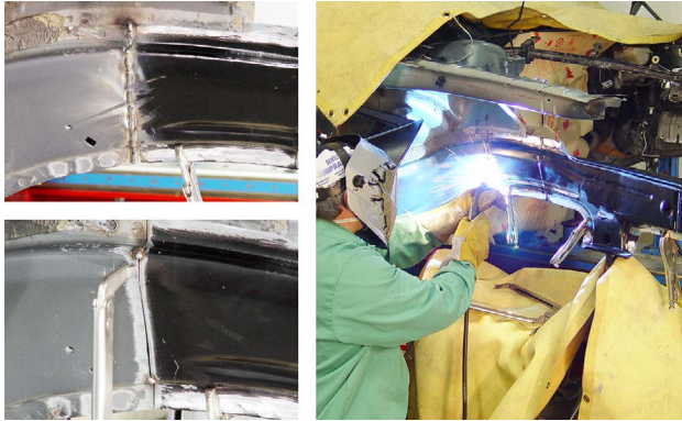
After careful cleaning and fit-up, this open butt joint weld was made using a stitch weld technique to avoid excessive heat buildup.
