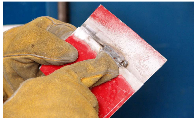
The front side of the practice weld is being visually inspected for flaws.
