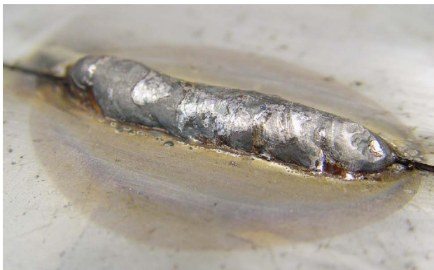
Too high a wire speed with too slow a travel speed may cause an excessive amount of weld metal to be deposited on the weld bead.
