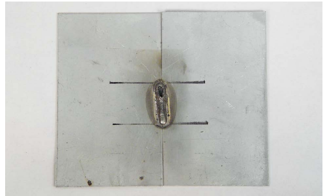
The porosity holes in one end of this weld were the result of a blocked shielding gas nozzle.
