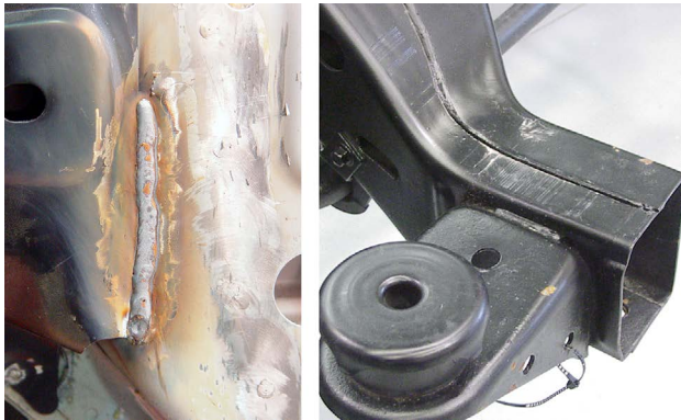
This fillet weld on lap joint and fillet weld on corner joint are examples of fillet welds that may be found on vehicles.
