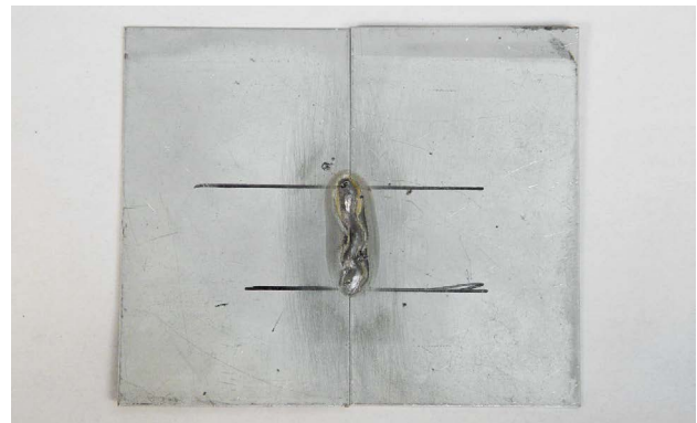
This distorted bead was caused by a technician's unsteady hand when welding.
