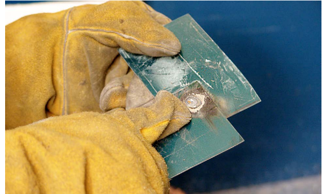
This practice, or test, plug weld is being visually inspected on the front side for flaws.
