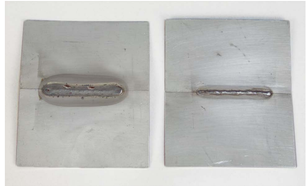
These welds show the difference in weld bead shape and heat input between a fast and slow travel speed, with all other parameters being the same.
