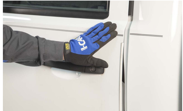
The opening and closing effort is checked to verify proper alignment.
