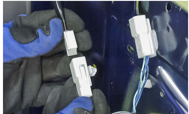
Door wiring harnesses use connectors to provide power to the door accessories.
