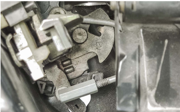
This latch is equipped with a child lockout mechanism.
