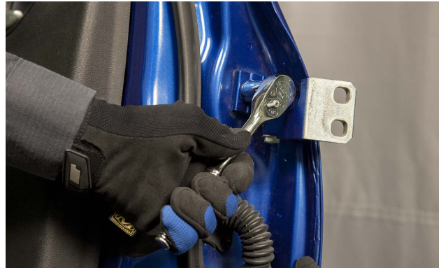
Tighten fasteners only enough to allow for adjustments. Torque once necessary adjustments have been made.
