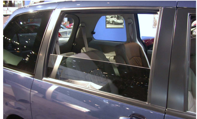
This van is equipped with a power window in the sliding door.
