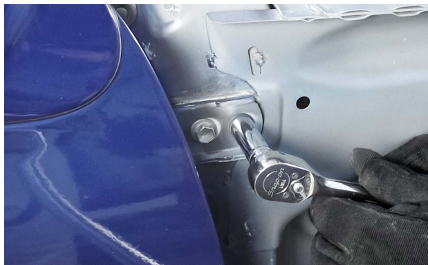
This hinge can be adjusted up and down and forward and rearward.
