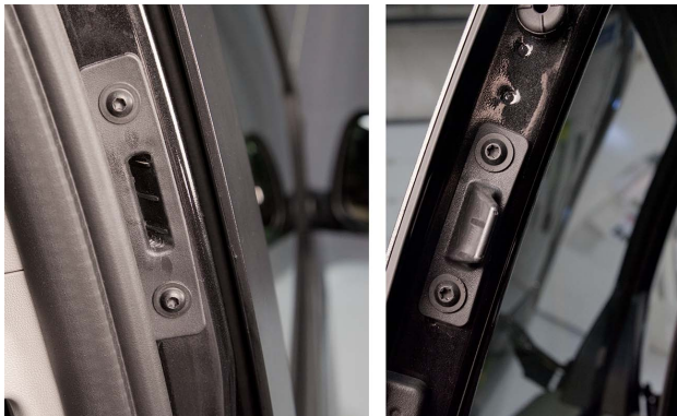
The plunger mechanism carries electricity to the sliding door accessories.
