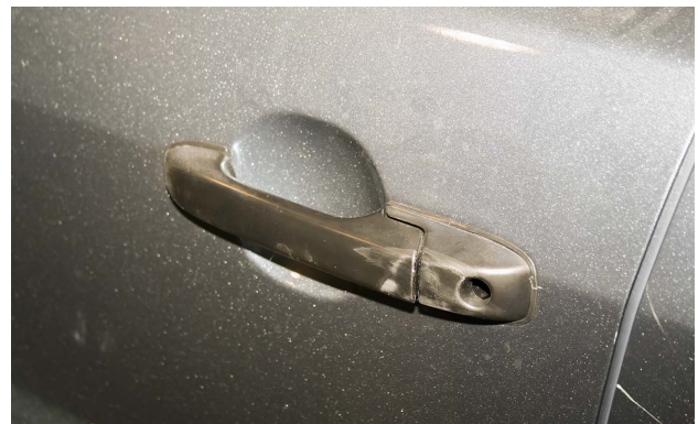
Outer door handles are connected to the latch mechanism by rods and clips or by cables.
