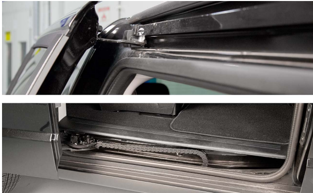
On this van, the sliding door tracks are located at the roof and rocker panel areas.
