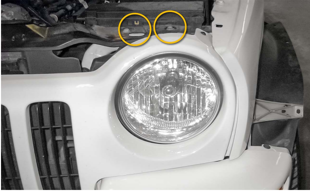
A body-over-frame vehicle may have a bolted radiator core support. A unibody core support is usually welded to the vehicle structure.
