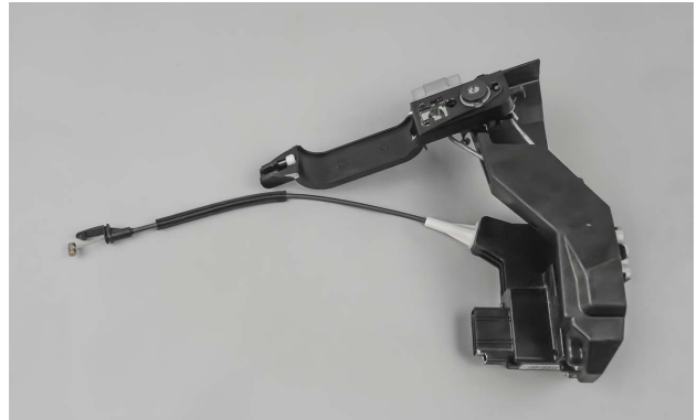
Inner and outer door handles are connected to the latching mechanism.
