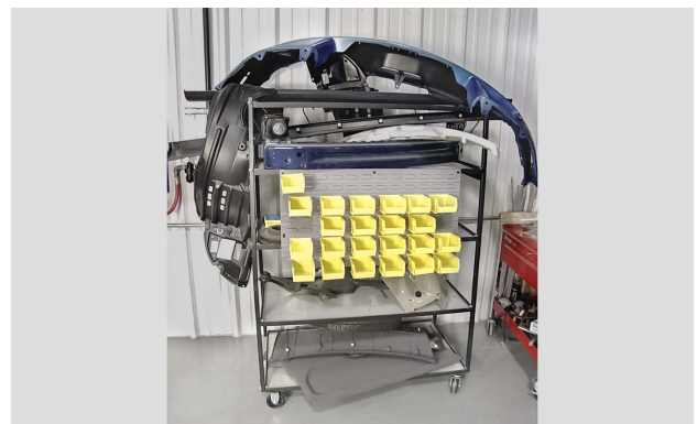
When disassembling a vehicle, a parts storage rack will help keep fasteners and parts organized.
