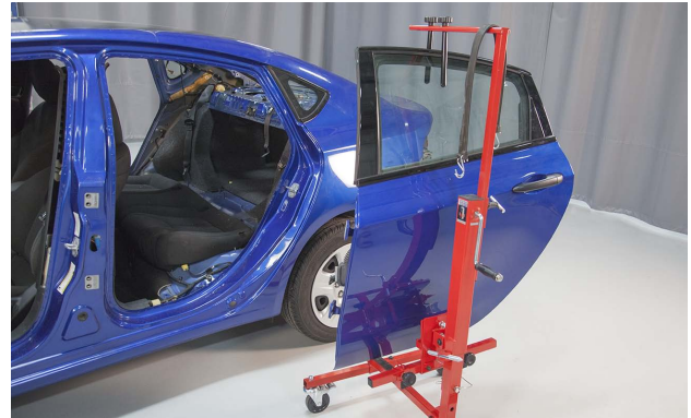
To safely remove a door from a vehicle, use a door stand or the help of an assistant.
