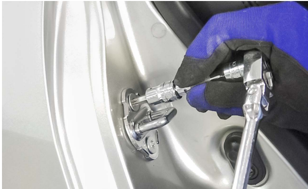
A Torx driver is used to remove this door striker.
