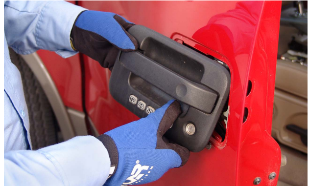
This door handle is being positioned to reinstall the fasteners.
