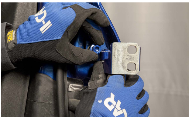
Inspecting the finish condition on the mounting area may be helpful when aligning the hinge.
