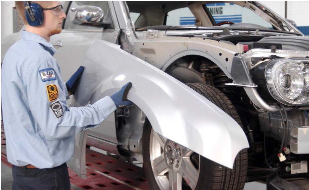
A recycled fender is temporarily installed for test-fitting.
