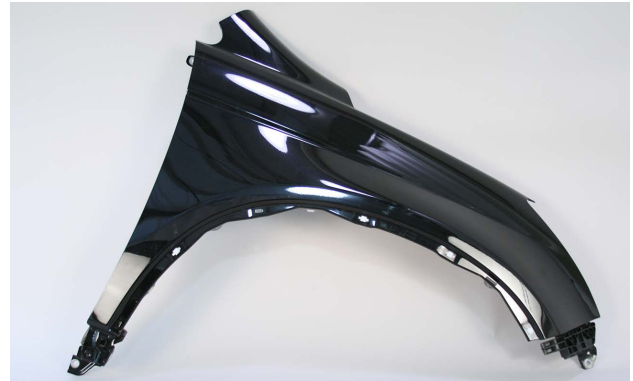
Do not install recycled parts if there are signs of pitting from corrosion or cracks at mounting locations.
