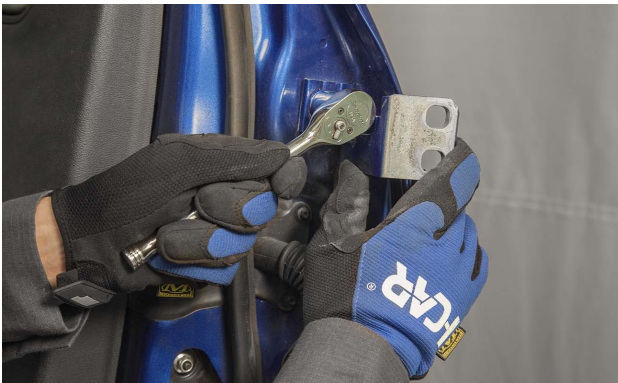
A ratchet can be used to remove the hinge-to-pillar fasteners.
