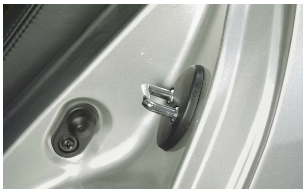
The striker may have some adjustment, but should not be used to adjust door height.
