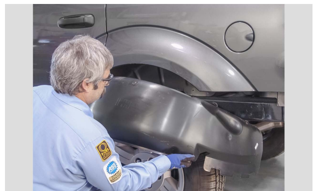
This plastic wheelhouse is removed to access hidden fasteners.
