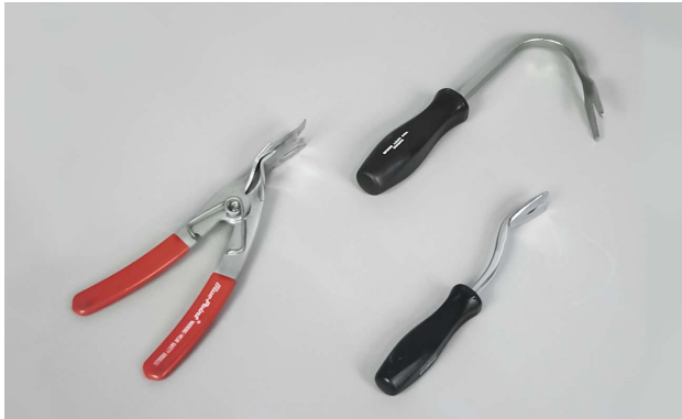
These tools can be used to remove a door interior trim panel.
