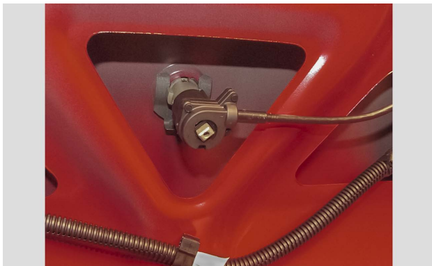
A steel retainer clip holds this lock cylinder in position.
