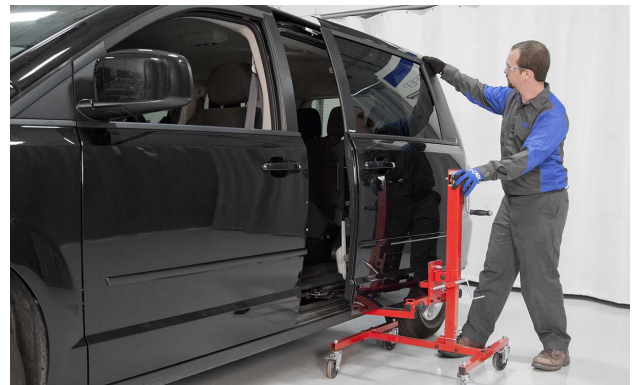
This sliding door is removed by removing the stop and rolling the door off of the tracks.
