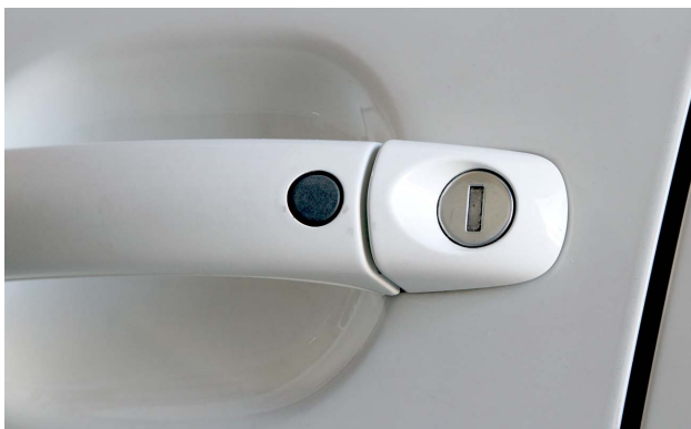
This door lock cylinder is installed in the outer door handle.
