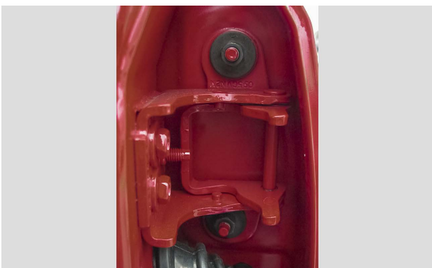
This door hinge is bolted to the pillar.
