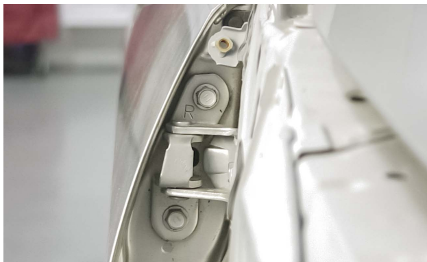
This door-mounted hinge has adjustments for height and flushness.
