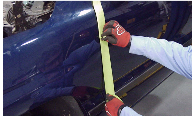
Tape is used on the door panel edge to prevent paint chipping when the fender is removed.
