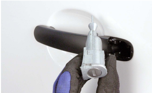
This lock cylinder is removed in preparation for refinishing.
