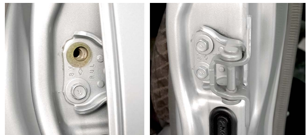
The lack of finish on this door hinge (left) can help during alignment.
