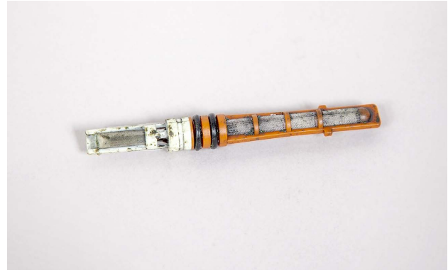
One troubleshooting method is a visual examination of system parts, such as with this orifice tube.
