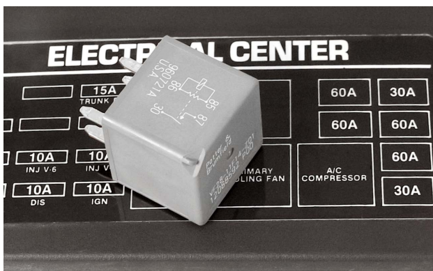
The compressor clutch uses a large amount of current and requires a relay to operate.
