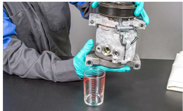
Use a clean container to collect and measure the amount of oil in a compressor.
