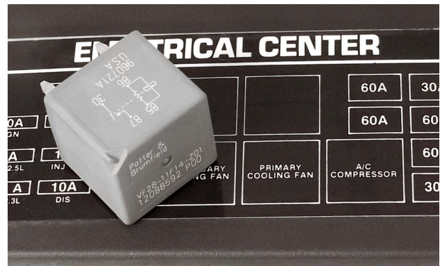
One fan relay may control the primary fan while another fan relay controls the secondary fan.
