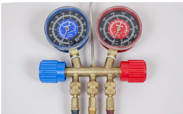
Manifold gauges read system pressures in pounds per square inch (psi) and / or kilopascals (kPa).
