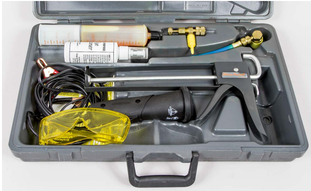
Leak detectors may use UV dye and a black light.
