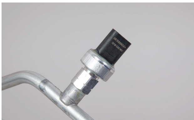
This switch is an environmentally safe way of controlling excessively high system pressures.
