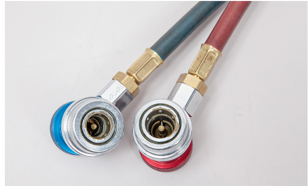
The blue hose is for the low side. The red hose is for the high side.
