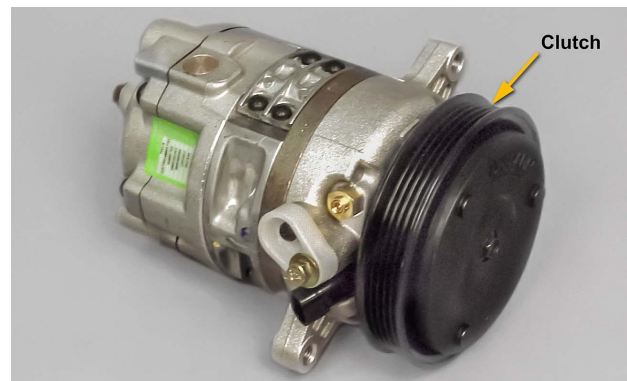
This variable displacement compressor continuously cycles the clutch and regulates pressure internally.
