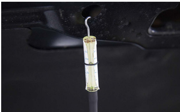
The flow meter will indicate little or no refrigerant flow if sealant is present in the system.
