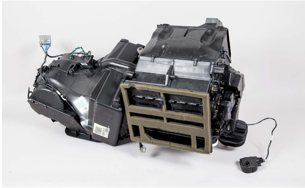
The air distribution center is located in the engine compartment and under the instrument panel.
