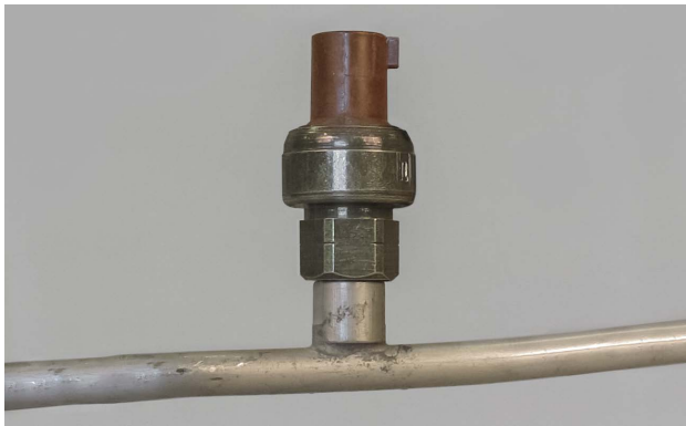
This high / low-pressure cutoff switch protects the compressor from excessive high and low pressures.
