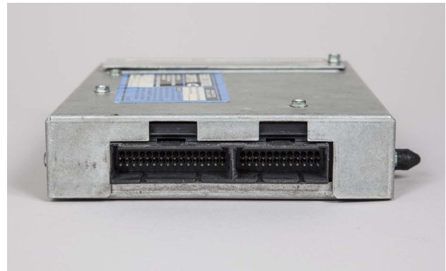
Powertrain control modules may look similar to other types of control modules including ABS and traction control.
