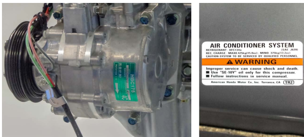
Electric A/C compressors have specific refrigerant oil requirements.
