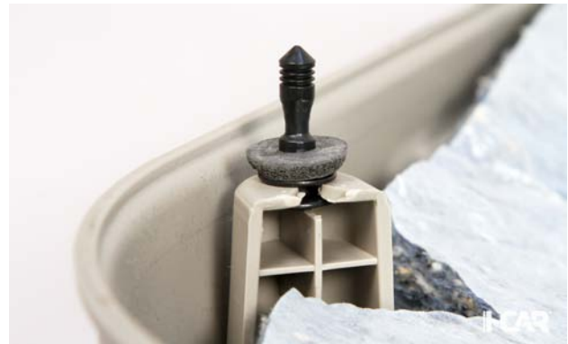
This type of clip can break easily during part removal.
