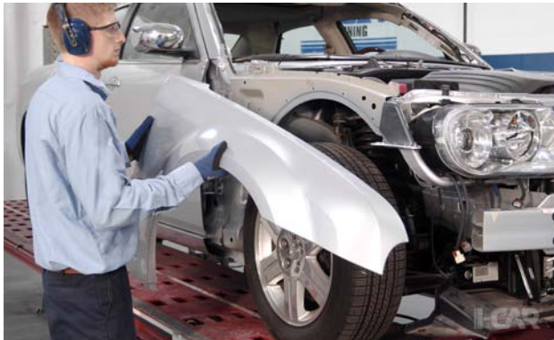
A frame rack should not be used to hang exterior body panels after structural repairs are complete.
