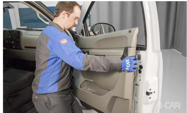
Repairing a door requires removal of the interior trim.
