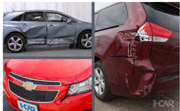
Damage can be ranked by severity, clockwise from the top: one (heavy), two (medium), and three (light).
