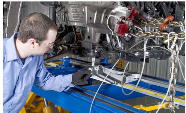
Measuring is part of the straightening process and done before complete disassembly.
