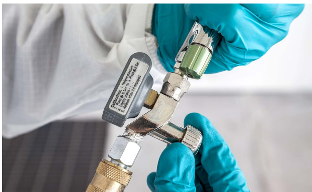
This shows the adjustment for spray gun air pressure.
