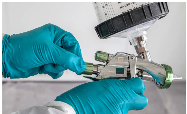
This shows the adjustment location for the fluid needle.
