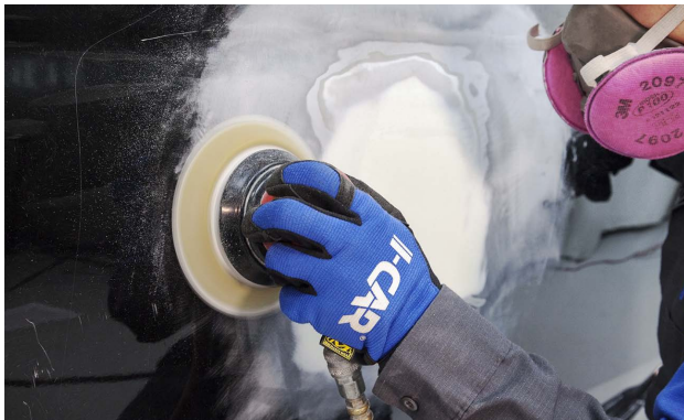
Featheredging out the OEM finish helps eliminate a noticeable repair area.
