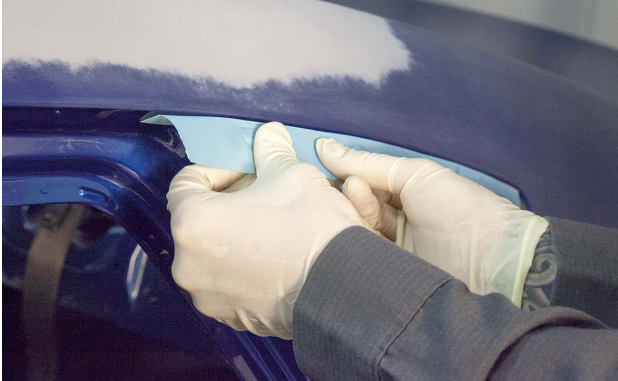
Lifting tape is being applied to quarter glass molding.
