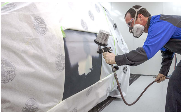
This epoxy primer is being applied over body filler.
