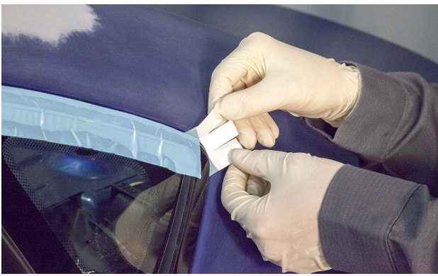
Relief cuts in the lifting tape are used to help mask the corner of the quarter glass.
