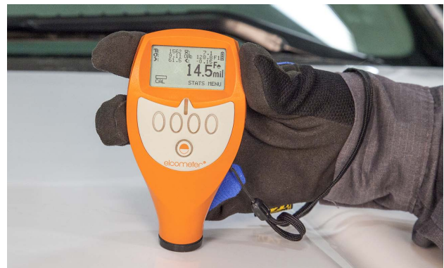
A thickness of 14.5 mils means that some of the finish must be removed before refinishing.
