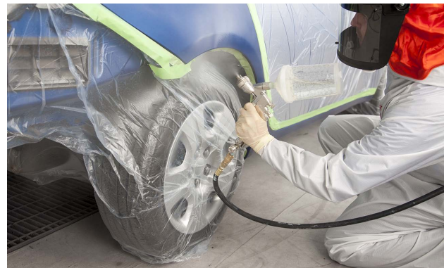
Spraying the wheelhouse requires good technique to avoid paint defects.
