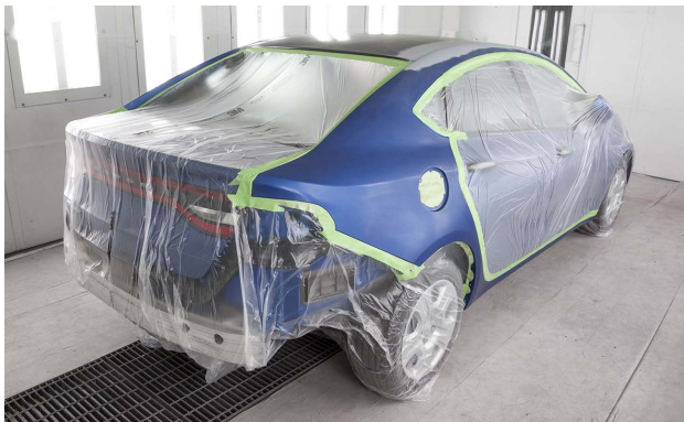
Proper masking ensures overspray does not damage the finish or parts away from the repair area.
