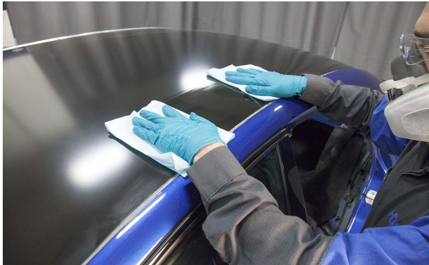
Wiping an E-coated panel with solvent helps prepare it for basecoats.
