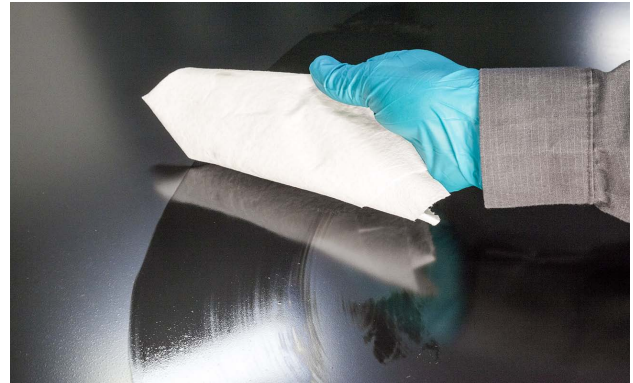
No coating transfer to the cloth generally means the part has E-coat applied.
