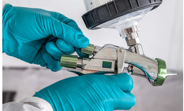
This shows the location for the spray gun fan adjustment.
