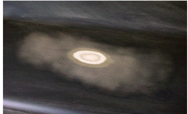
Featheredging is a standard repair technique used to smooth out the repair area.
