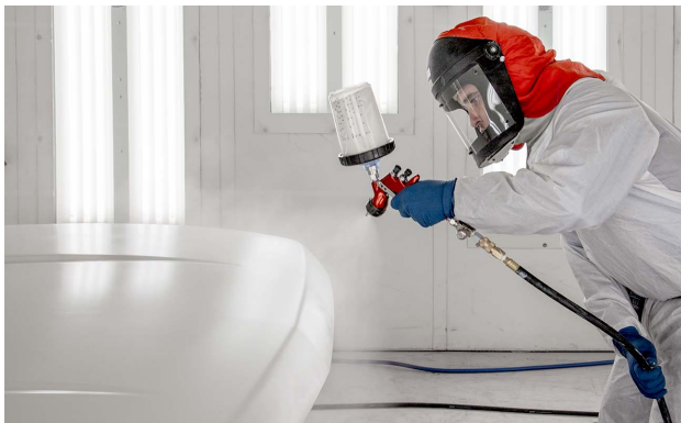
Wearing the proper personal protection equipment prevents hazardous materials from entering the body.
