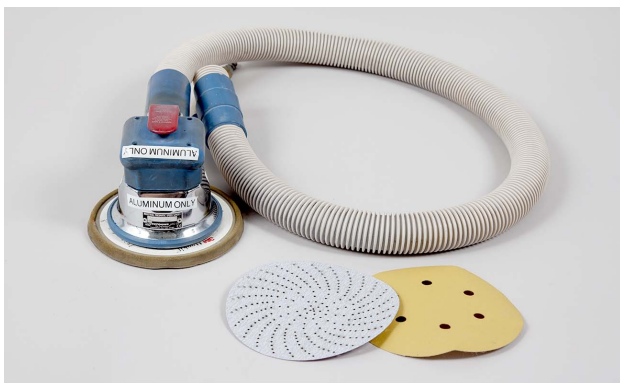
Dedicated tools for aluminum only should be used when working on aluminum panels.
