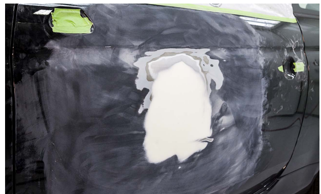
Scuffing the surface of a finish adjacent to the repair area will allow good topcoat adhesion.
