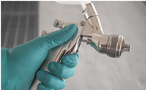
Proper trigger technique can help create better transfer efficiency.
