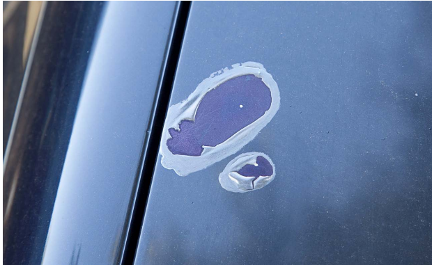
This shows a clearcoat with adhesion problems.
