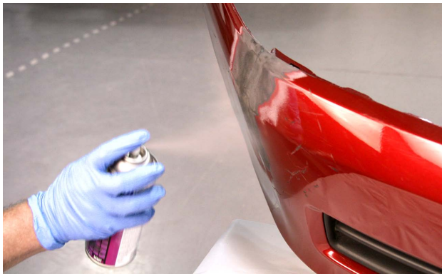
This adhesion promoter is being applied to bare plastic before priming.
