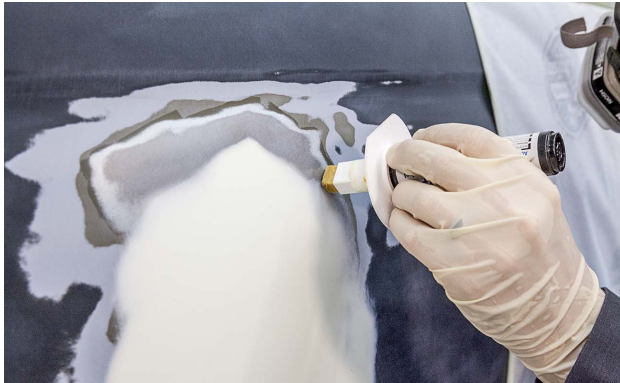
This application stick allows self-etching primer to be applied to bare metal only.
