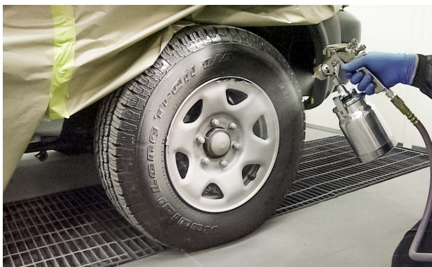
Spray masking can also be applied to tires.
