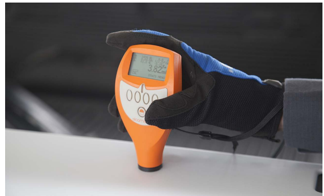
A film thickness reading of 3.82 mils should allow additional coatings to be applied without any problems.
