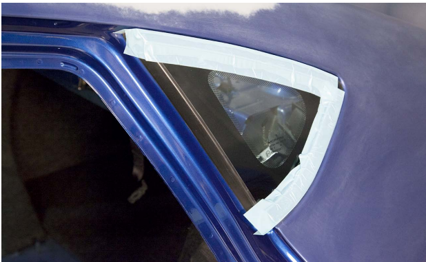
Lifting tape is applied around the entire quarter glass to pull the molding away from the refinish area.
