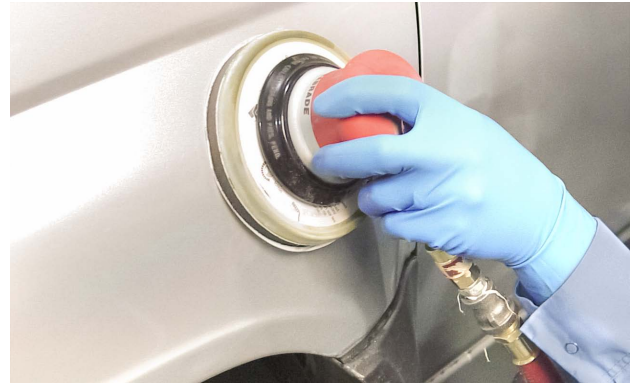
It may be necessary to remove refinish coatings if they are too thick.
