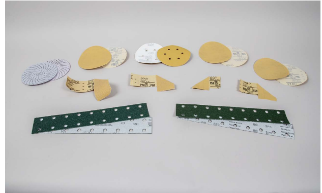
A variety of grits are used to reduce the thickness of a finish.
