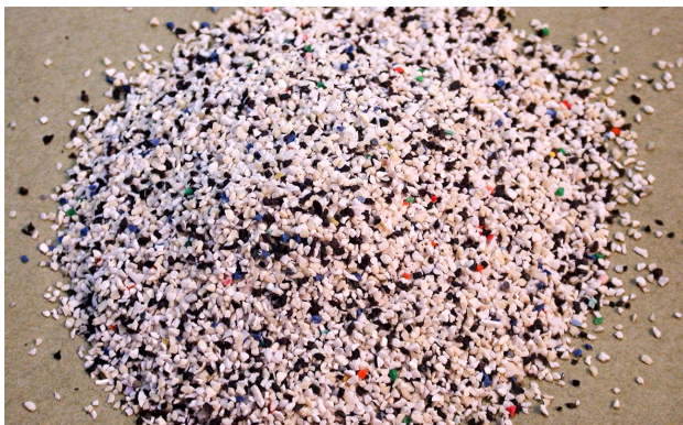
Plastic, such as this, can also be used for media blasting.
