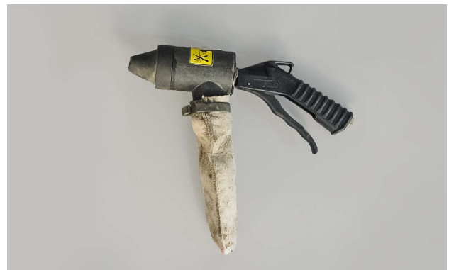
Portable media blasters can be used to remove a finish.
