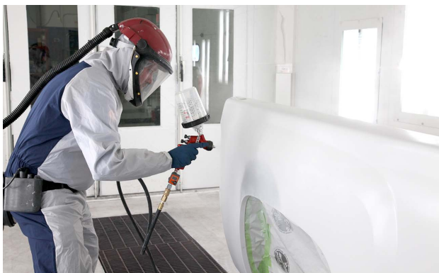
Improper travel speed can cause drips or poor coverage.
