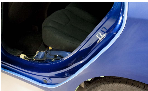
Aperture tape is applied around the entire door opening, along the dog leg area and outer rocker panel.
