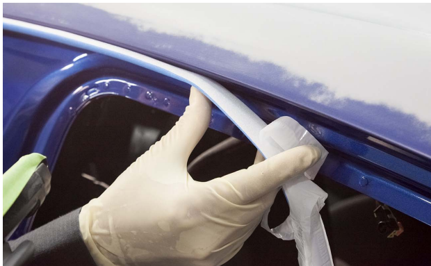
Aperture tape is being applied to the door opening.
