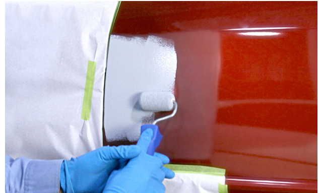
Axalta offers a primer-surfacer which can be applied with a roller.
