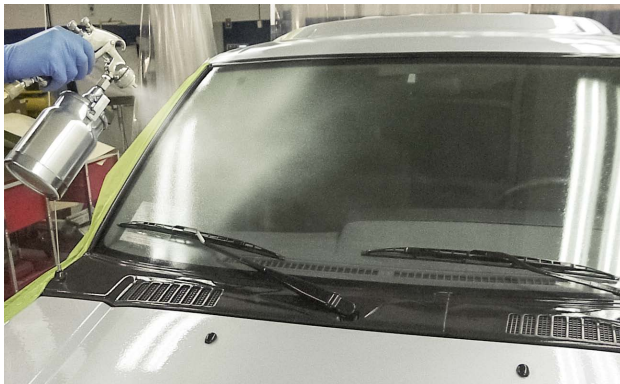
Spray Masking is sprayed away from the area being refinished, such as the windshield on this vehicle.
