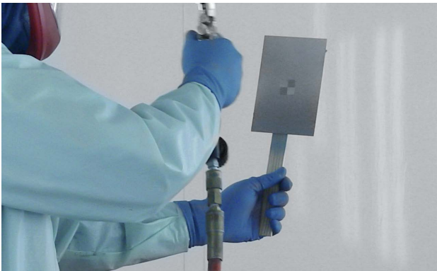
Sprayout panels are used to determine color match.
