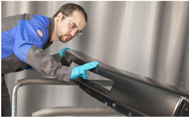
Inspecting the E-coated part upon delivery can help identify potential refinish problems.
