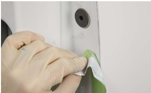
Improper masking led to improper refinish coverage.
