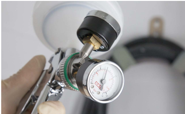
This is an example of an air pressure gauge on a spray gun.
