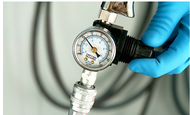
Setting the proper air pressure ensures the refinish material is applied most efficiently.
