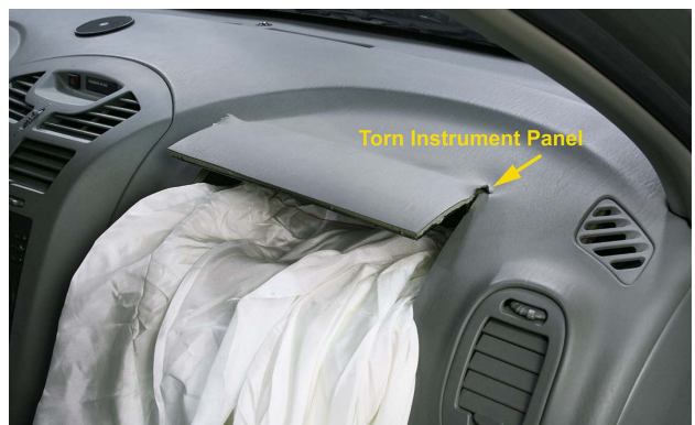
This instrument panel was torn during the passenger airbag deployment.
