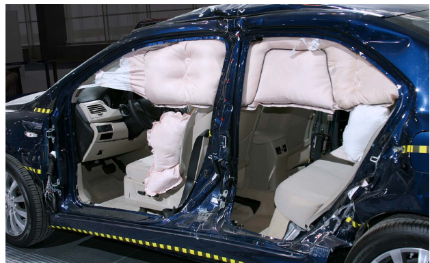
This Suzuki Kazashi display shows side airbags frozen in their deployment state.
