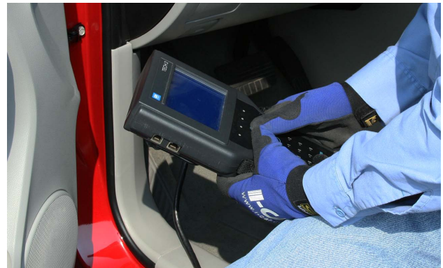
Reprogramming the restraints control module typically requires a vehicle maker scan tool.
