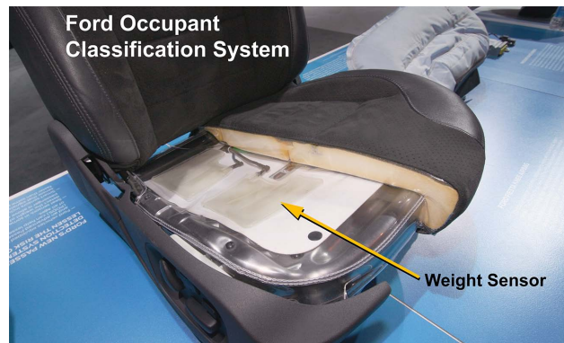
This cutaway passenger seat from a 2011 Ford Taurus reveals the bladder sensor that is part of the occupant classification system.
