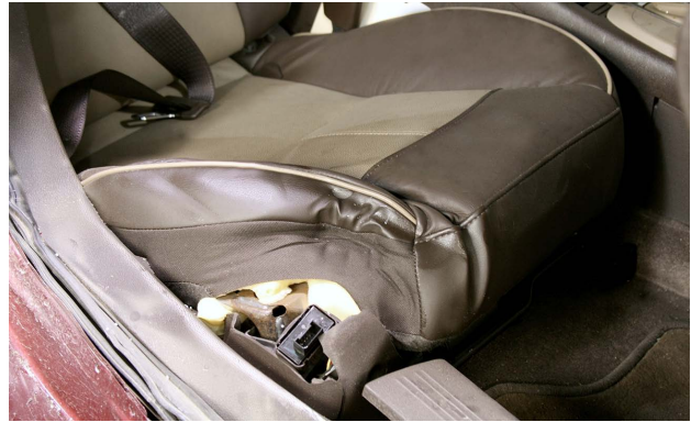
Side impact damage caused damage to the bottom of this seat, perhaps even damage to the seat frame.
