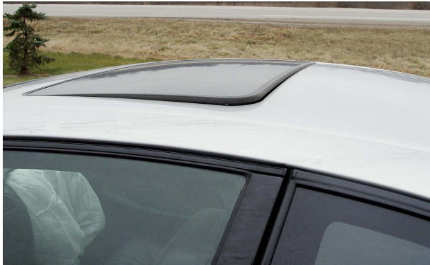
This sunroof is dislodged due to the pressure of airbags deploying in the passenger compartment.
