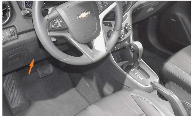
The knee bolster is mounted under the instrument panel and may provide extra protection to the knees.
