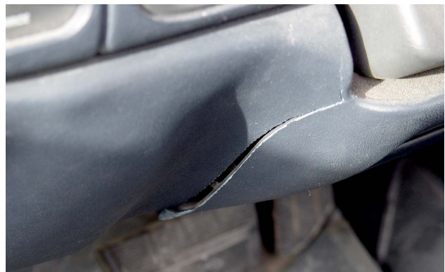
A damaged knee bolster, such as a crack like this, requires replacement.
