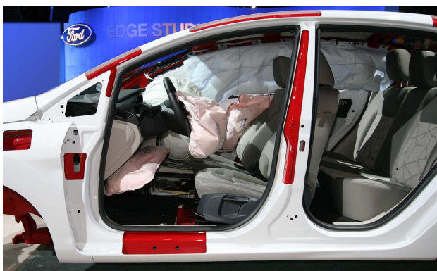
This 2011 Ford Fiesta cutaway shows several airbags frozen in their deployed state.
