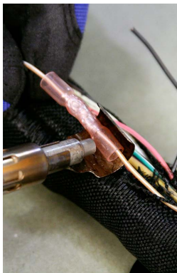
SRS wiring repairs may require wire splice sleeves (left) and a special repair kit (right).
