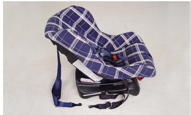
Removable child safety seats must be closely inspected for damage. Some may require replacement after a collision even if not damaged.
