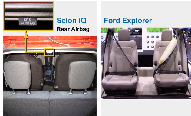
Two novel types of airbags include the rear window curtain airbag on the 2011 Scion iQ and the Ford rear inflatable seat belt.
