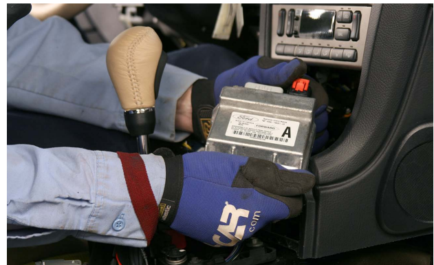
It is a common recommendation for the RCM to be replaced after a deployment or a certain number of deployments.
