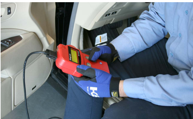
The technician may have to use a scan tool to reveal electronic problems with the restraint system.
