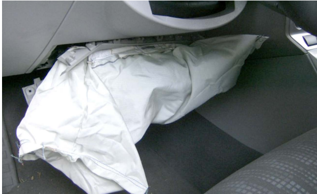
Knee airbags are used on more vehicles today than ever before.
