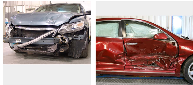
A front impact (left) will deploy different restraints than a side impact (right).
