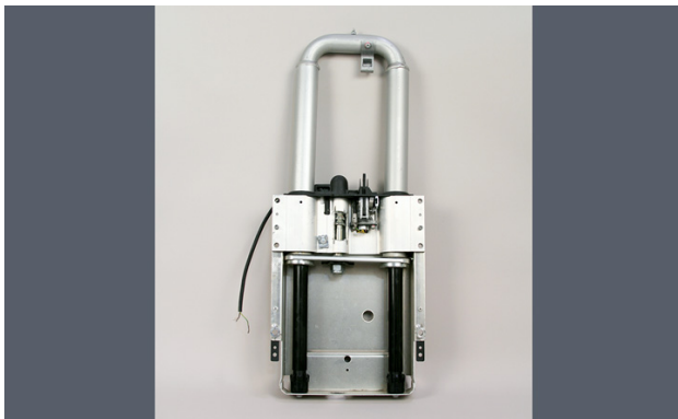
Pop-up roll bars may be serviced as separate cassette assemblies.
