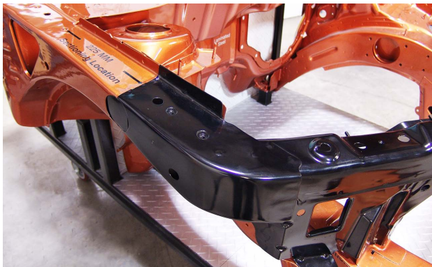
This is the sectioning location for the upper rail on the Chevrolet Cobalt.
