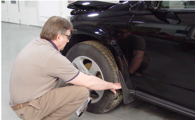
Checking wheel positioning can determine if there is damage to the suspension or vehicle underbody.
