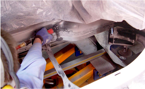
This shows the floor pan being replaced on a Chevrolet Corvette Z06.
