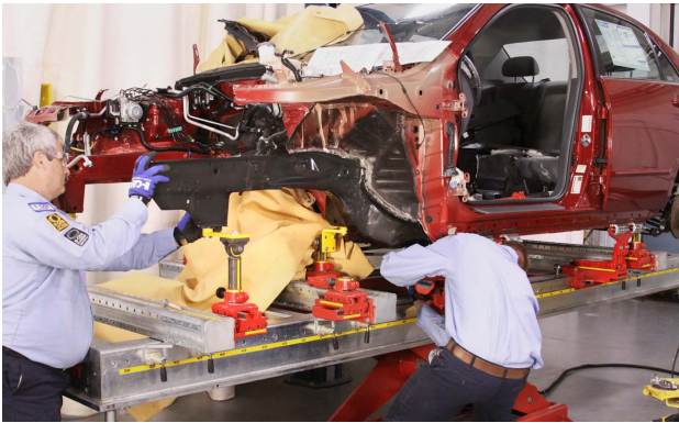
The front rail on this Honda Accord is being completely replaced at factory seams.
