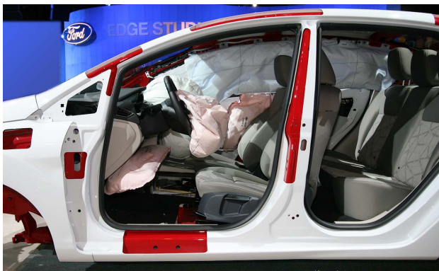
This shows the HSS and UHSS inner structures on the Ford Fiesta.
