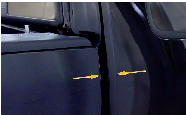
Inconsistent cab-to-bed gaps may be a visual indication of frame damage.
