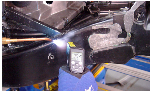
If heat is allowed by the vehicle maker, the amount of heat applied should be monitored to make sure it does not exceed recommendations.
