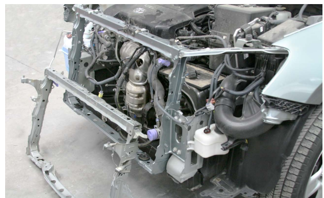
This shows a bolt-on radiator core support with upper and lower tie bars, and side panels.
