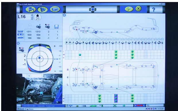
Electronic measuring system equipment provides vehicle specific measurements.
