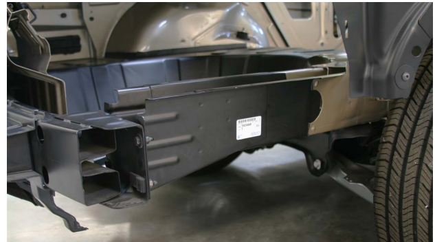
The rear rails on this Chevrolet Malibu allow partial replacement at factory seams.
