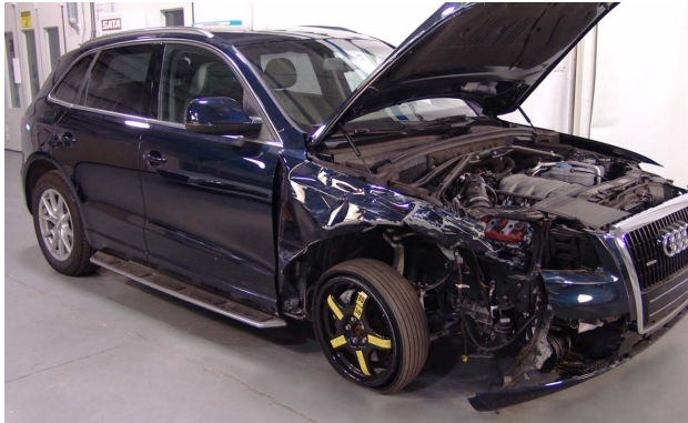
Direct damage to this vehicle occurred at the passenger-side front rail.
