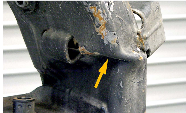
This portion of a frame rail is kinked.
