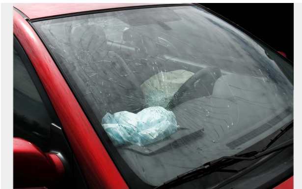
This glass was damaged from the airbag deflecting off the windshield during deployment.
