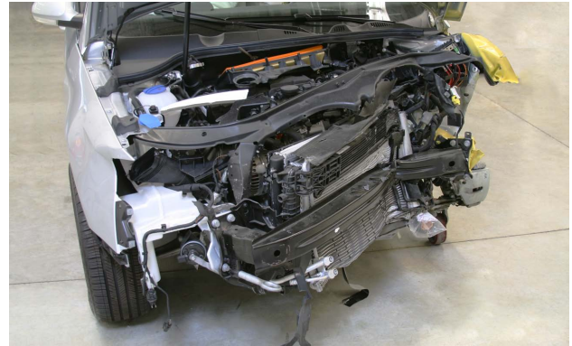
This particular damage shows mash, twist, and possibly diamond.
