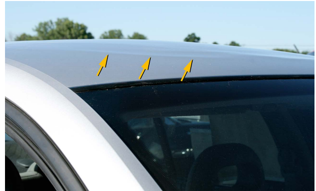
Some roofs can buckle from structural damage since the unitized structure can twist and distort body panels.
