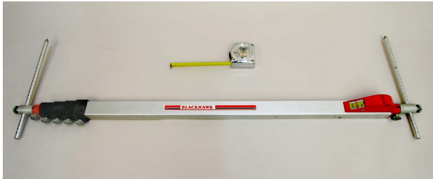
Tape measures and tram gauges are used to make point-to-point measurements.
