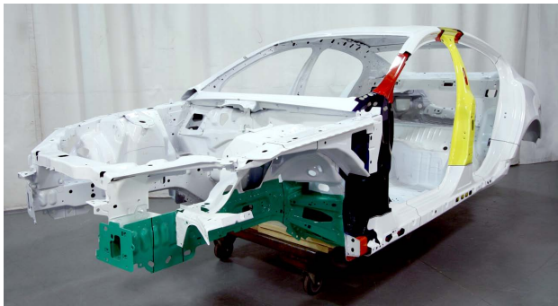
This Jaguar XF unibody shows the inner structure with the outer panels and trim removed.
