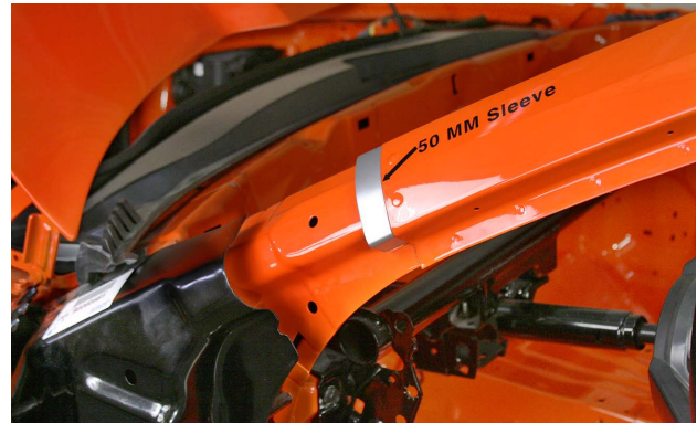
The Chevrolet Camaro has a sectioning procedure for the A-pillar.
