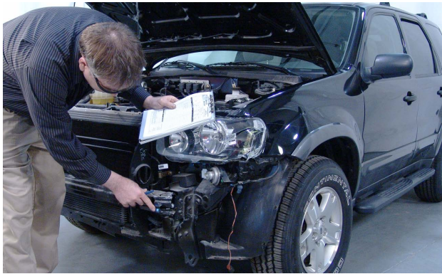
A thorough damage analysis may require some part removal to accurately assess damage.
