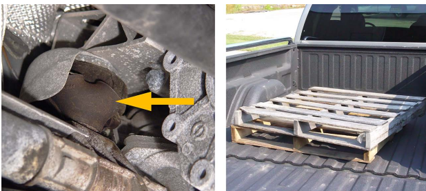
Motor mounts can be damaged from the engine moving forward or rearward during impact (left). Items in a pickup truck bed can cause damage to the front of the box or the tailgate (right).
