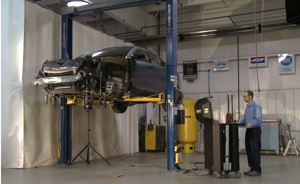
Three-dimensional measuring systems, such as this one, can be used to measure without anchoring to a bench.
